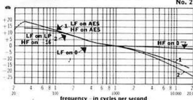
A440A preamplifier—range at base and treble tone controls
