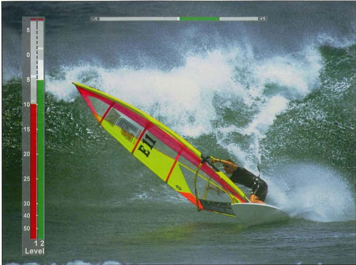
The Chromatec AM-2 is an in-picture and dedicated on-screen audio level meter for displaying two channels of analog or digital audio, in bargraph form.
