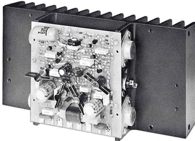
One of the two assembled and tested power output modules as supplied in the kit.
