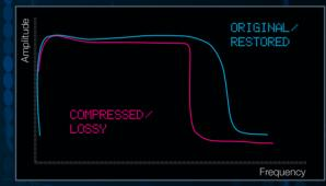
Adds high-frequency bandwidth extension for more clarity and detail.
