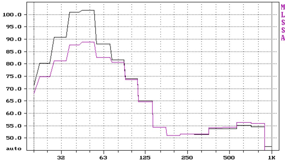
Figure 5. We think we can improve the shape a bit, so we dial in some attenuation at the two highest peaks, using a 1/3-octave graphic equalizer (lower curve).
