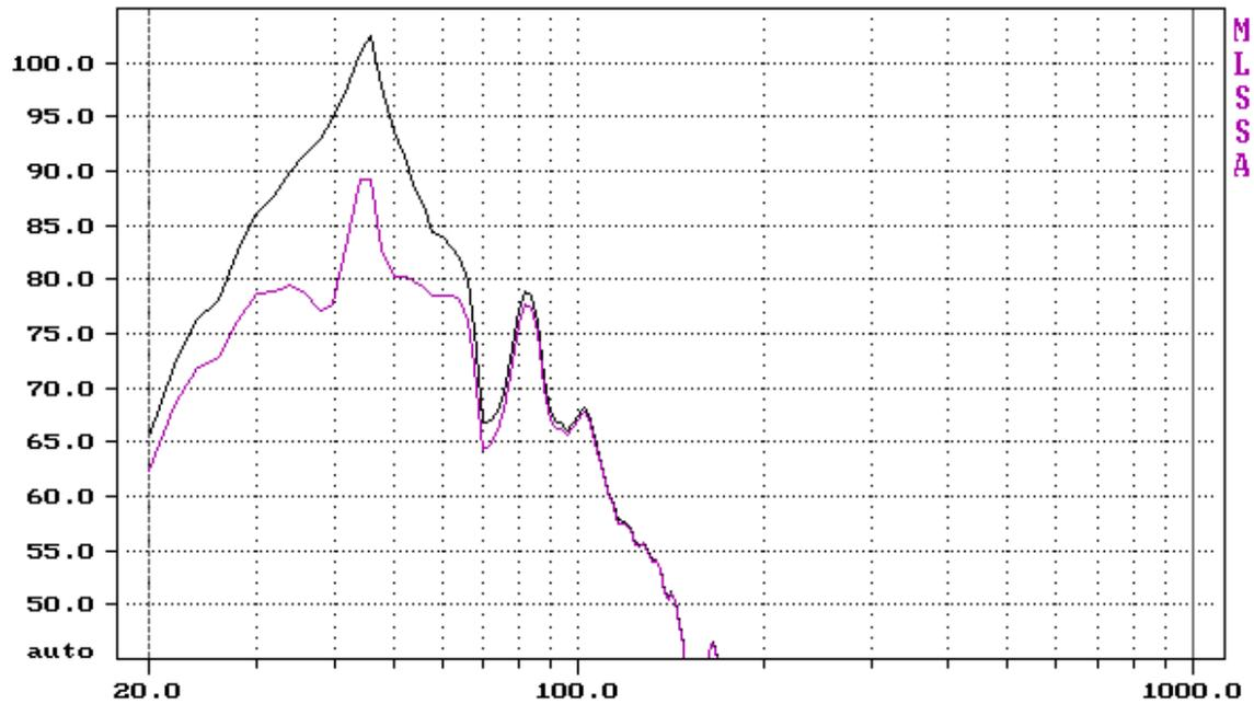
Figure 6. These are the high-resolution frequency response measurements of the subwoofer before (top curve) and after (bottom curve) equalization with the 1/3-octave graphic equalizer.
