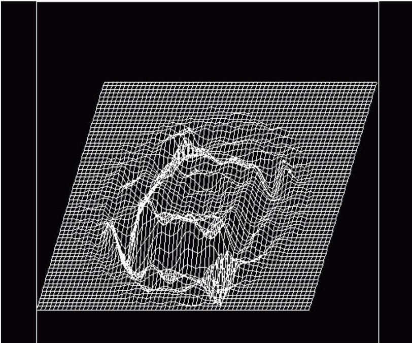
*Figure 9. A scanning laser vibrometer measurement of cone movement for a 6.5-inch fabric-reinforced composite cone, operating at 3.5 kHz.*
