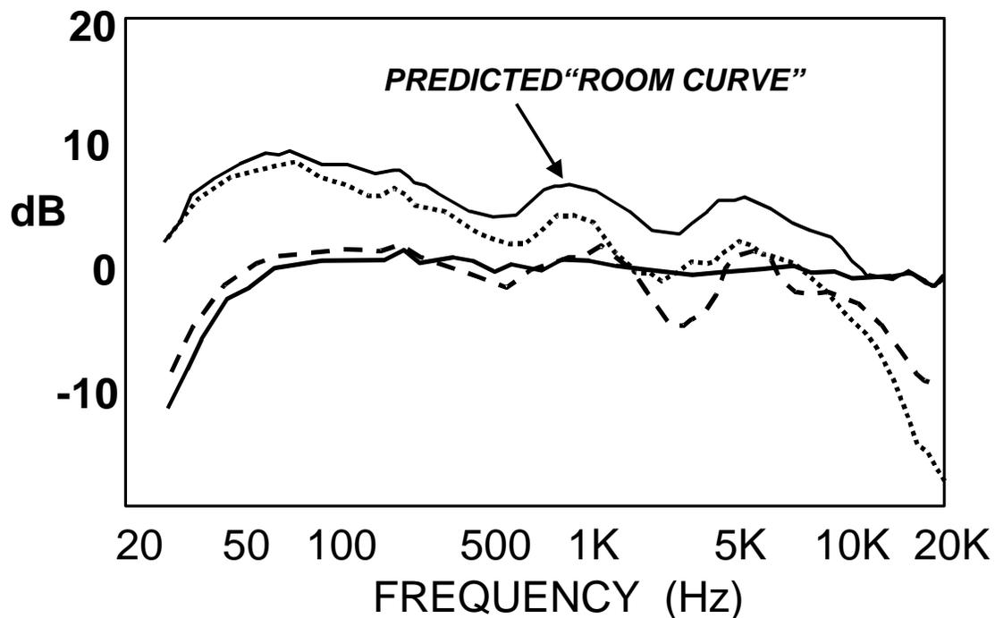
Figure 2. The sequence of sounds arriving at the listening area in a room. The first sound to arrive is the direct sound, represented by the on-axis frequency response (the solid line around 0 dB). The second sounds to arrive are the early reflections from the floor, ceiling and side walls. These are represented by an energy sum of anechoic
