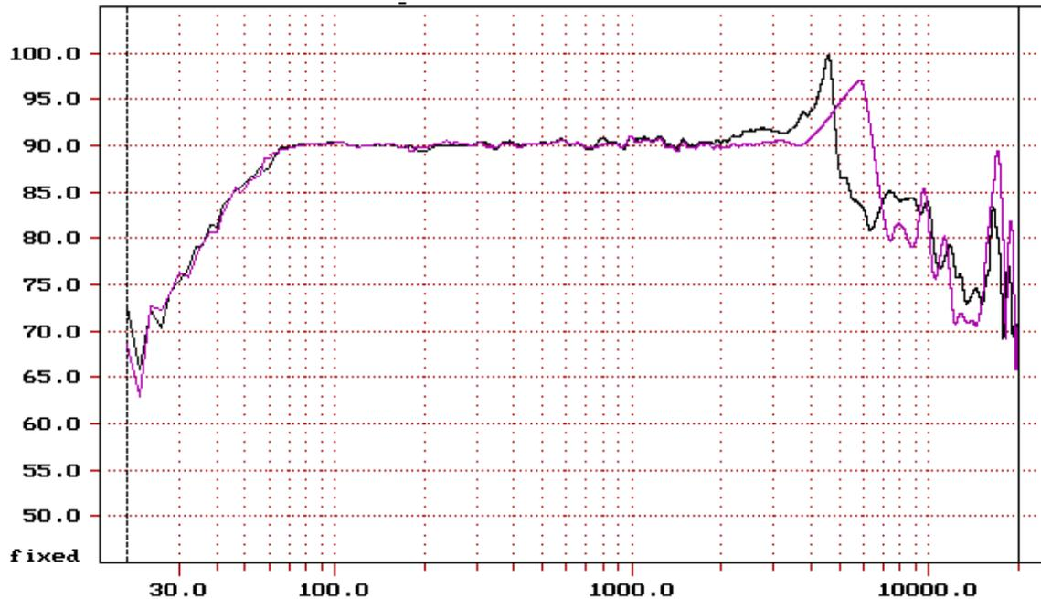
Figure 6. On-axis measurements of a 6.5 inch mid-bass driver with a cone made of aluminum (top curve) and of a ceramic / aluminum laminate (bottom curve).
