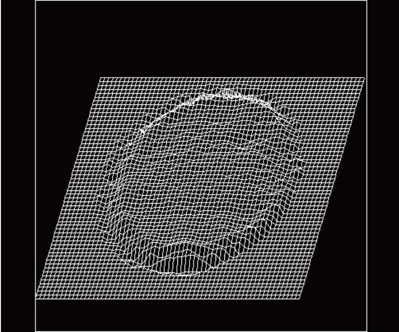
*Figure 8. A scanning laser vibrometer measurement of cone movement for a 6.5-inch ceramic/aluminum laminated cone, operating at 3.5 kHz.*
