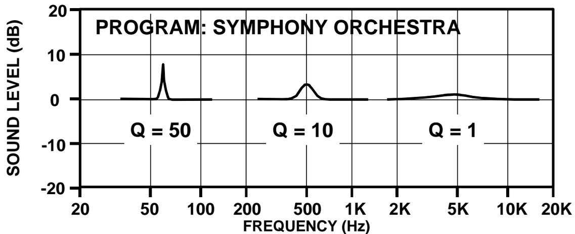
*Figure 5. Frequency response deviations caused by resonances with different  $Q$ 's, when they have been adjusted to the levels at which they are just detectable when using symphonic music as a test signal. NOTE: Ignore the positions the resonances occupy on the frequency scale; they are about equally detectable at all middle and high frequencies. From reference 2.*
