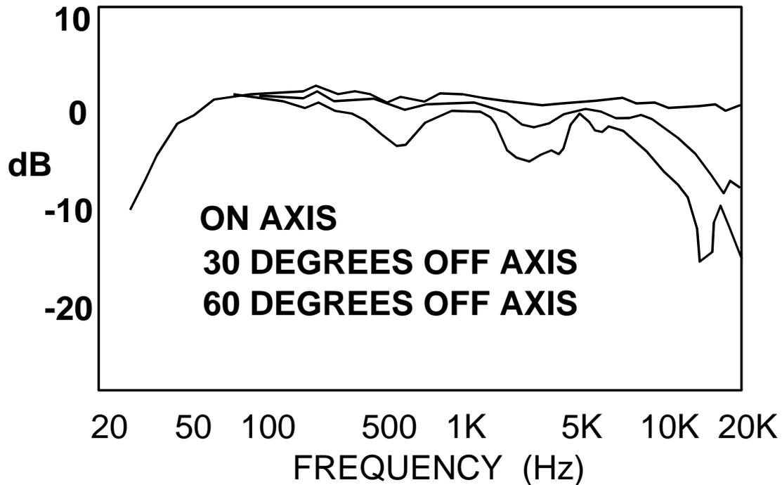
Figure 1. Anechoic frequency response measurements of a loudspeaker showing (top to bottom) a very smooth and flat on-axis response, and increasingly non-flat behavior at increasing angles off axis.
