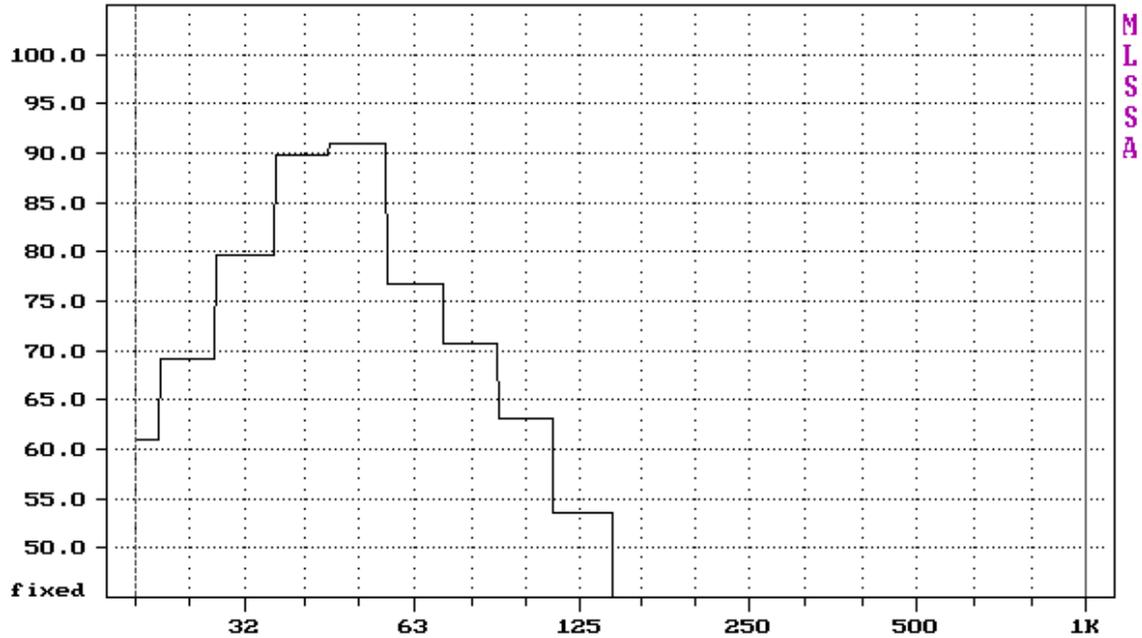
Figure 4. A 1/3-octave version of the unequaled high-resolution frequency response curve in Figure 2. Note the absence of any hint of a high-Q resonance at 47 Hz, and the lack of any evidence of an interference dip at 73 Hz. It doesn't look all that bad, really.
