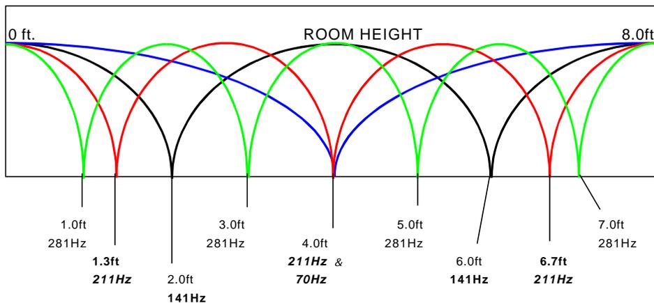
Figure 1 The output of a program that calculates the axial modes of a room, and plots the pressure as a function of distance along each of the principal axes.
