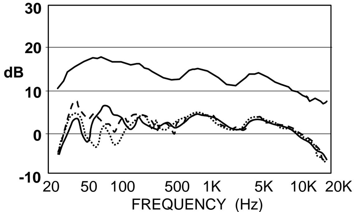
*Figure 3. Measurements of the example loudspeaker in a room. The loudspeaker was placed in three realistic left/right channel locations and, for each one, measurements were made at four possible listening locations, all within a two-foot radius. Each of the bottom curves is an energy average of the four measurements. The top curve is the predicted room curve from Figure 2, which, for clarity, has been shifted vertically by 10 dB.*
