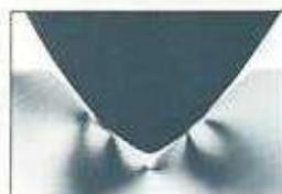
The effect of tracking force (2 grams) on a disc using a SHIBATA stylus.
