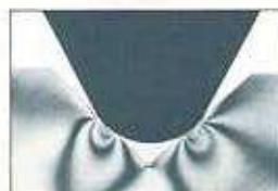
The effect of tracking force (2 grams) on a disc using a conventional elliptical stylus.
