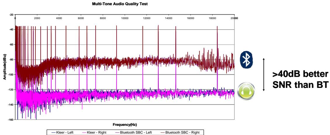
**Figure 1. Multi-Tone Test: Kleer versus BT**
