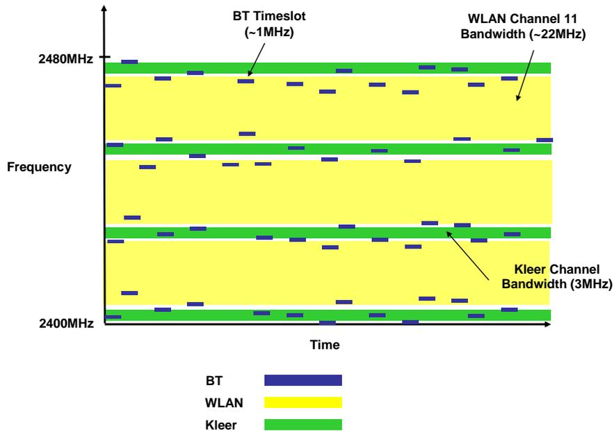
**Figure 2. Minimum Bandwidth Requirements**
