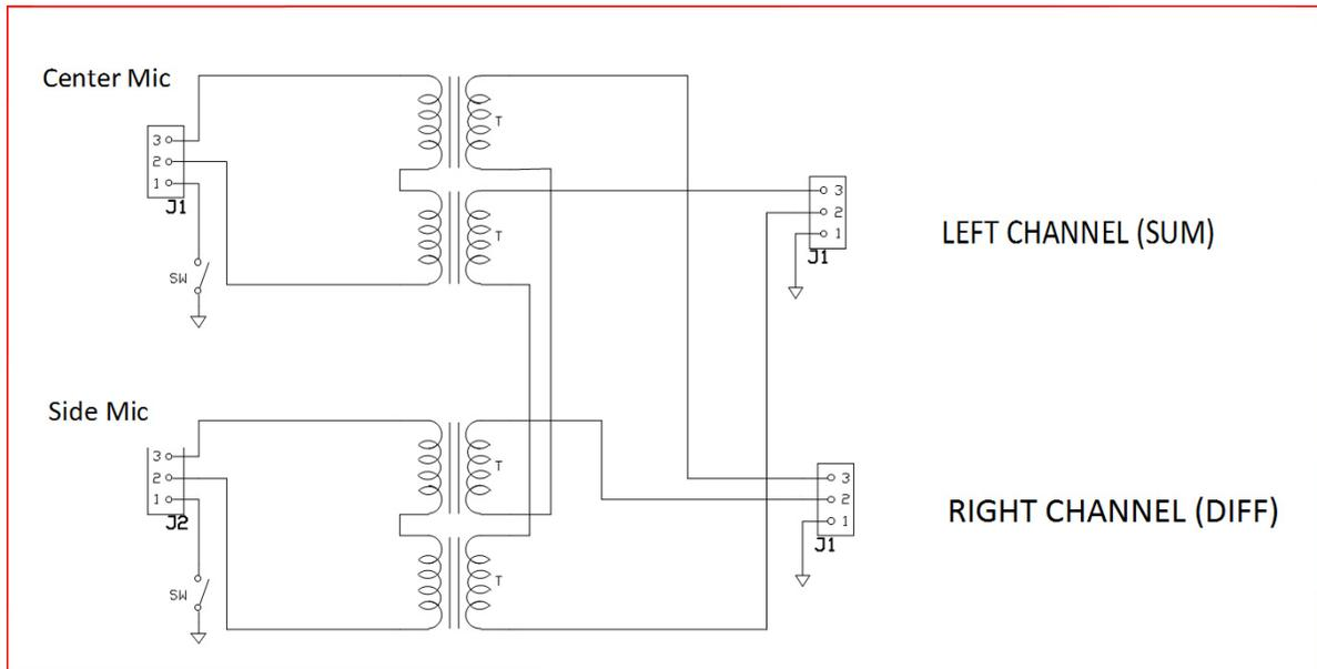
Figure 4: This schematic shows how the dual secondaries are wired to provide the sum and the difference of the two M-S microphones.
