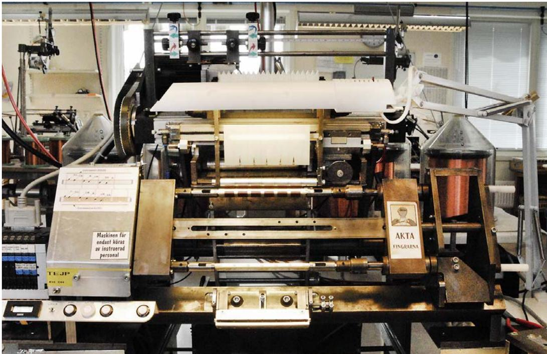
Figure 4: Front view of a Lundahl coil-winding machine.
