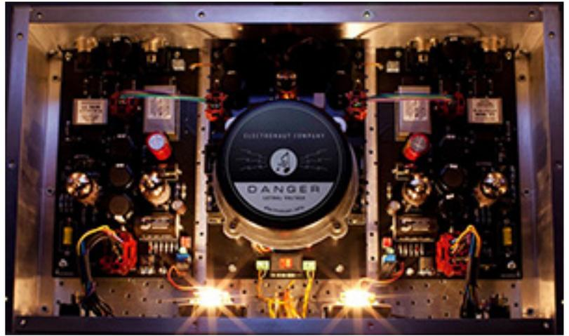
*Lundahl transformers inside an Electronaut mic/instrument preamp.*
