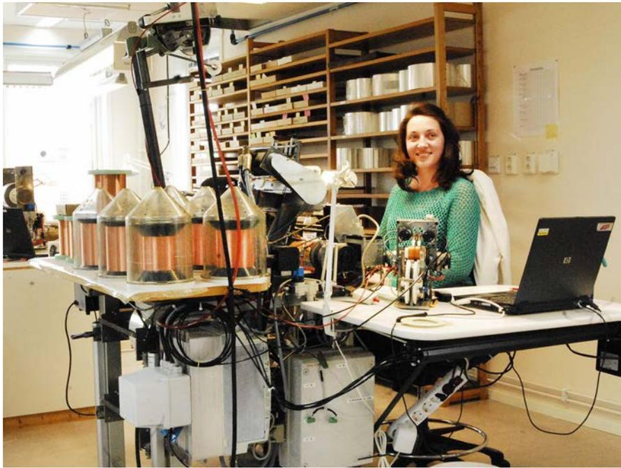
*Figure 10: Lundahl coil-winding machine in use.*
