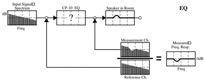
Notice that the analyzer can display an *inverse transfer function*, causing the equalizer's response dip to appear as a peak (1/EQ). This greatly facilitates the system correction procedure: all the operator needs to do is to set the system equalizers so that the 1/EQ display duplicates the major characteristics of the room+speaker display. A precise *complement* of the loudspeaker/room characteristic is thereby generated.
