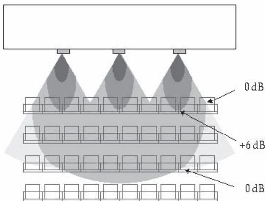
**Fig 3.7e Split-parallel arrays recommended for frontfill applications.**
