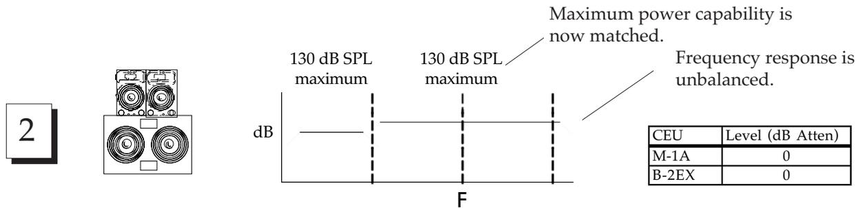
A second UPA-1C is added to the system, which increases the power capability in the MF and HF range. This creates an even maximum power capability over the full range. The coupling that produces the additional power capability also causes the frequency response to rise in the MF and HF range. This unbalancing of the frequency response will need to be remedied or the system will sound thin.
