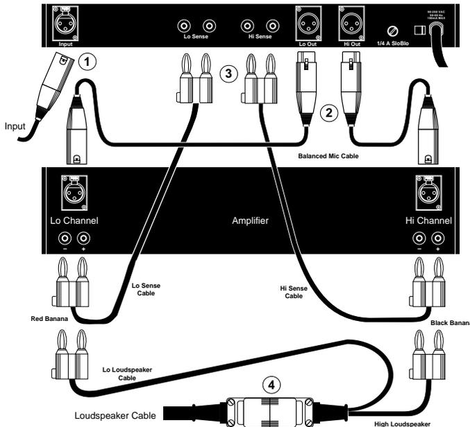
Fig. 1.3i Basic connections.
