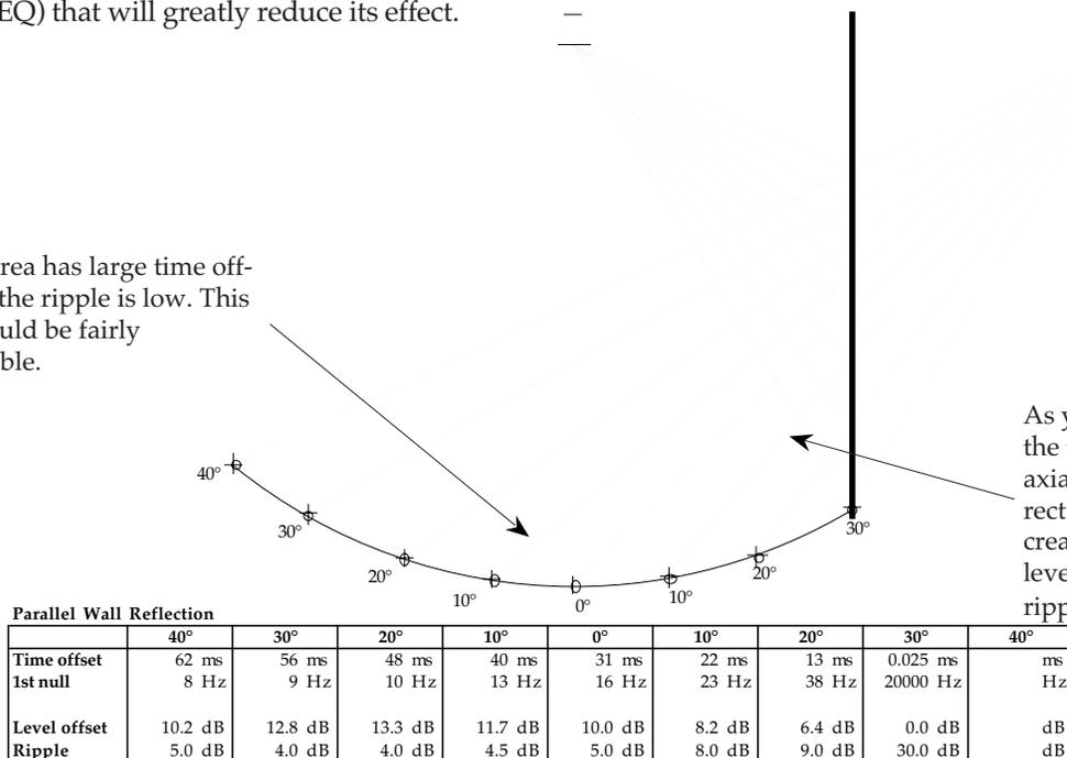
Fig 2.3c Parallel wall reflection.
