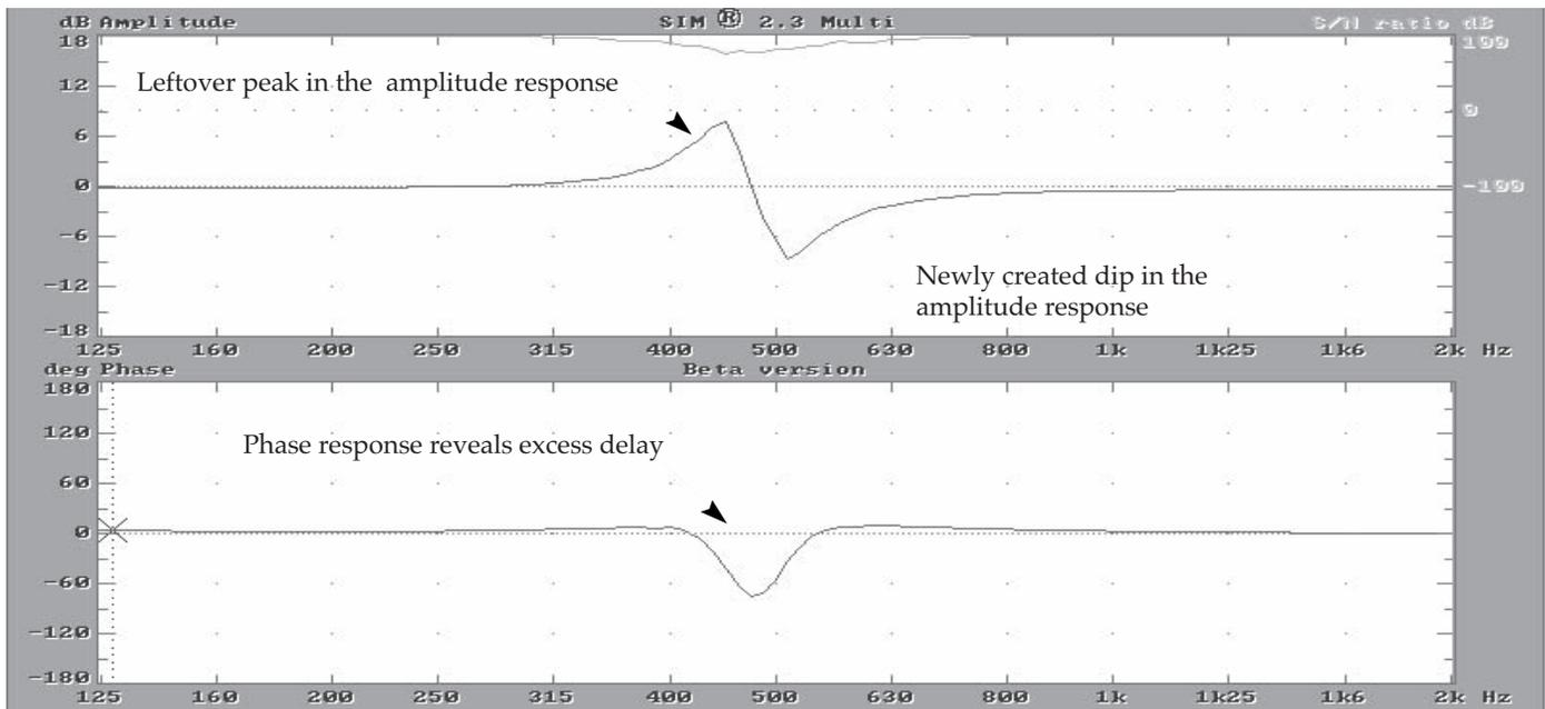
Fig 1.6i Result of error in center frequency.
