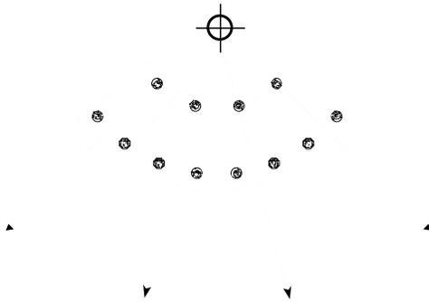
Fig 3.6a Horizontal point-source array with the focal point behind the speakers.
