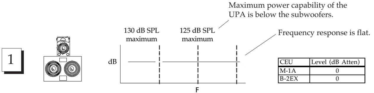
A single UPA is placed on top of a 650-R2 subwoofer. CEU levels and amplifier voltage gains are matched, creating a combined flat frequency response. If the system is run to full power over a broad spectrum, the UPA will compress first since its maximum power capability is less than that of the 650.
