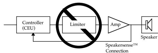
**Fig 1.3a Additional limiters are not required for system protection and may actually compromise reliability as well as dynamic range.**
