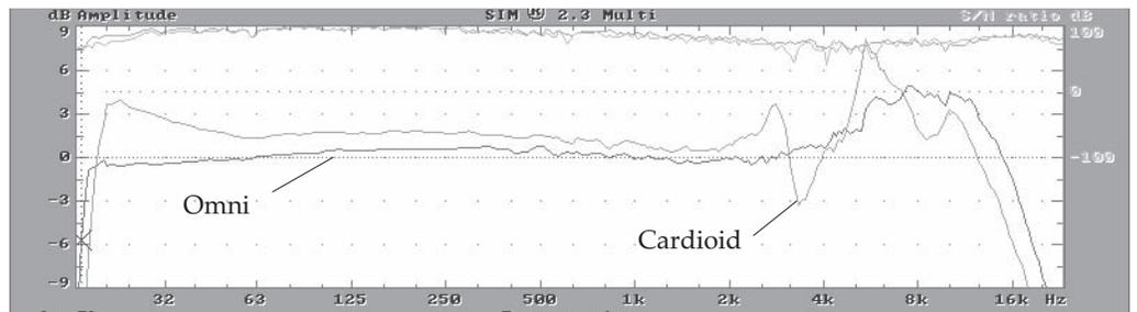
Fig 4.3e Frequency response changes with pattern switch setting.
