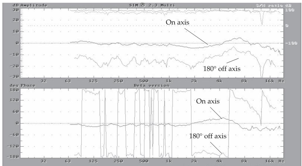
Fig 4.3f Microphone pattern verification.
