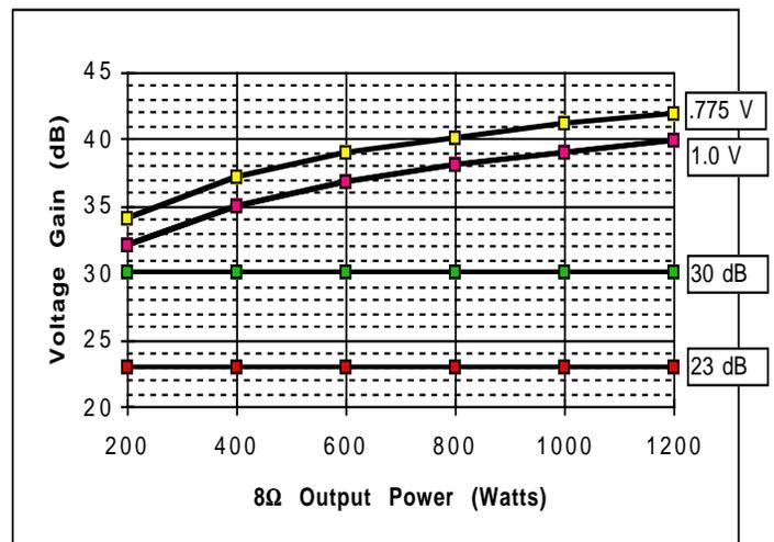
Fig. 1.4c Amplifier sensitivity versus dB gain.
