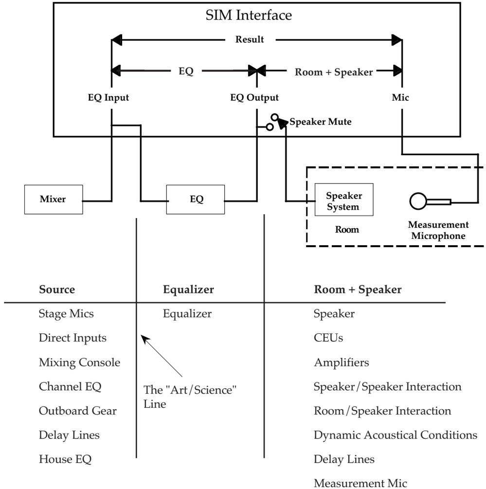
Fig 5.2a SIM interface patched into a sound system.
