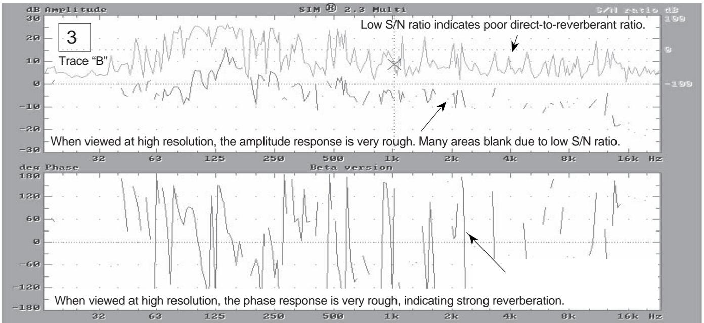
Fig 1.9l (3) High-resolution view of amplitude, phase and S/N ratio of speaker "B" alone.
