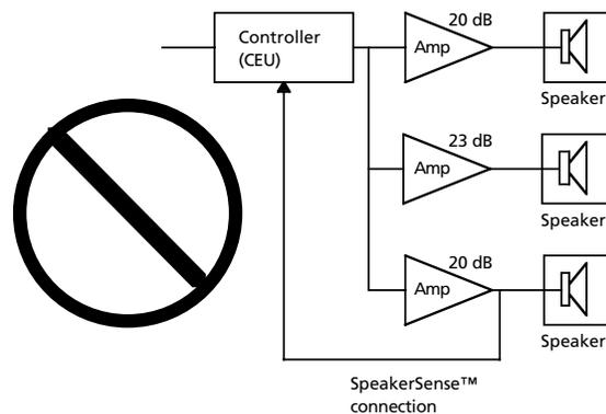
Fig. 1.3n Improper MultiSensing. Sense lines shorted together.
