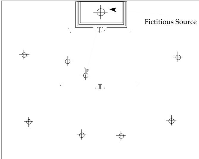
Step 1: Delay the main center system to synchronize to the fictitious source. This helps to create a sonic image in the area of the minister.
