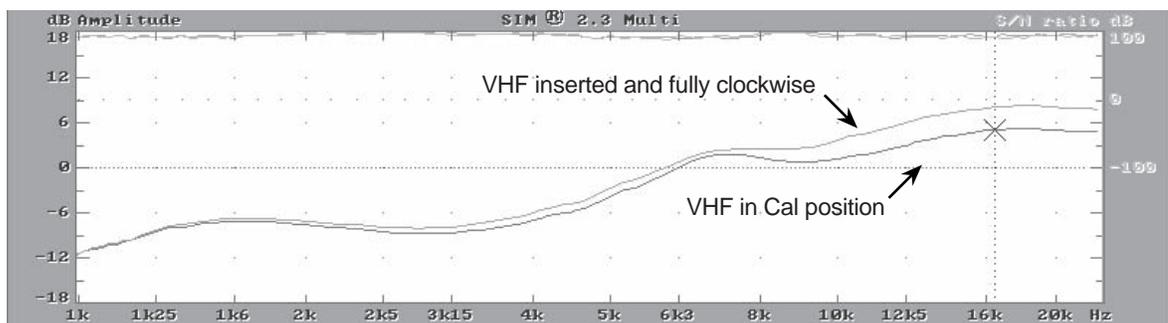
Fig 1.2n The VHF circuit response in the S-1 controller.
