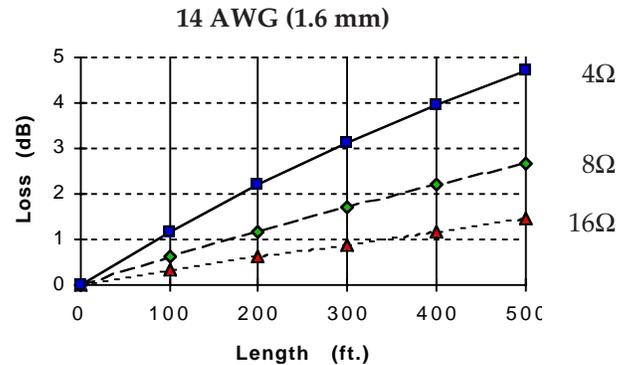
Fig. 1.7.i Cable loss over distance for 14 AWG (1.6 mm).
