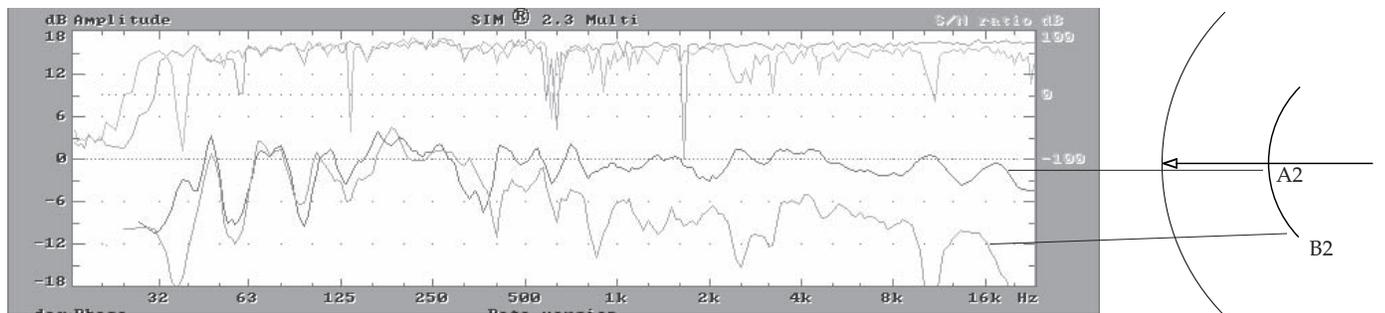
Fig 3.3d Comparison of on-axis near (A2) and off-axis near (B1).
