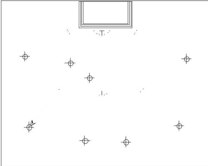
Step 5: Delay the delay sides to the main center system. This was chosen because the main center was the second strongest signal in the delay side area and created a sonic image in the direction of the stage. The interaction with the delay center was negligible.
