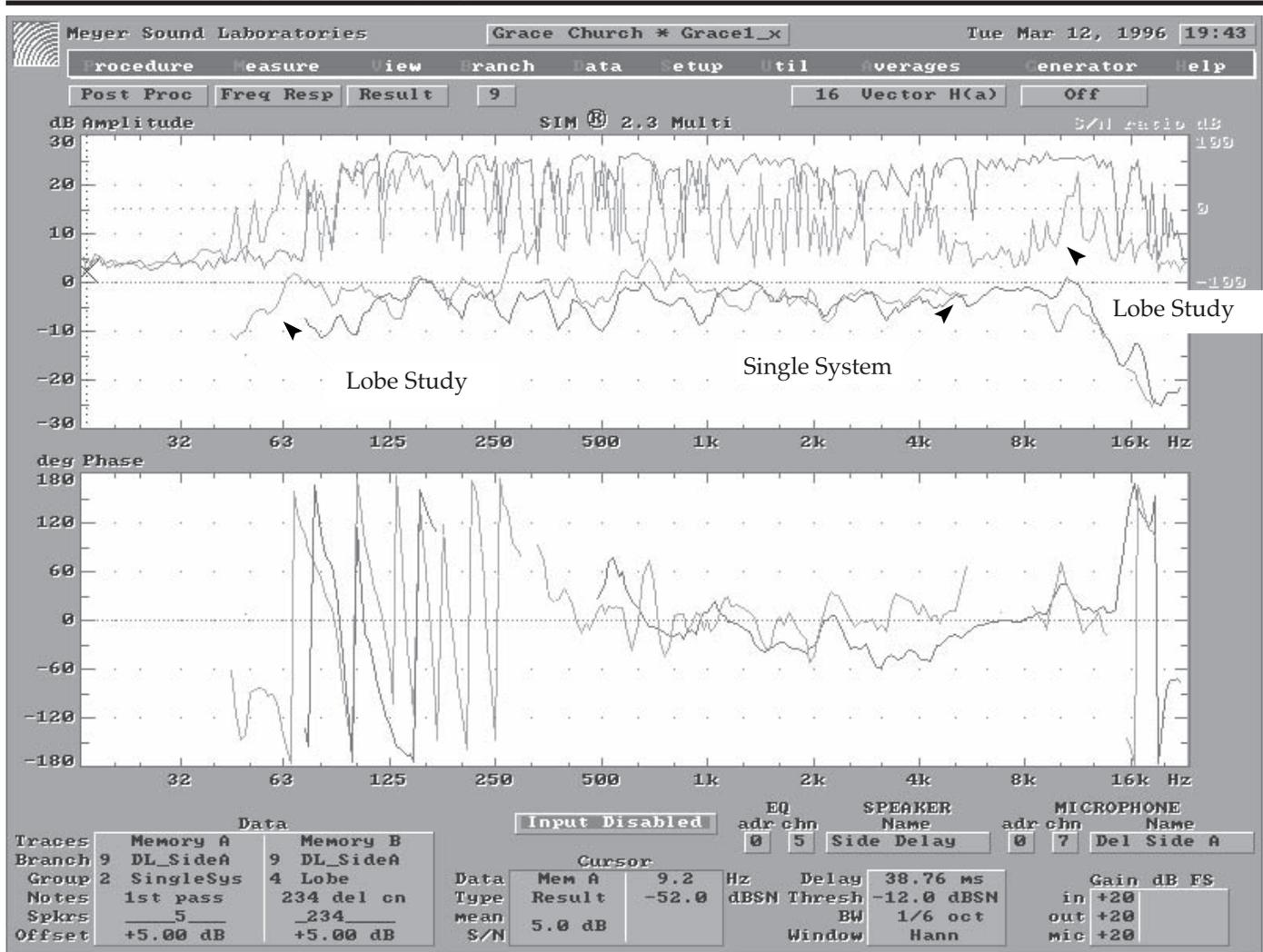
Fig 5.10m Evaluating the need for the delay speakers.
