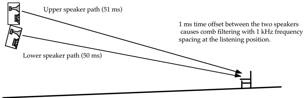
Fig 2.2a Elevation view of speaker interaction between an upper main and downfill system.
