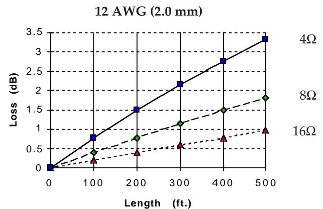
Fig. 1.7.j Cable loss over distance for 12 AWG (2.0 mm).
