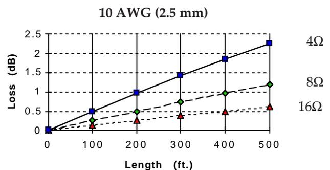
Fig. 1.7.k Cable loss over distance for 10 AWG (2.5 mm).
