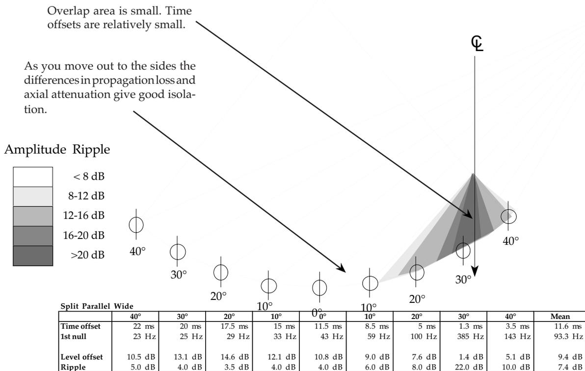
Fig 2.2x Split-parallel (wide) array interaction.
