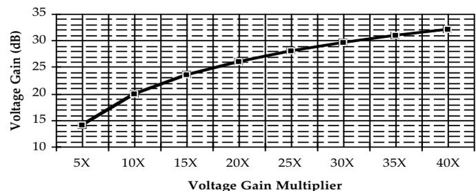
Fig. 1.4b Voltage gain multiplier versus dB gain.
