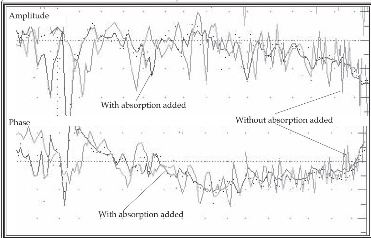
Fig 5.4b Effect of absorptive materials on frequency response.
