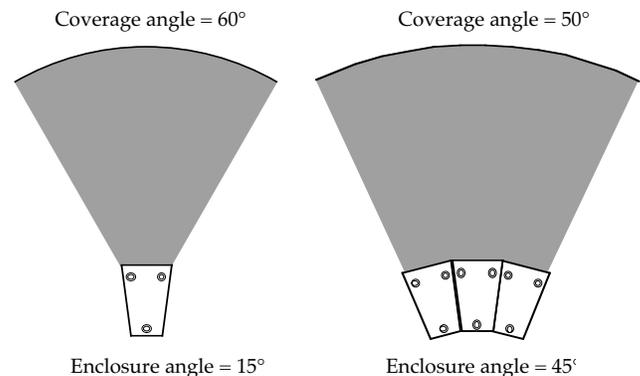
Fig 3.6d MSL-3A coverage pattern narrows while on-axis power increases as additional units are packed together. Use this configuration for long-throw applications.
