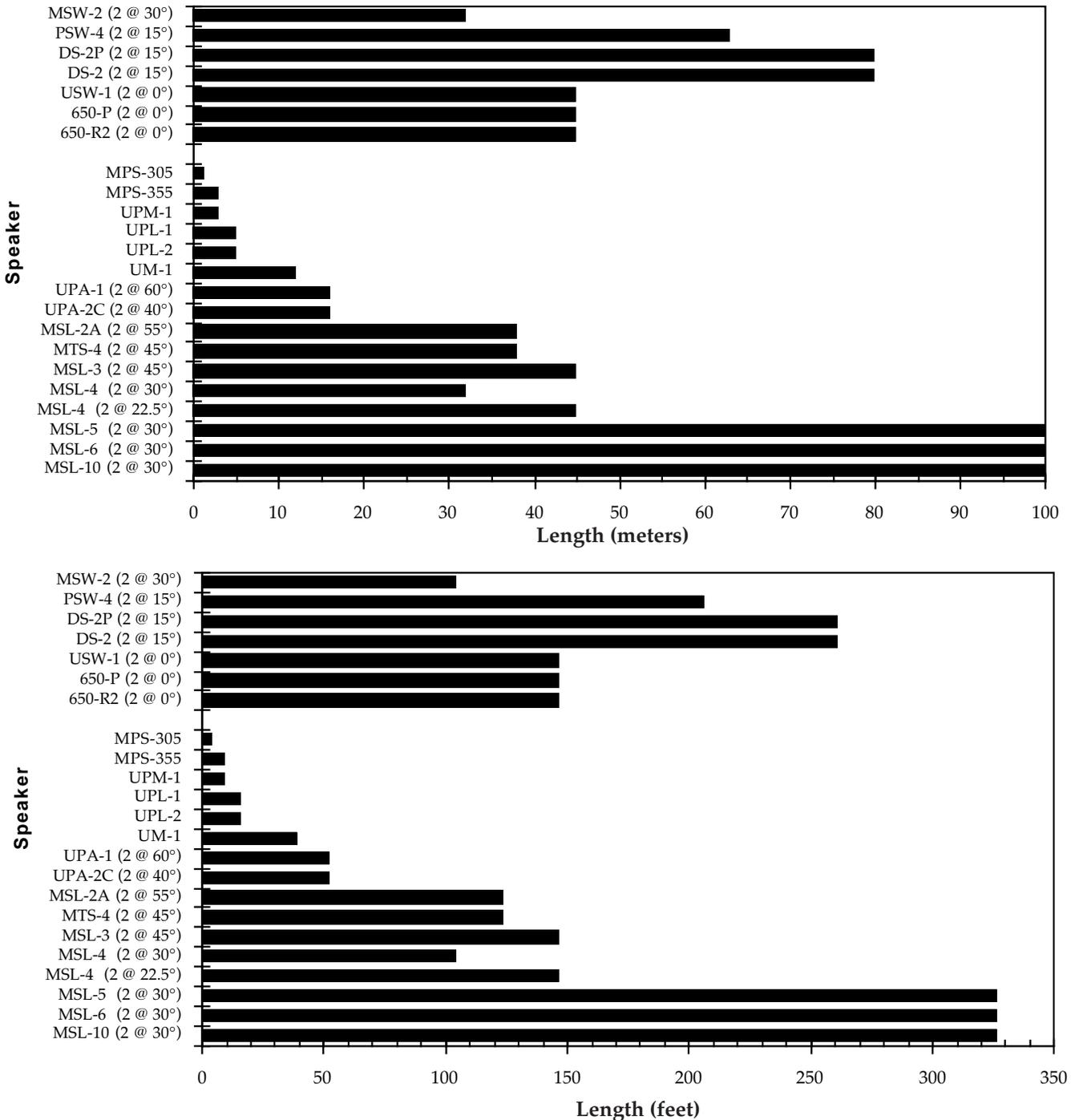
Fig 3.3c Meyer speaker SPL/distance reference (meters and feet).
