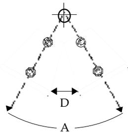
In many situations it is impractical to use a protractor to verify that you have achieved the desired splay angle. Reference chart 3.6n allows you to determine the splay angle by measuring the gap between the speaker fronts. It is assumed that the rears are adjacent. The gap (D) for each angle (A) is shown in inches and centimeters for each speaker model. For cabinets with a protruding front grill (such as UPAs, MSL-2A and CQs) the gap is measured from the wood edge, not the grill edge.
