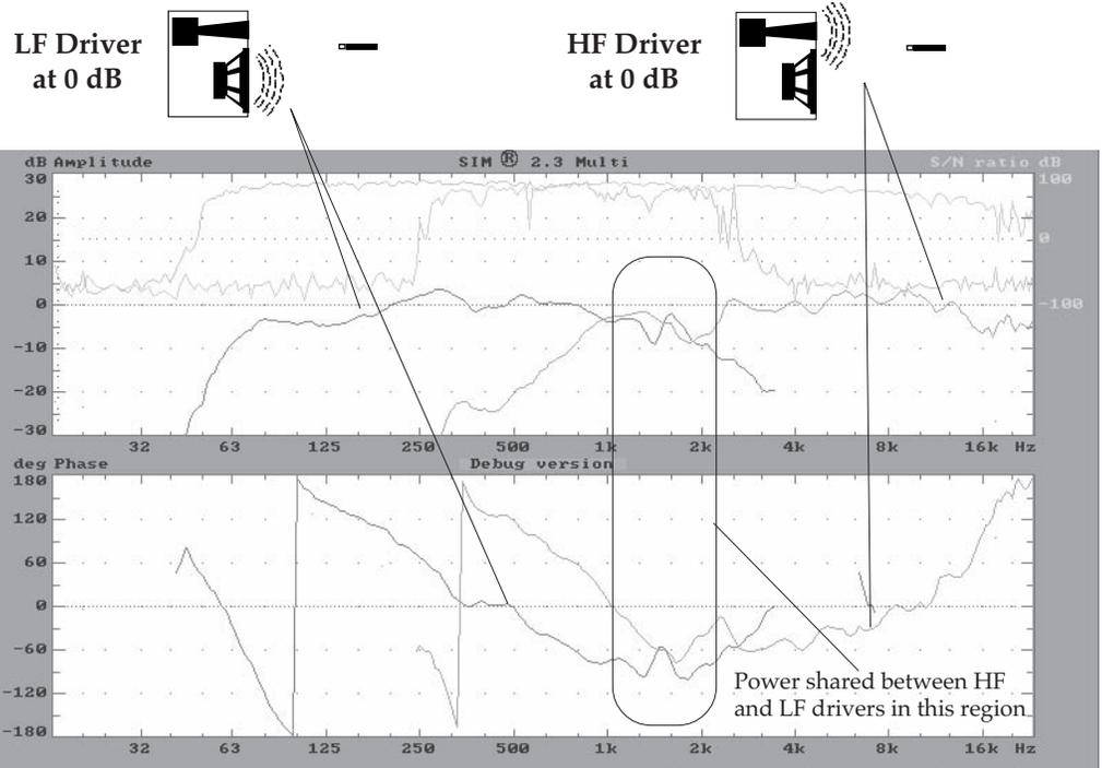
Fig 4.10a Normal crossover of the UPA-1C. Both amplifiers have the same gain.
