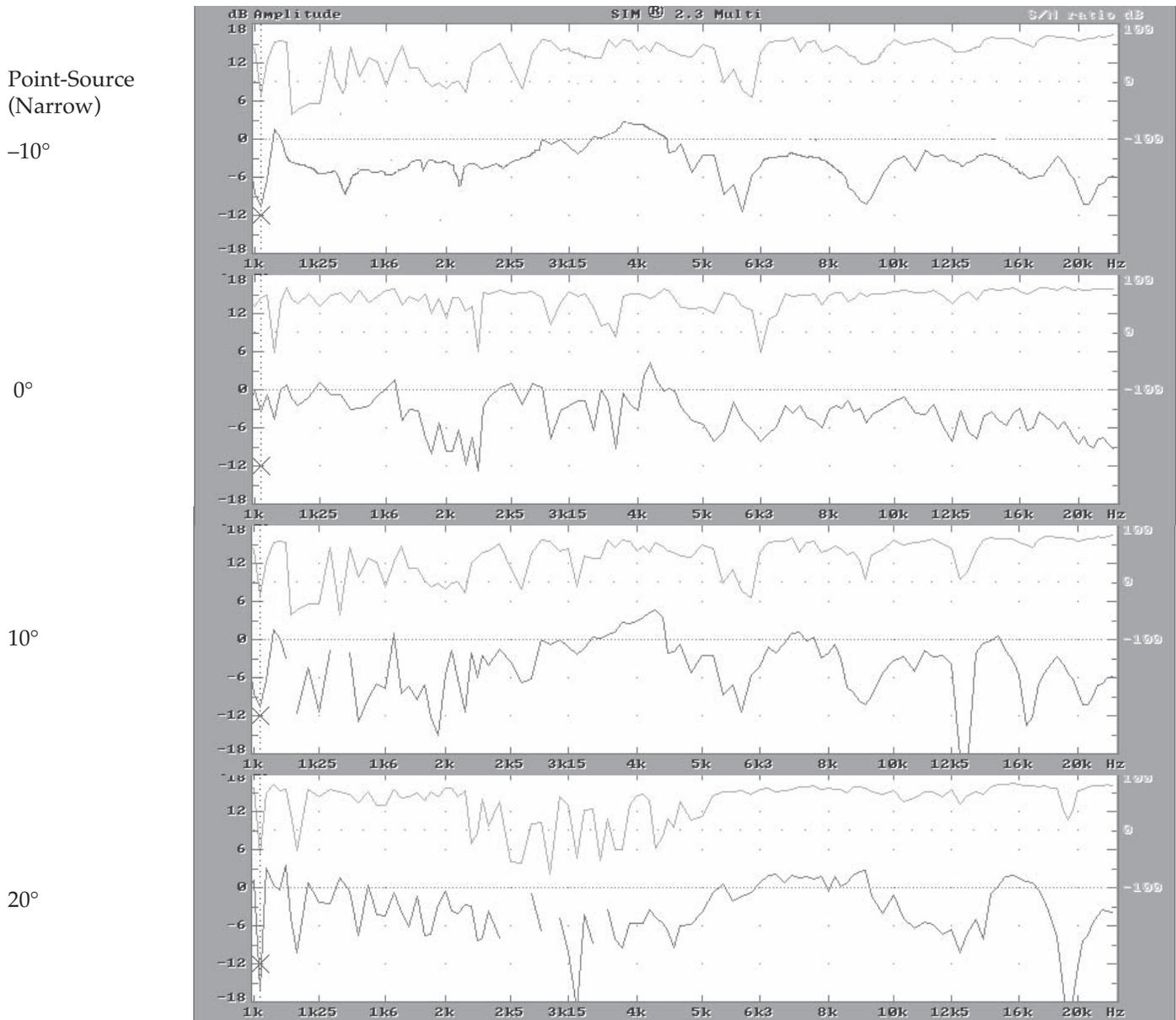
Fig 2.2k Narrow point-source array HF frequency response.
