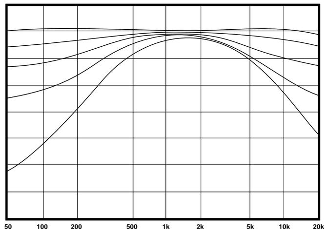
Fig 1.6b The CP-10 shelving section family of curves.
