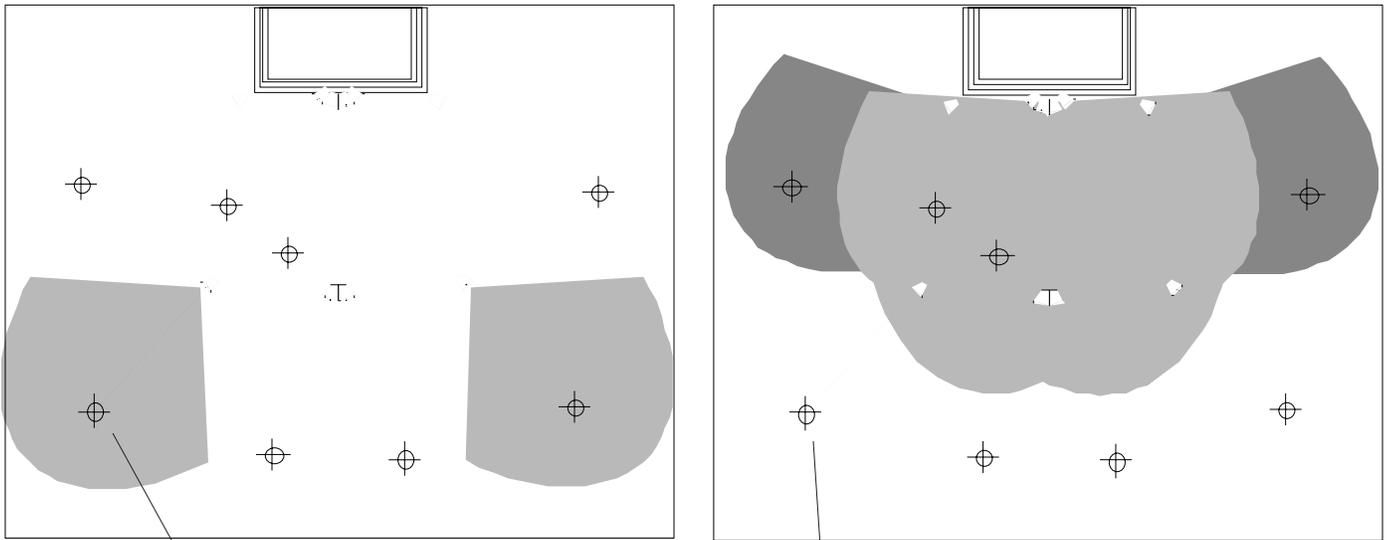
Plan view of the hall indicating the mic position and speaker status during the measurements shown on the opposite page.
