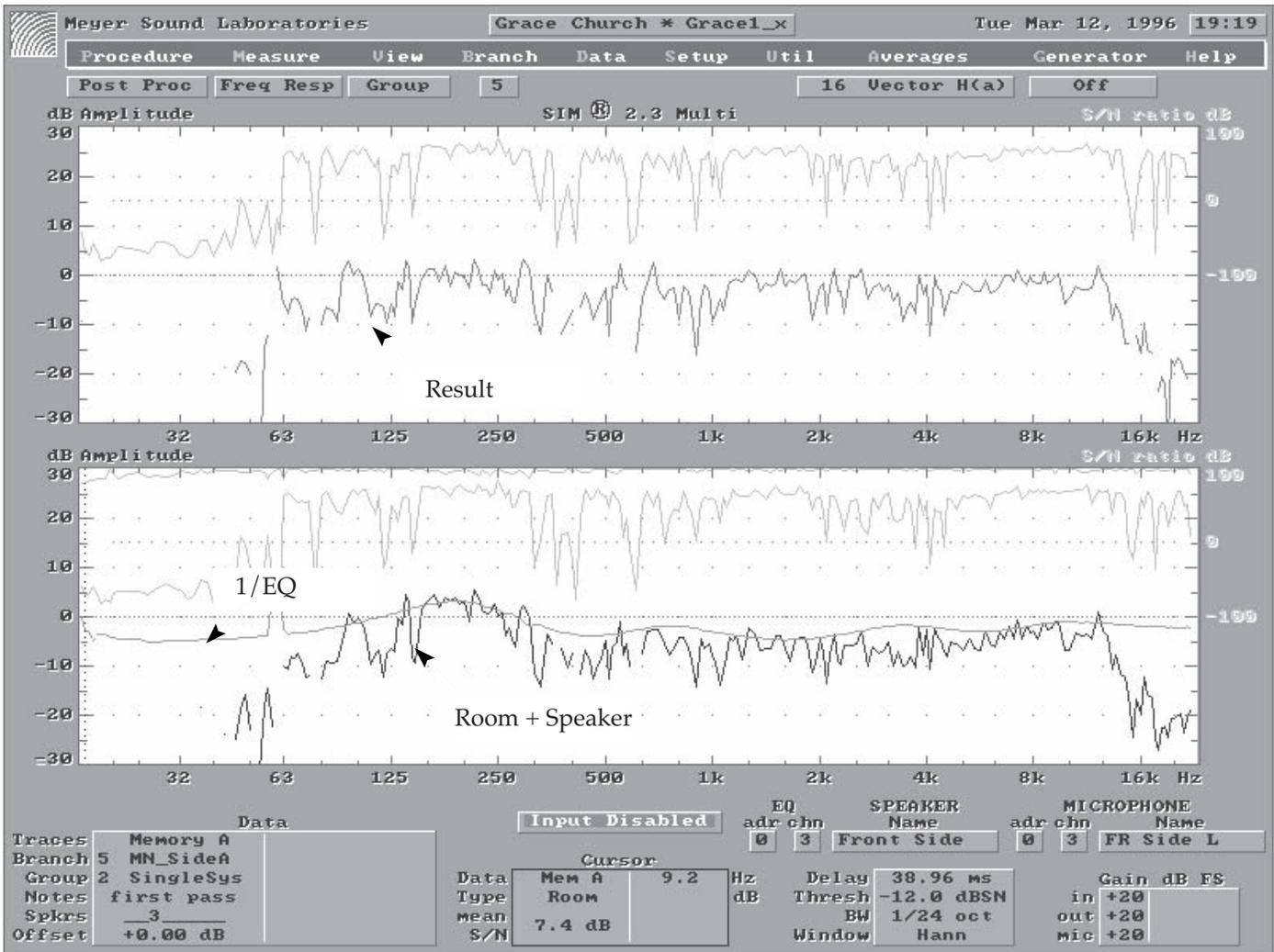
Fig 5.10h Equalizing the main side system.
