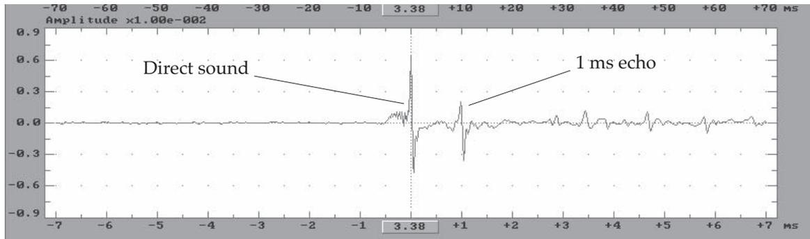
Fig 2.11 Identifying delay offset to find frequency response ripple.
