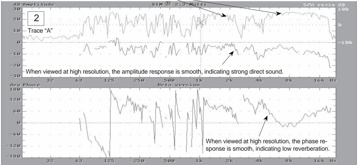
Fig 1.9k (2) High resolution view of amplitude, phase and S/N ratio of speaker "A" alone.
