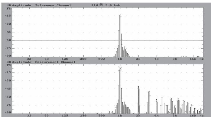
Fig 4.5b Distortion and maximum output testing with SIM.
