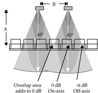
3.7j Speakers were moved closer together to optimize the response for the narrower speakers.
