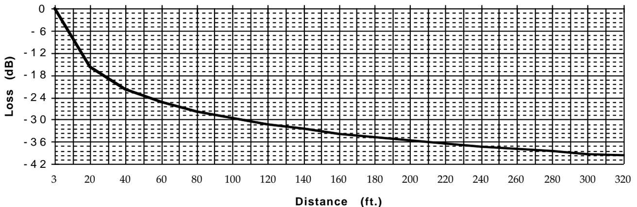
Fig 3.3b Propagation loss over distance (free-field) referenced to 1 meter SPL (in meters and feet).
