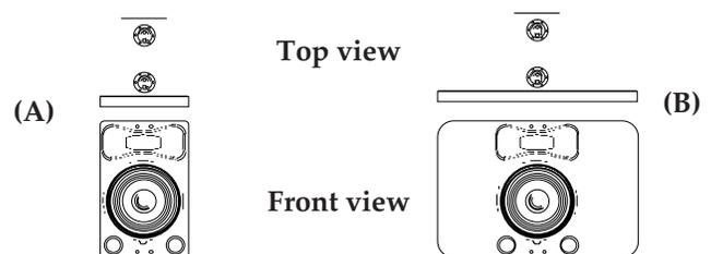
Fig 3.6e UPA-1C Enclosure design: (A) actual; (B) if the enclosure angle were equal to the coverage angle.
