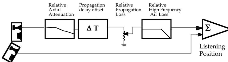
Fig 2.2b Model of speaker interaction between an upper main and downfill system.
