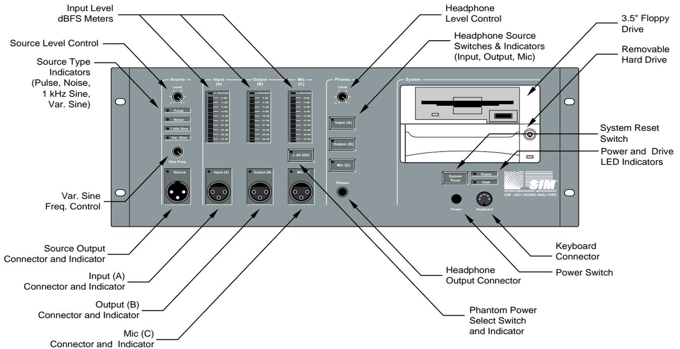
Fig 1.9m SIM 2201 sound analyzer.
