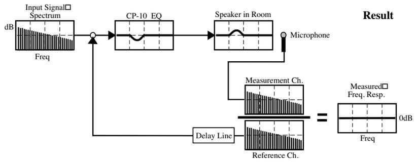
In practice, all three of the responses (room, EQ and result) are measured and displayed simultaneously as shown in Figs 5.8c to
