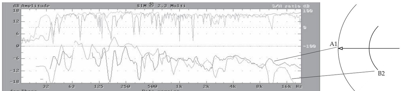
Fig 3.3e Comparison of on-axis far (A1) and off-axis near (B2).
