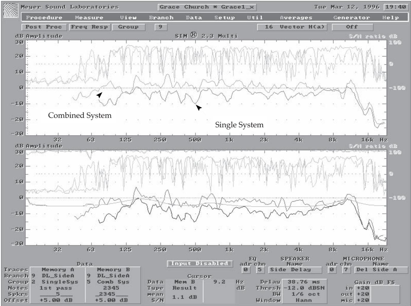
Fig 5.10n Combining the delays with the mains.
