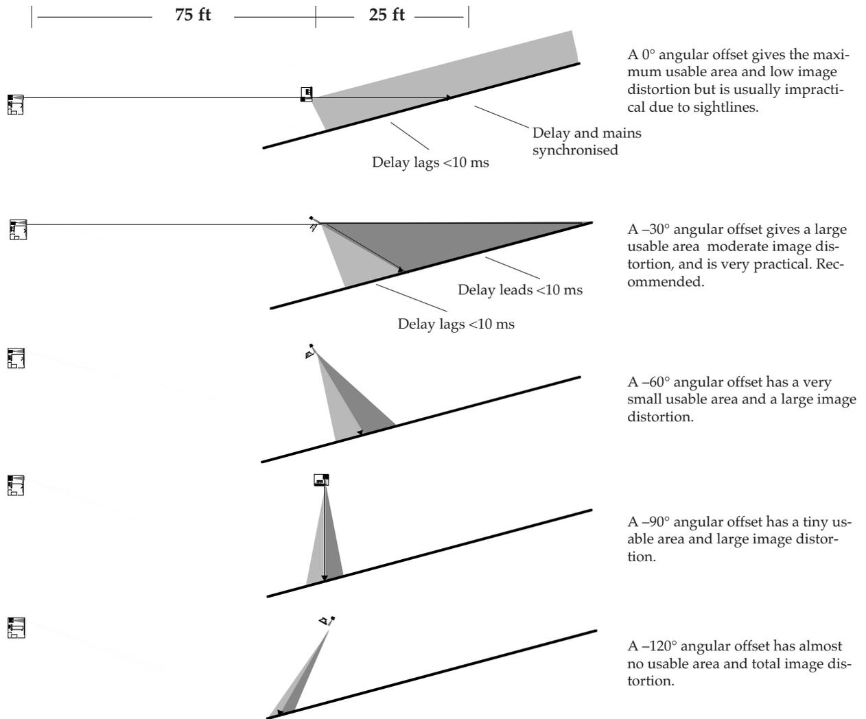
Fig 3.7m Usable vertical angle for distributed delays.
