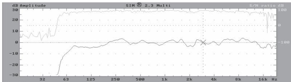
Fig 1.2e UPA-1C on-axis amplitude response.
