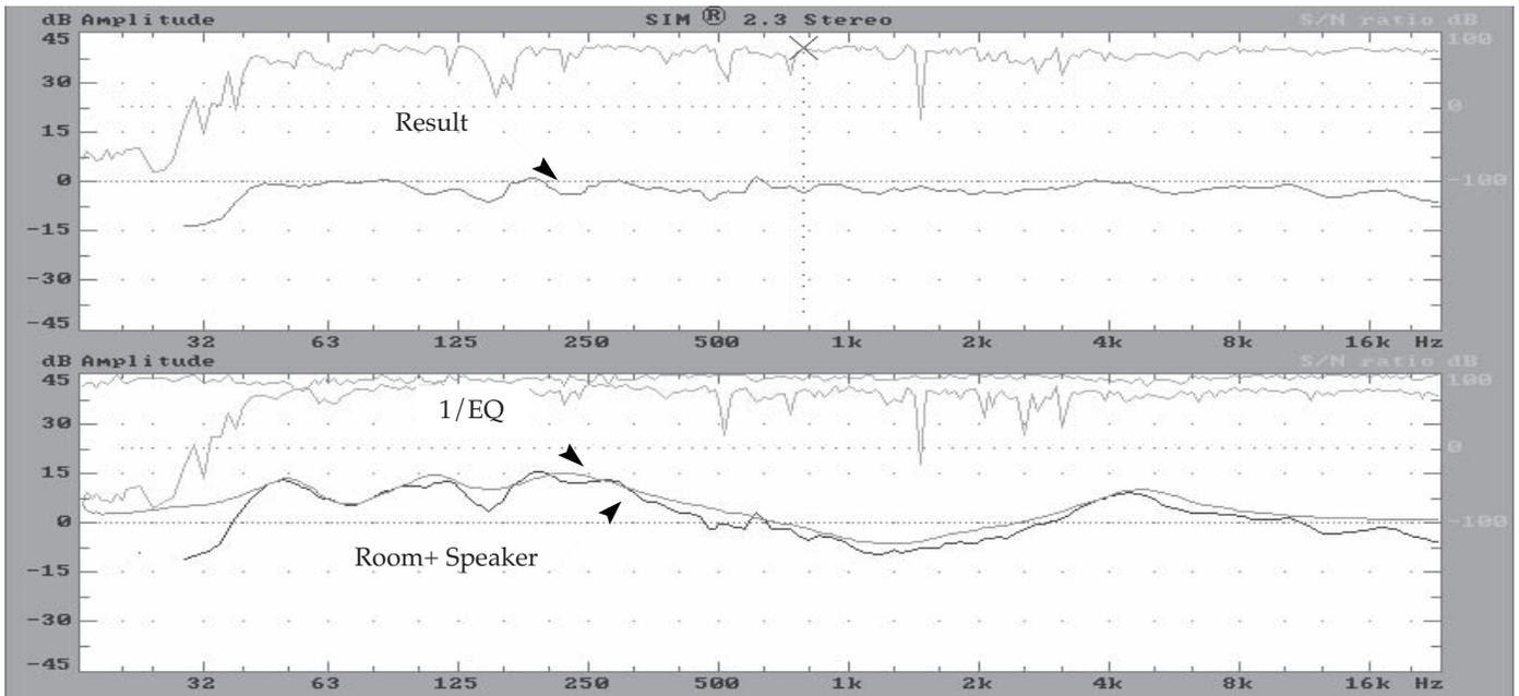
Fig 5.8c Group view of the three SIM transfer functions with the 1/EQ response. The process of creating a complementary response is aided by the visual inversion of the EQ trace. This allows you to simply match the equalizer response to the room+speaker response. This creates a flat response in the result.
