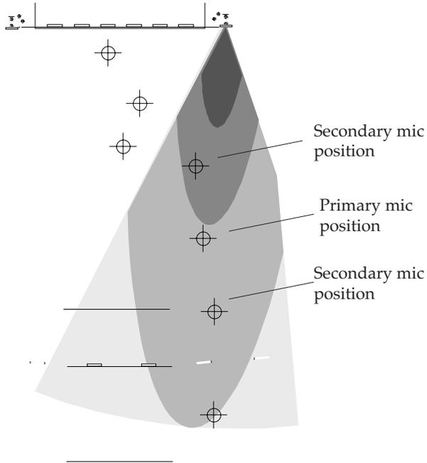
Step 1: The stalls outer system is measured alone as a single system. The primary mic is positioned at one-half the depth of coverage, on-axis. Two secondary mics are placed in alternate positions. Because the system is a split-parallel array only one of the speakers is used for the initial alignment. Coverage verification, level setting and EQ can be done at this time.
