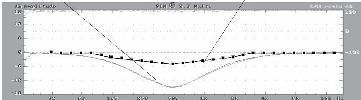
Fig 1.6e Contrasting a graphic equalizer and the CP-10 Parametric
