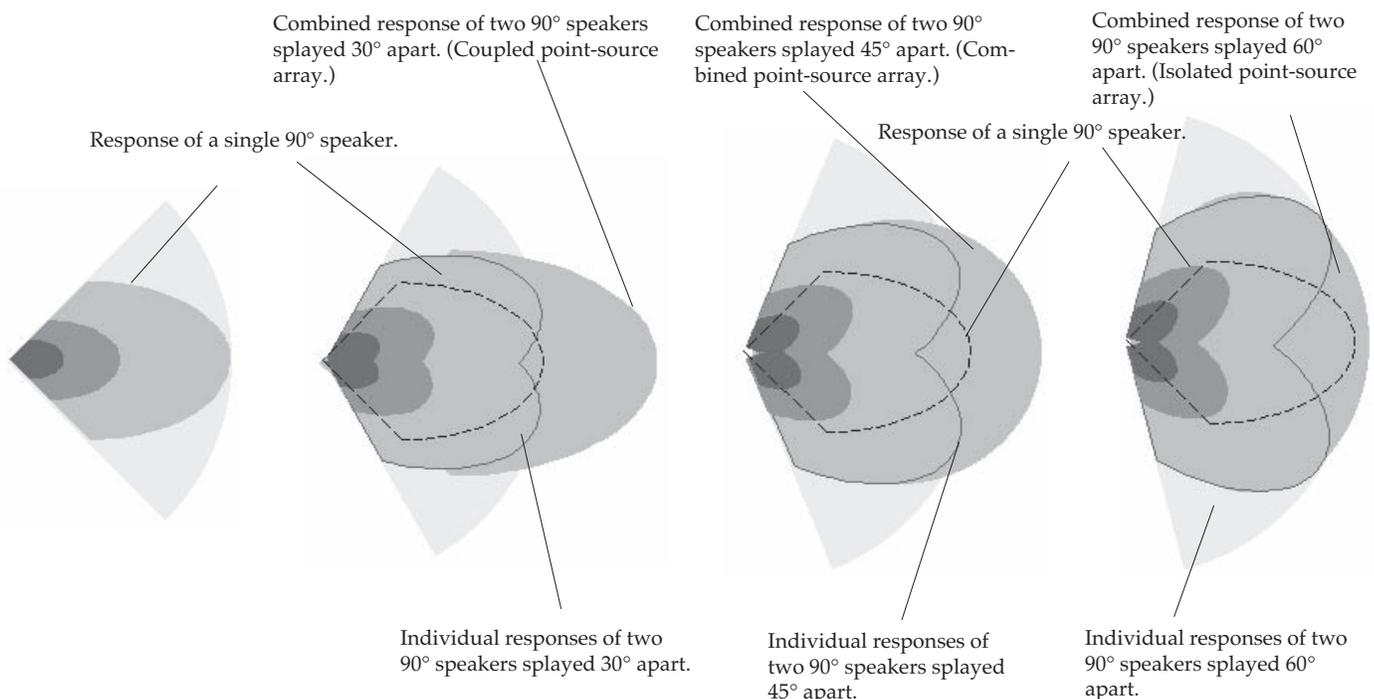
Fig 3.6h Coupled, combined and isolated point-source arrays.
