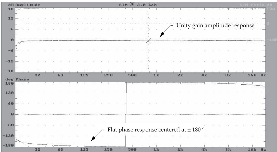
Fig 4.8c Polarity reversal of a balanced line. The amplitude trace is unaffected, however, the phase trace is centered at 180°. This indicates a polarity inversion.
