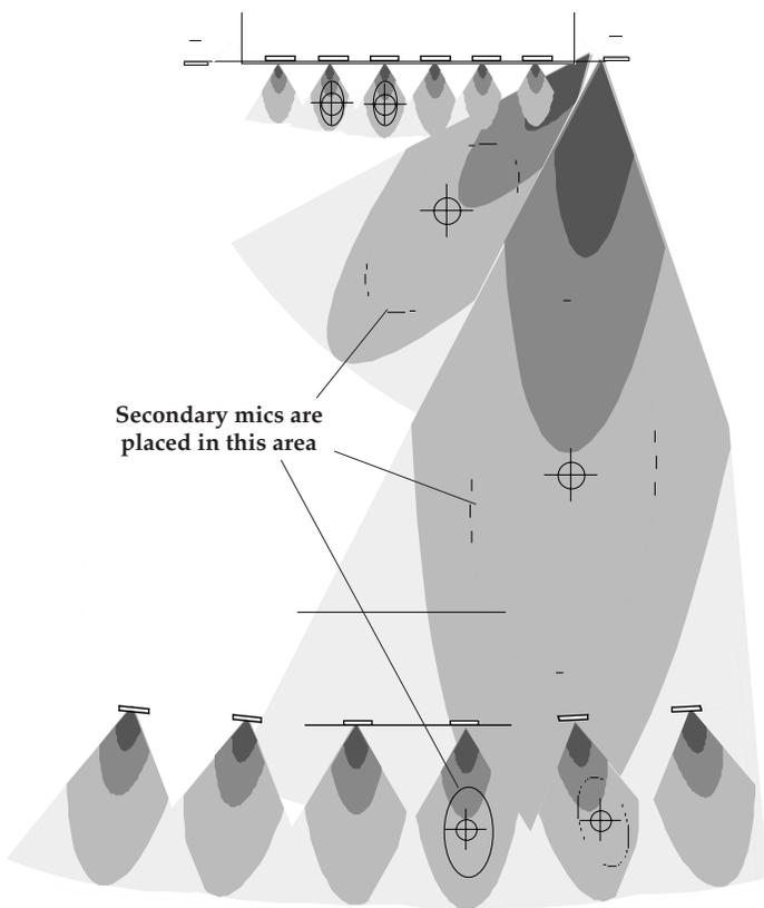
Fig 5.3c Plan view of secondary mic positions.
