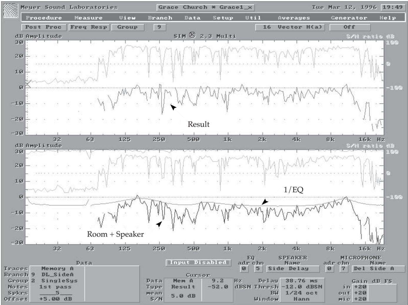
Fig 5.10I SIM equalization of the side delay speakers.
