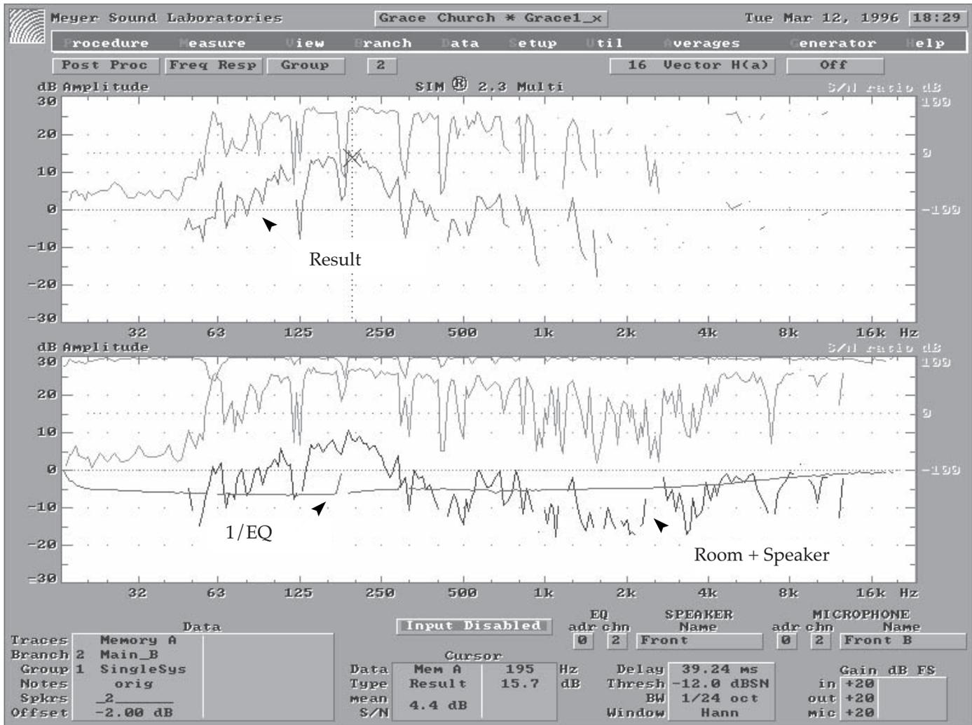
Fig 5.10e Original equalization of the main cluster.
