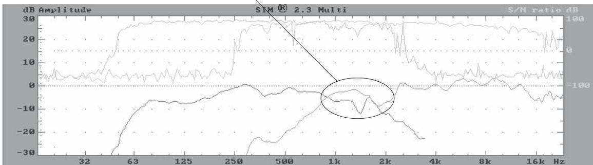
Fig 1.4i UPA-1C with unmatched voltage gains at crossover.
