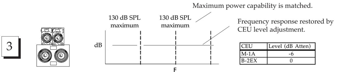
The most effective way to rebalance the system above is to turn down the M-1A CEU by 6 dB. This will restore the frequency response to its original response. The maximum power capability over frequency has been changed so that both the UPAs and subwoofers will reach their limits at the same time.
