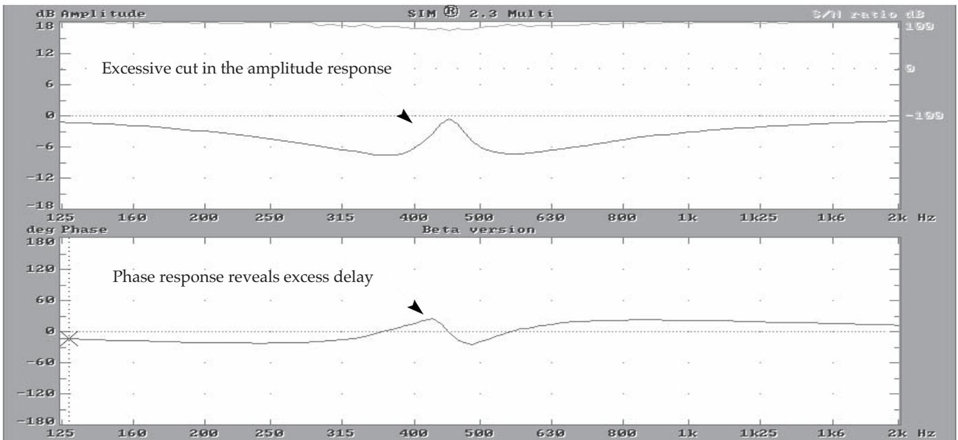
Fig 1.6k Result of error in bandwidth.
