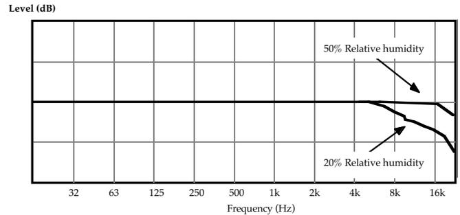
Fig 2.4b Relative humidity effect on frequency response.
