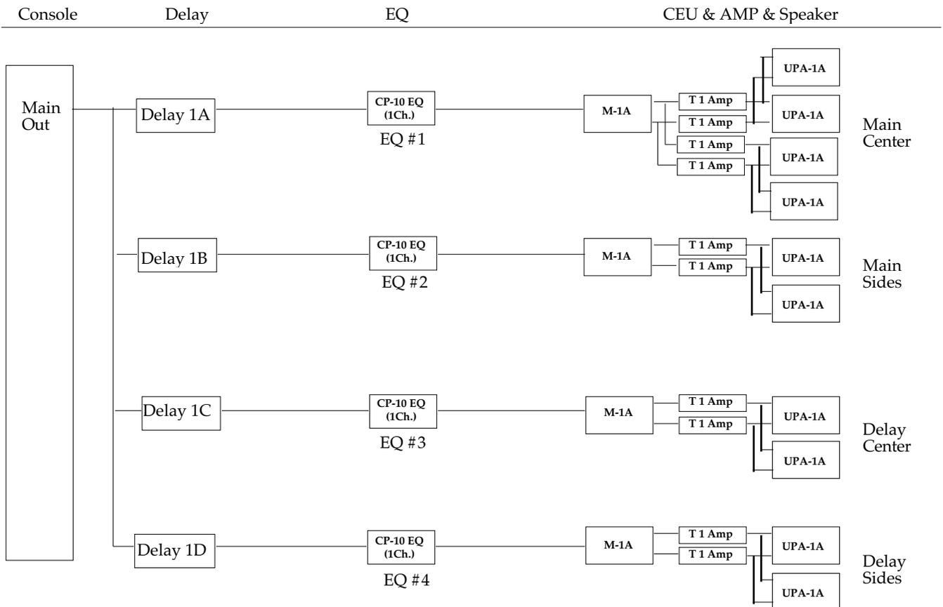
5.10b Flow block diagram of the system from mix console to the speakers.
