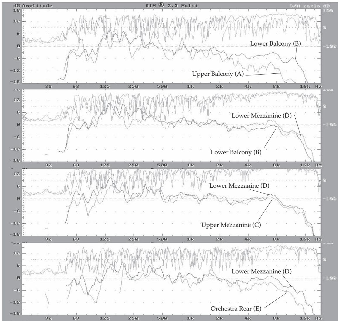
Fig 5.3g Vertical coverage map using multiple microphones.
