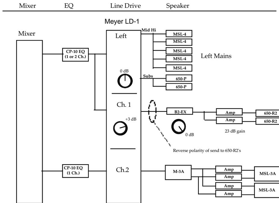
Fig 7.1a Combining externally-powered with self-powered speakers.
