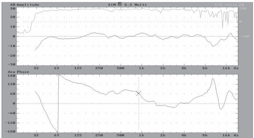
Fig 1.2c Combined acoustical response of the MSL-2A.<sup>1</sup>
