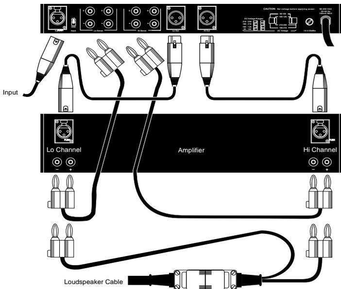
Fig. 1.3l MultiSense connection.
