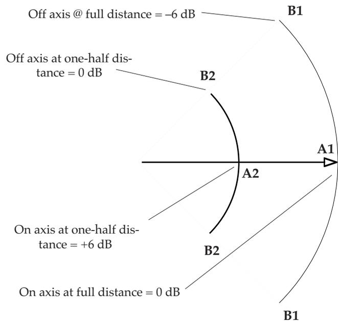
Fig 3.3b Relationship between propagation loss and coverage pattern.
