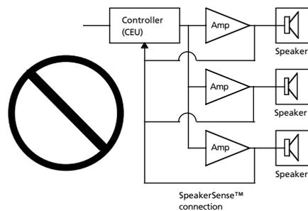
Fig 1.3k Sensing one of several amplifiers. Sense line connected to amplifier with lower gain.
