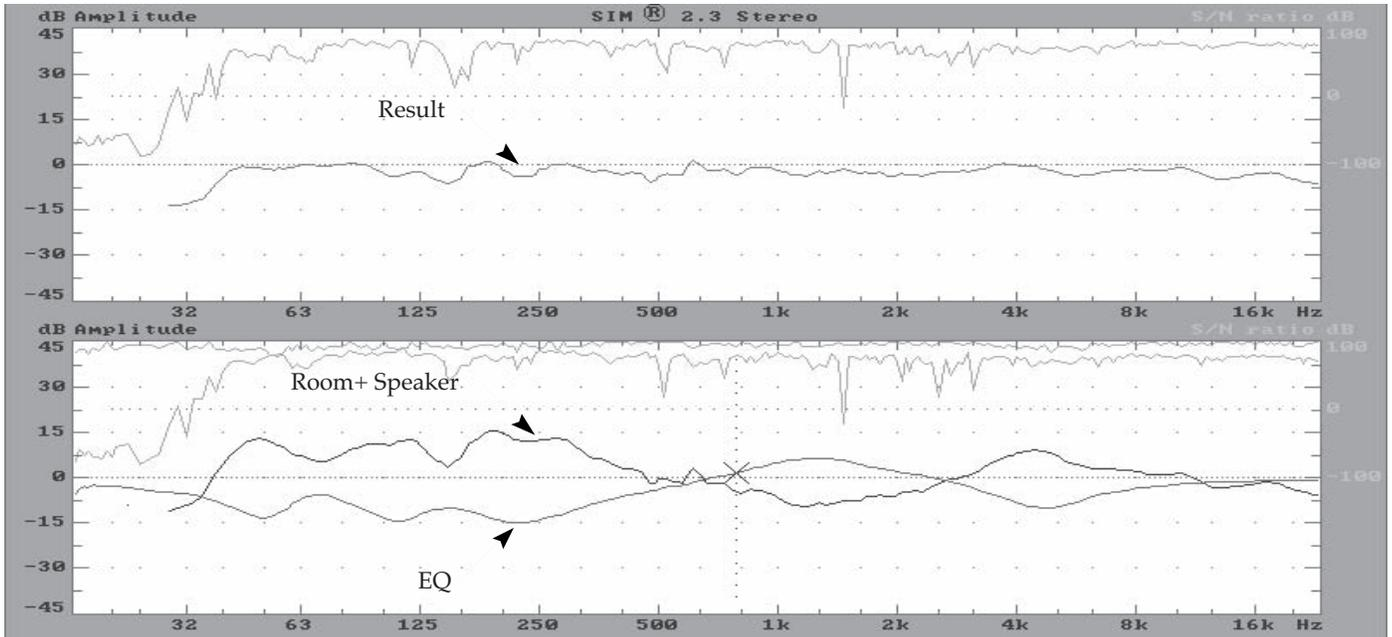
Fig 5.8b Group view of the three SIM transfer functions. The equalizer response is adjusted until it has created an inverse of the room+speaker response. This creates a flat response in the result.
