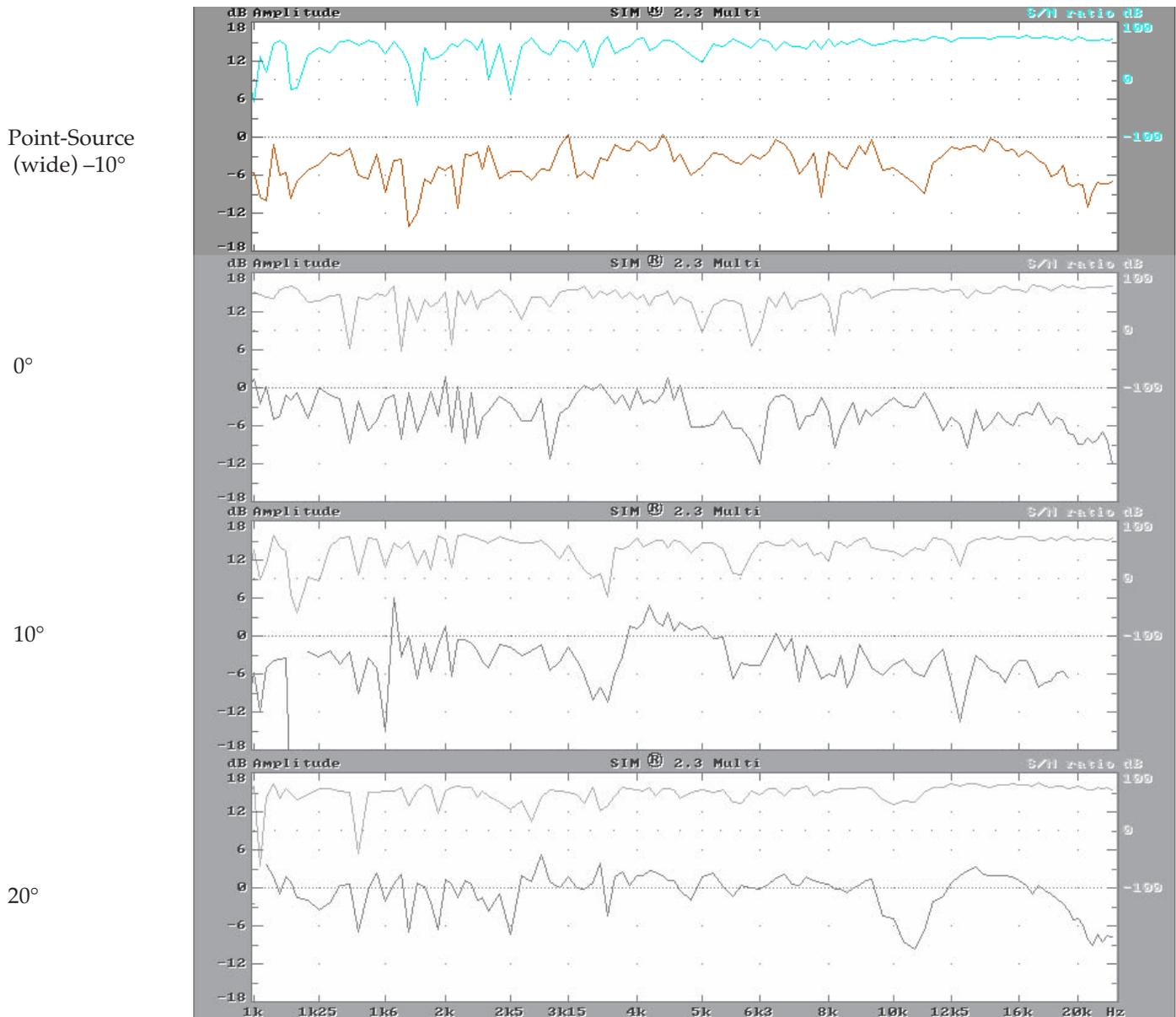
Fig. 2.2r Wide point-source array HF frequency response.
