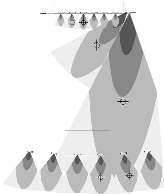
Primary mic is on the horizontal axis, at one-half the depth of field of coverage as shown in plan and elevation views.
