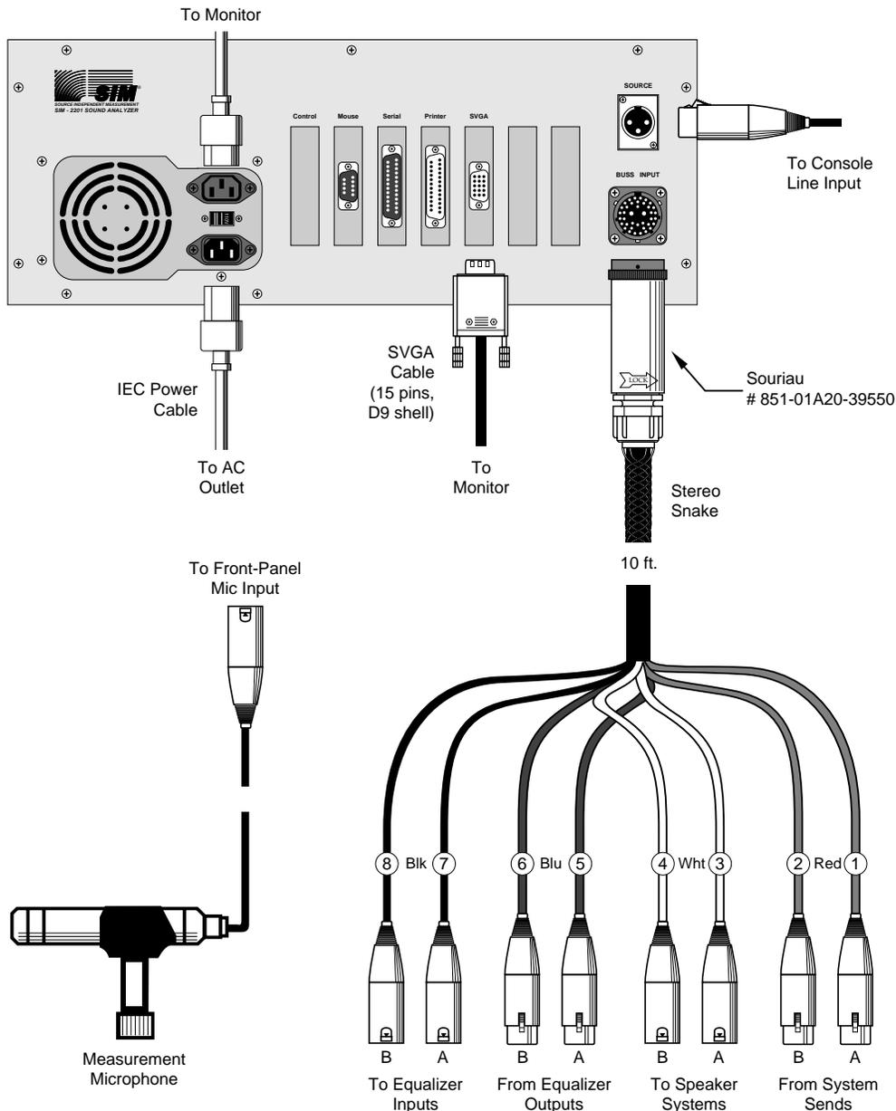
Fig 1.9q The v2.3 stereo hookup.
