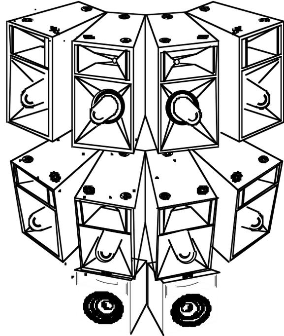
Fig 3.6b Point-source Array.
