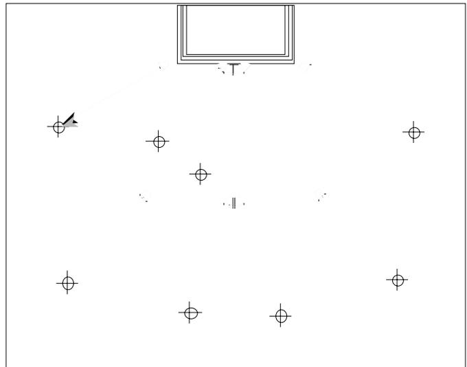
Step 3: Delay the main side system to synchronize to the signal from the main center system. This proved far superior for intelligibility than the previous setting.
