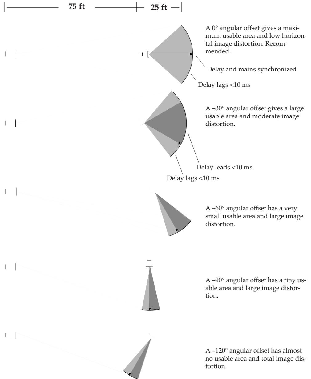
Fig 3.7n Usable horizontal angle for distributed delays.
