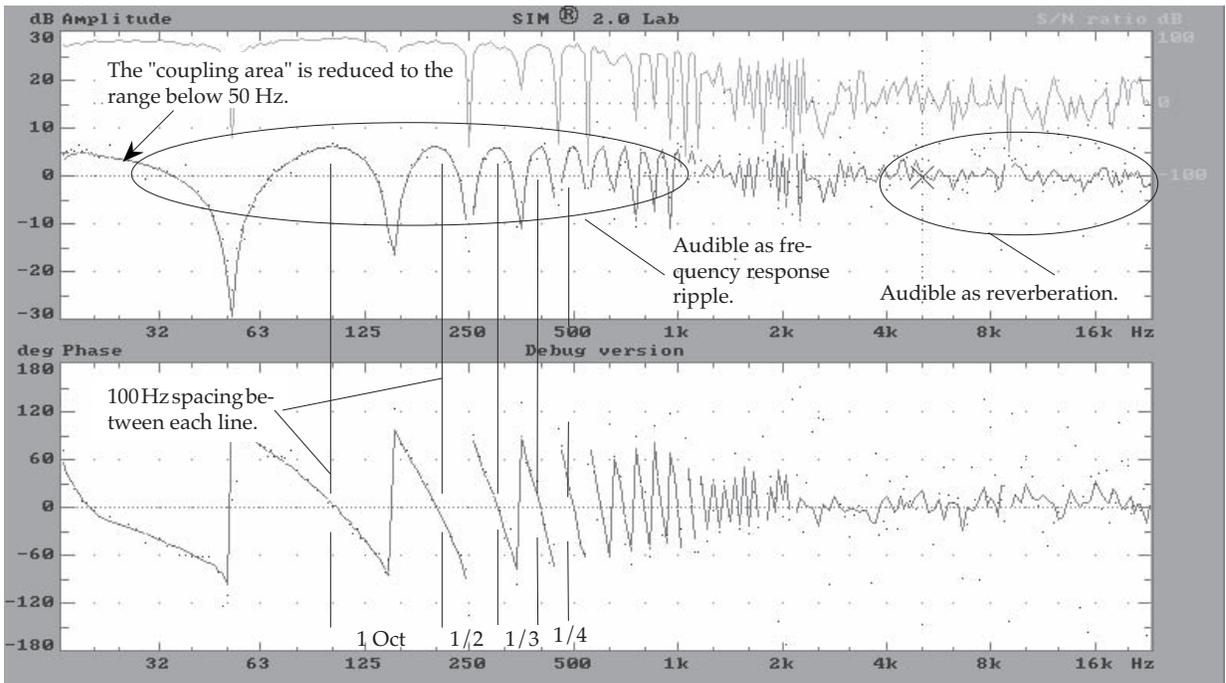
Fig 2.1g Comb filtering with 10 ms time offset between signals with 0 dB level offset.
