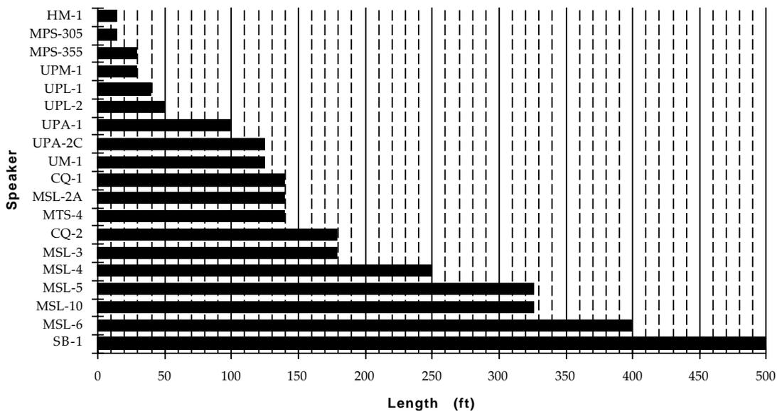
Fig 3.7l Delay speaker reference (feet).
