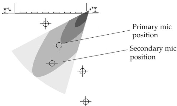
Step 2: The stalls inner system is measured similarly to the outer, above. The level of the inner system is set so that the inner and outer systems are matched at their respective primary positions. This will create equal average levels across the orchestra.
