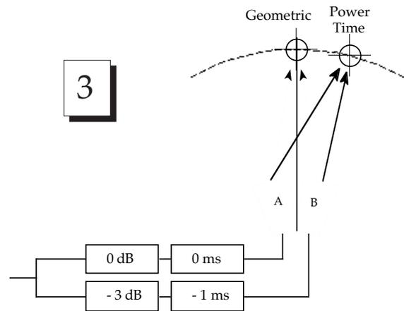
Fig 5.7i Delay tapering—Time center moved to power center.
