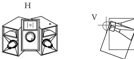
Horizontal Array with Vertical Stagger
