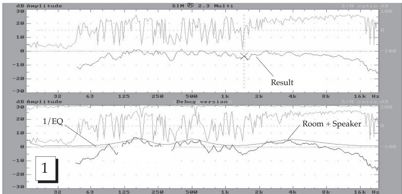
Fig 5.9a Single system analysis of the underbalcony system.
