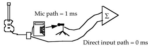
Fig 2.1a Four examples of typical causes of comb filtering.
