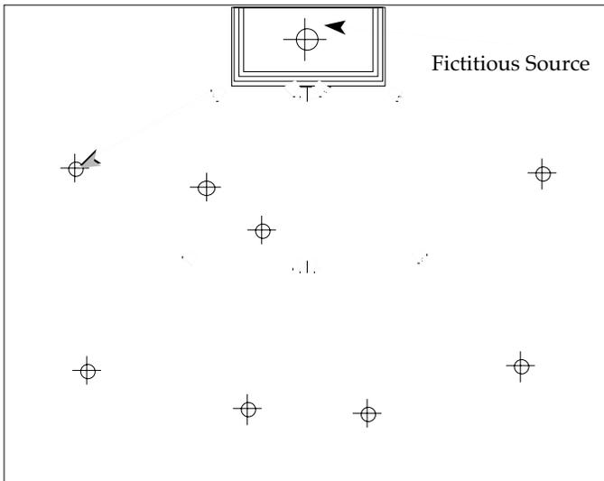
Step 2: Delay the main side system to synchronize to the fictitious source. This was chosen because the fictitious source would help create a sonic image in the direction of the stage. This proved unworkable, however, due to the interaction of the main sides with the main center system, as shown in the previous section.
