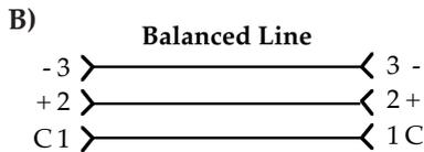
Fig. 1.7a Balanced mic line.
