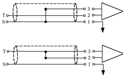
Fig 4.8e Unbalanced cable with mono phone jack.
