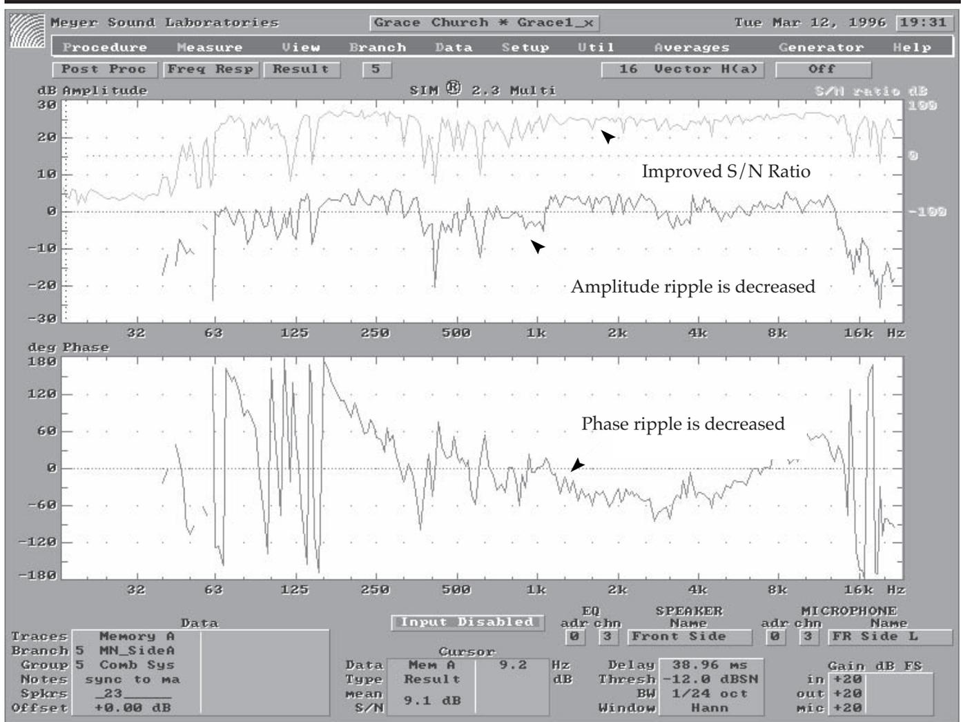
Fig 5.10k Delay tapering of the side system.
