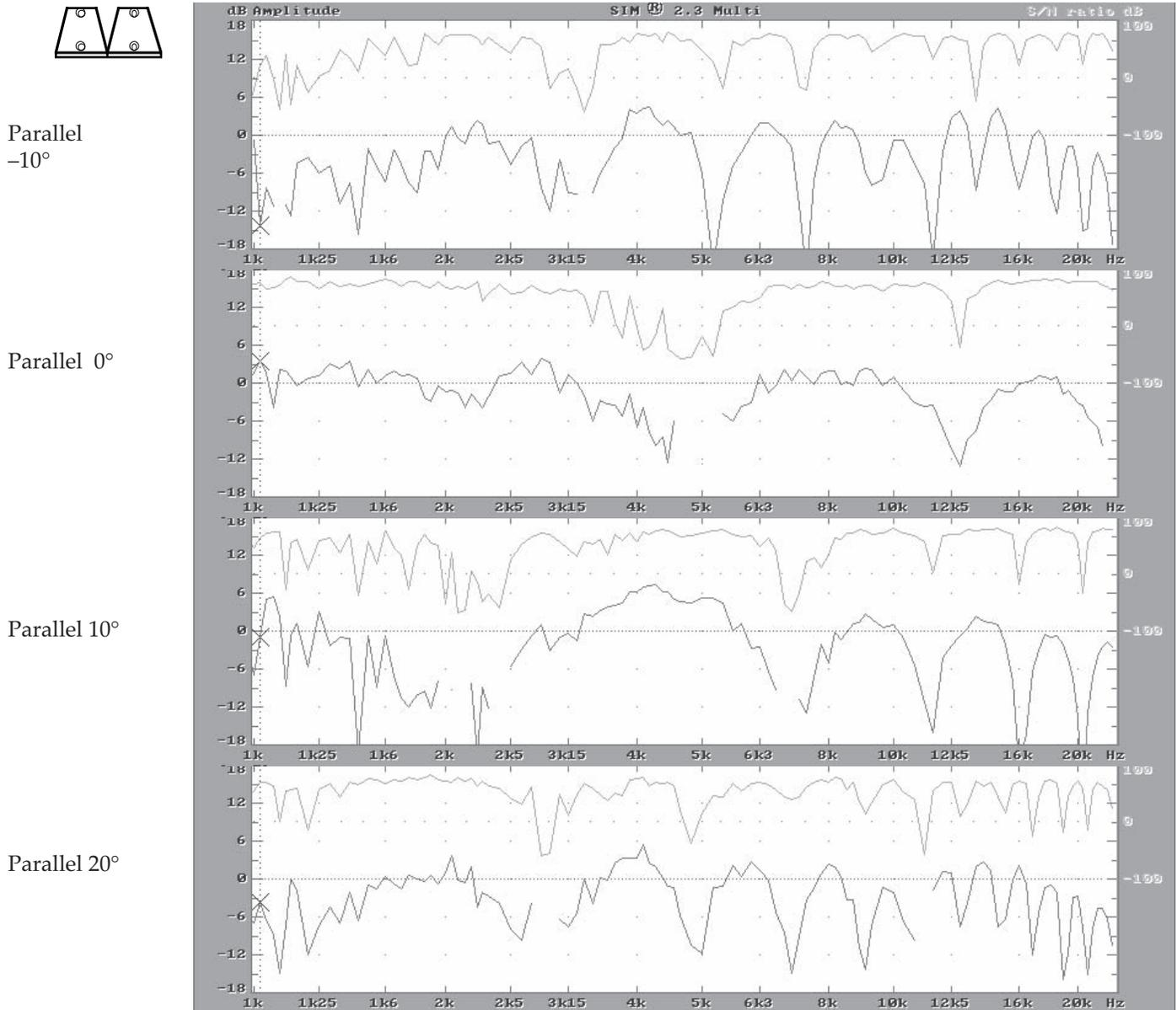
Fig 2.2t Parallel array HF frequency response.
