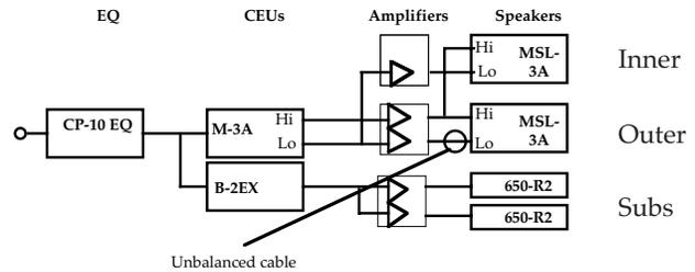
Fig 4.8i Flow block diagram of the system. The cable driving the left outer LF channel was unbalanced, creating the frequency response problems shown in Fig 4.8h below.
