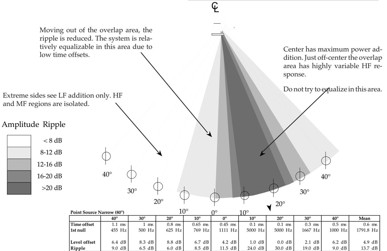
Fig 2.2j Narrow point-source array interaction.
