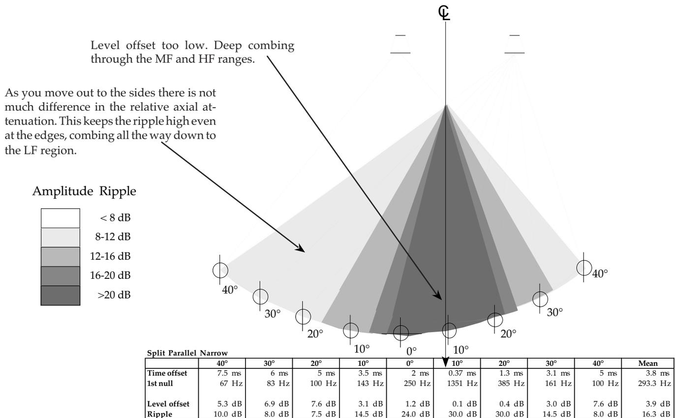
Fig 2.2w Split-parallel (narrow) array interaction.
