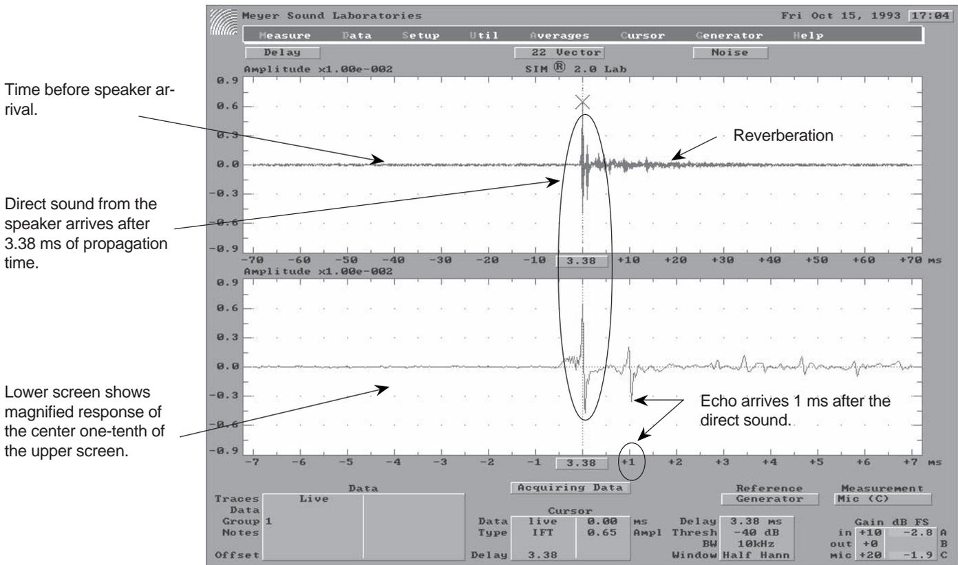
Fig 1.9h Reading the delayfinder screen.
