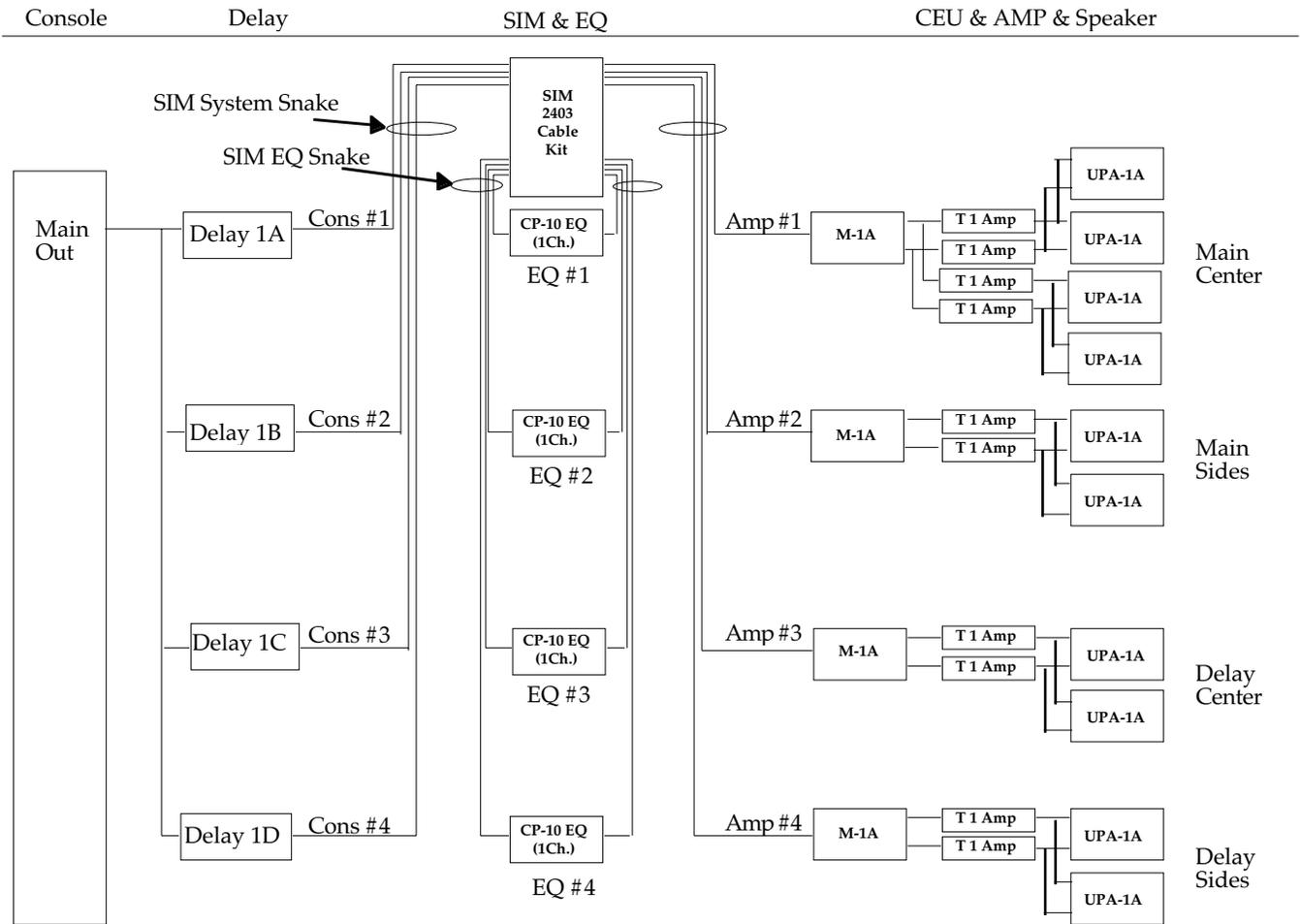
5.10c Flow block diagram of the system after SIM System II is patched in.
