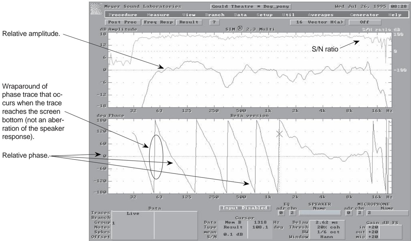
Fig 1.9i Reading the frequency response screen.
