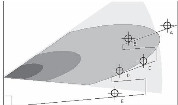
Fig 5.3h Mic positions and intended coverage.
