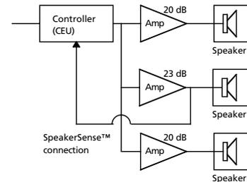
Fig 1.3j Sensing one of several amplifiers. Sense line connected to the correct amplifier.
