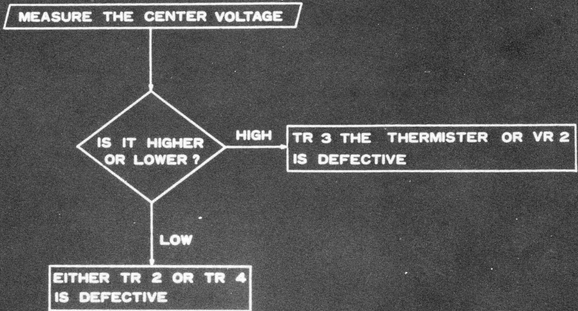
47. MEASURE THE CENTER VOLTAGE. IS IT HIGHER OR LOWER THAN  $\frac{1}{2}$  VCC? IF IT IS HIGHER THEN TR-3, THE THERMISTER OR VR2 IS DEFECTIVE. IF IT IS LOWER, THEN TR2 OR TR4 IS DEFECTIVE.
