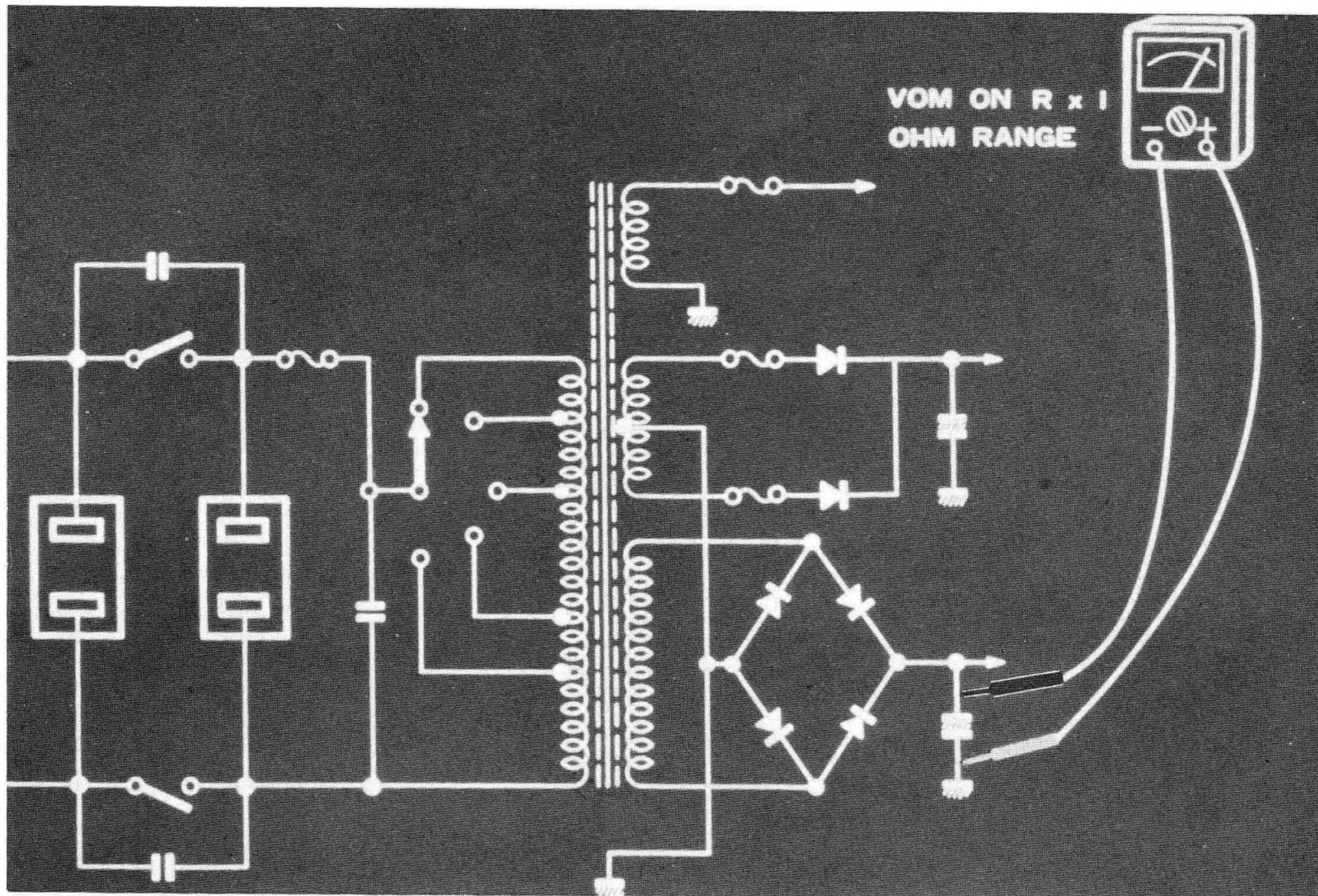
27. THIS IS A RATHER RARE CASE BUT THE FILTER CAPACITOR CAN BE LEAKING OR SHORTED. TO CHECK THE CAPACITOR, SET THE VOM ON R<sub>x</sub>1 OHM RANGE THEN PLACE THE TESTER LEADS ACROSS THE CAPACITOR. IF IT IS GOOD, THE VOM FIRST SWINGS TO ZERO THEN SLOWLY GOES BACK UP TO INFINITY. IF YOU GET A STEADY ZERO OR SEVERAL OHMS, THEN THE CAPACITOR IS SHORTED.
