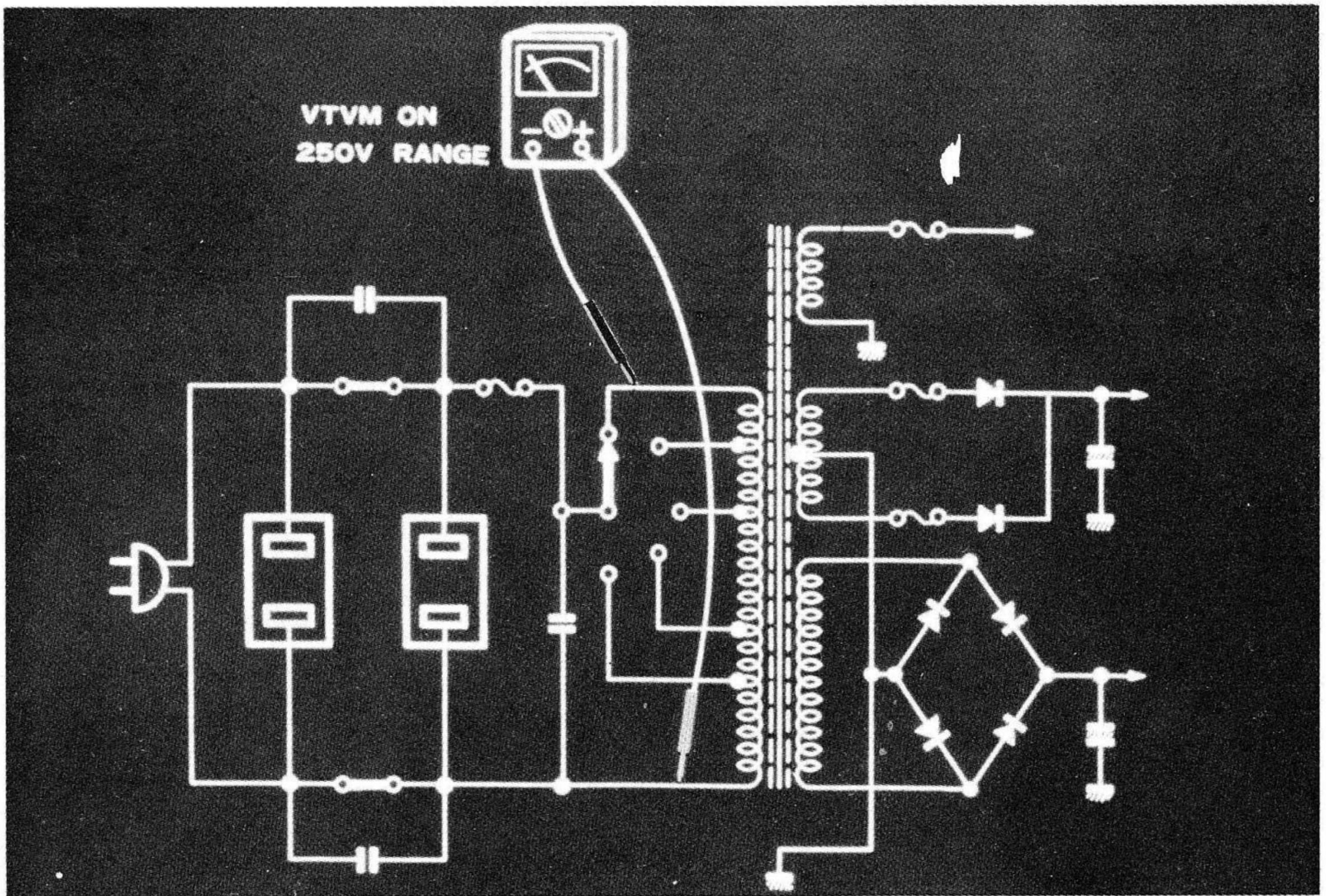
15. IF VOLTAGE IS PRESENT IN THE "UNSWITCHED" SOCKET, THEN CHECK VOLTAGE ACROSS THE PRIMARY WINDING OF THE POWER TRANSFORMER. USE A VTVM ON 250V RANGE.
