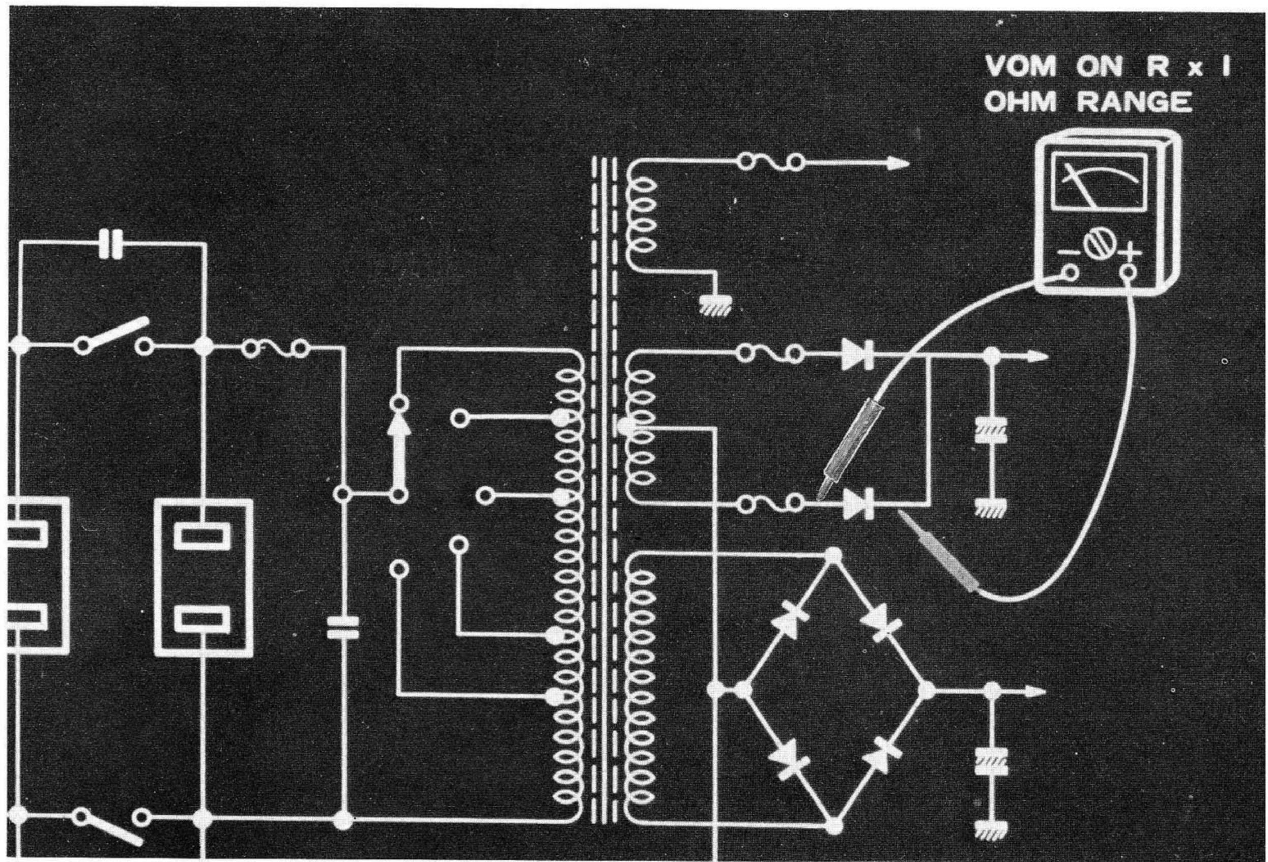
55. IF THE FAILURE IS IN THE POWER SUPPLY, THEN INSURE THAT THE POWER IS OFF AND CHECK THE DIODES FOR SHORTS.
