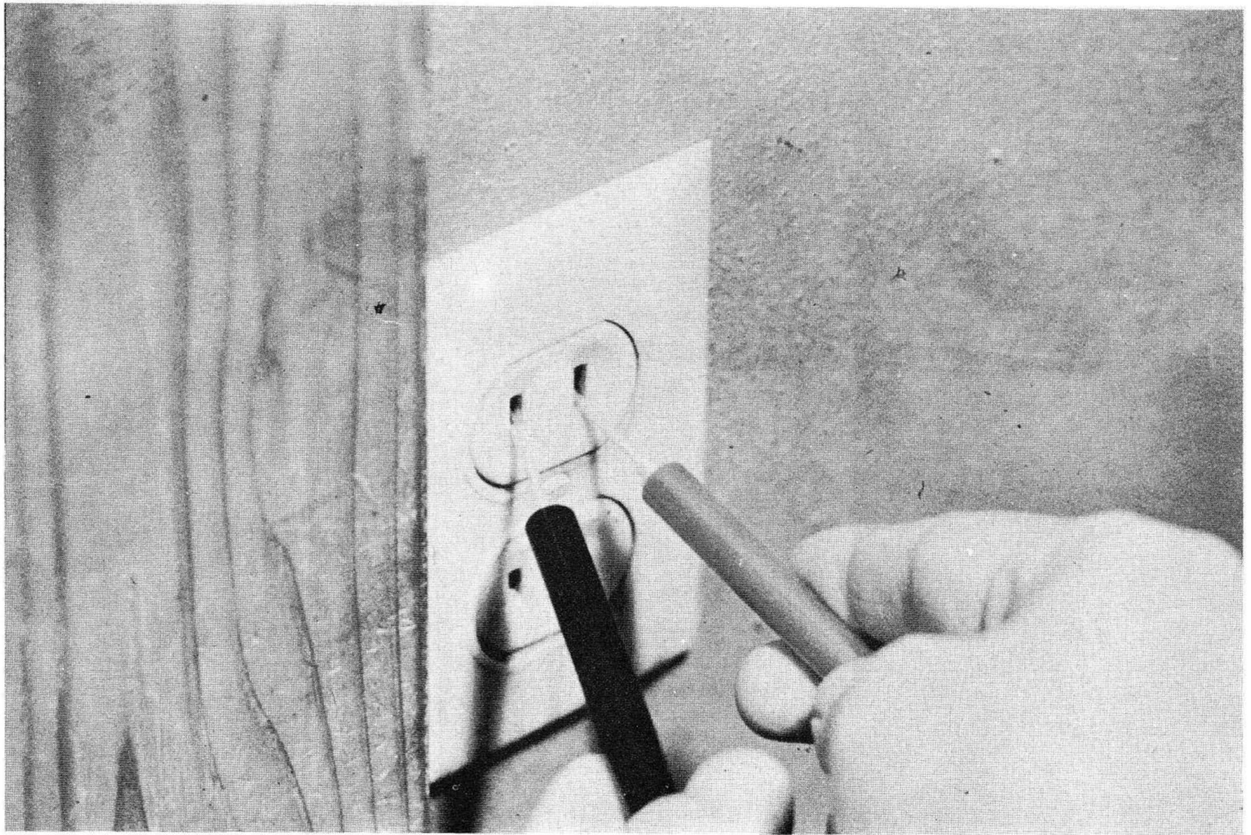
13. MEASURE THE LINE VOLTAGE TO SEE IF YOU ARE GETTING AC VOLTAGE OUT OF THE CORD. USE A VTVM ON 250V SCALE.
