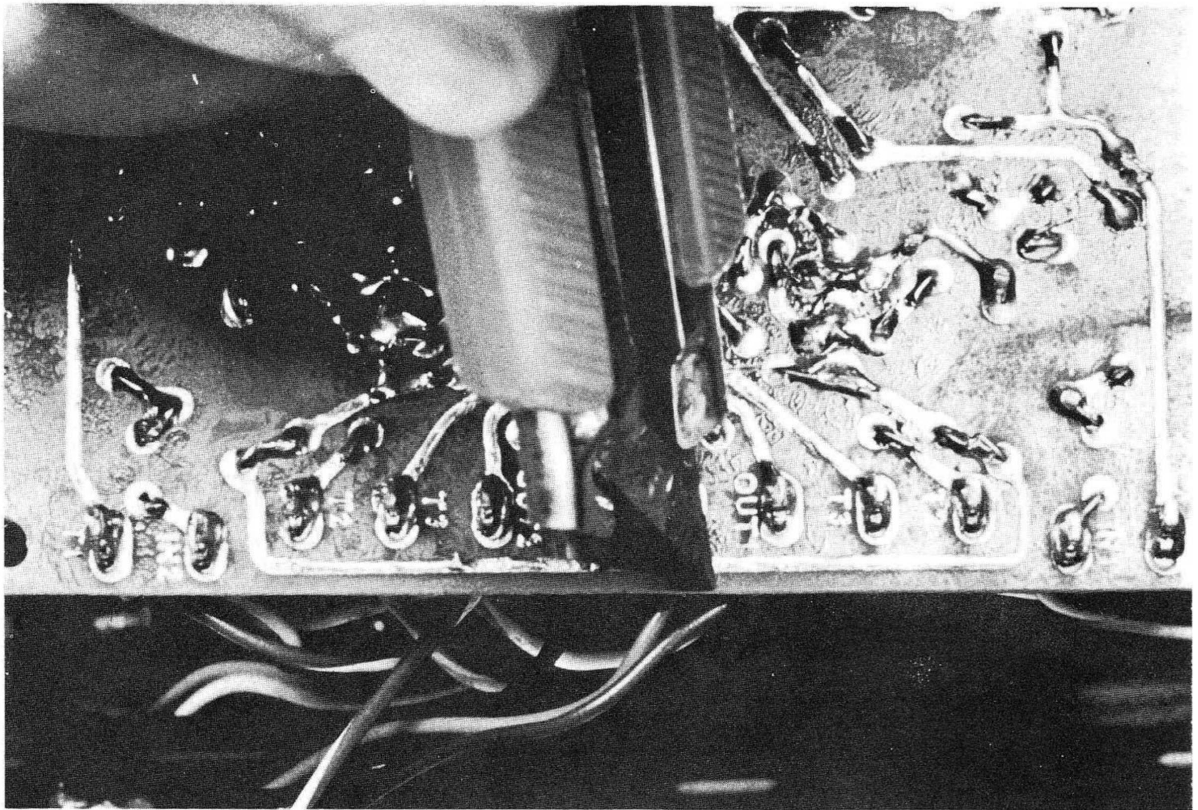
54. WHEN YOU CHECK UNITS THIS WAY, IT CAN BE VERY HELPFUL TO LOCATE THE PROBLEM FROM THE NEIBORHOOD OF THE RECTIFIER CIRCUIT THEN ON TO THE LOAD.
