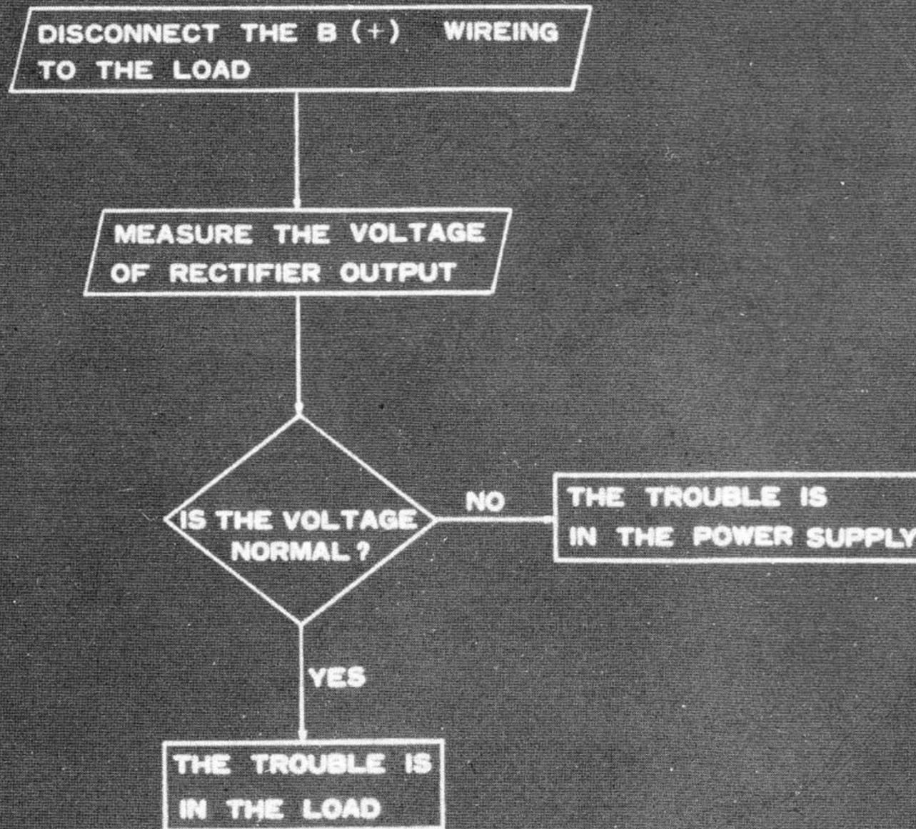
52. DETERMINE IF THE PROBLEM IS IN THE POWER SUPPLY OR IN THE LOAD.
