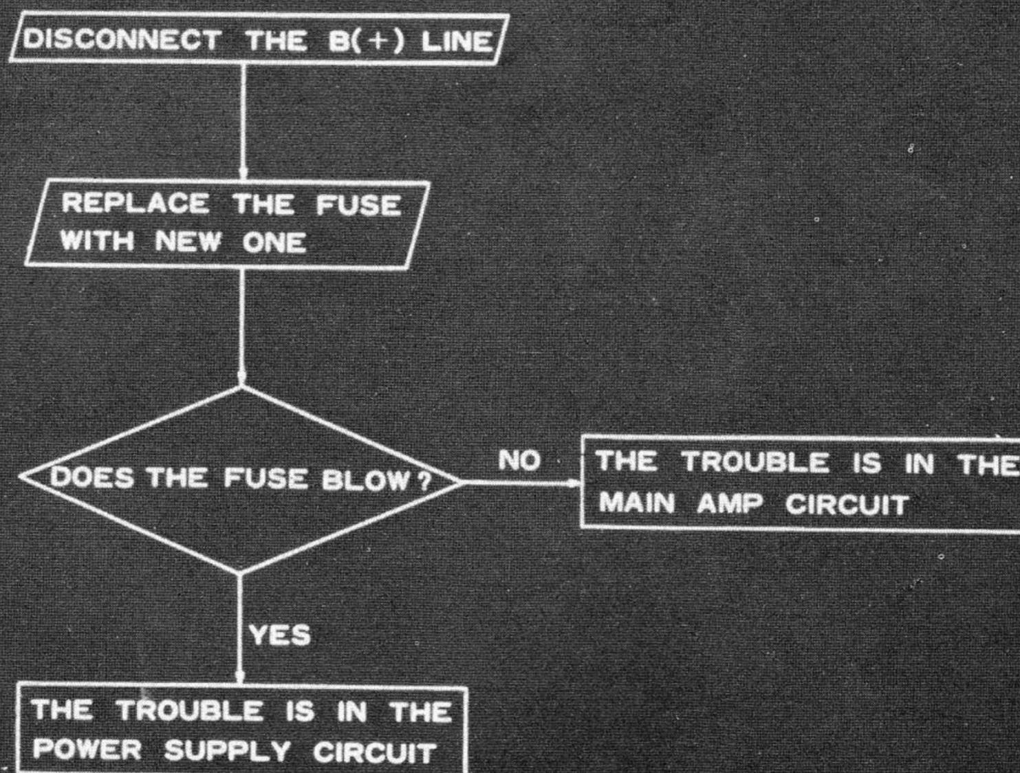
23. DETERMINE IF THE PROBLEM IS IN THE POWER SUPPLY OR THE MAIN AMP CIRCUIT. DISCONNECT THE B(+) LINE, REPLACE THE BLOWN FUSE. DOES THE FUSE BLOW AGAIN? IF "YES", THE PROBLEM IS IN THE POWER SUPPLY. IF "NO", THE PROBLEM IS IN THE MAIN AMP CIRCUIT.
