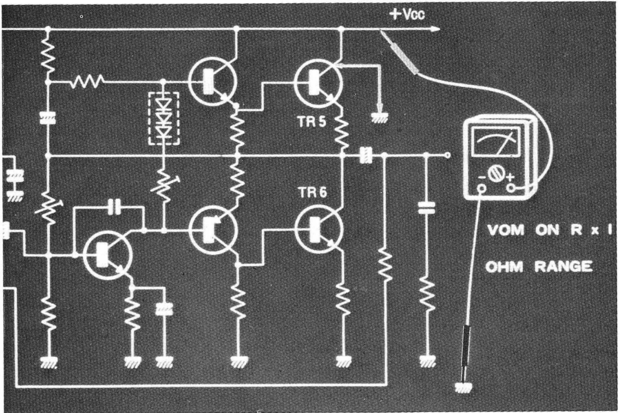
35. NOW WE WILL CONSIDER A CASE WHERE A SHORT OCCURS BETWEEN THE COLLECTOR AND EMITTER IN BOTH TRANSISTORS AT THE SAME TIME. USE YOUR VOM SET ON R<sub>x</sub>1 OHM RANGE AND TAKE A READING.
