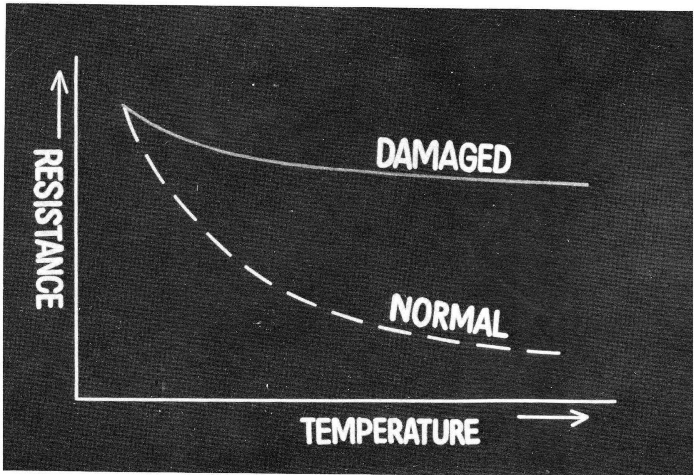
60. IF A DIODE IS DAMAGED, ITS RESISTANCE VALUE WILL NOT CHANGE WITH INCREASED TEMPERATURE. IF IT DOES NOT CHANGE, THEN IT WILL NOT CONTROL THE BIAS ON THE TRANSISTOR, THEREFORE LETTING THE TRANSISTOR HEAT UP AND BLOW THE FUSE.
