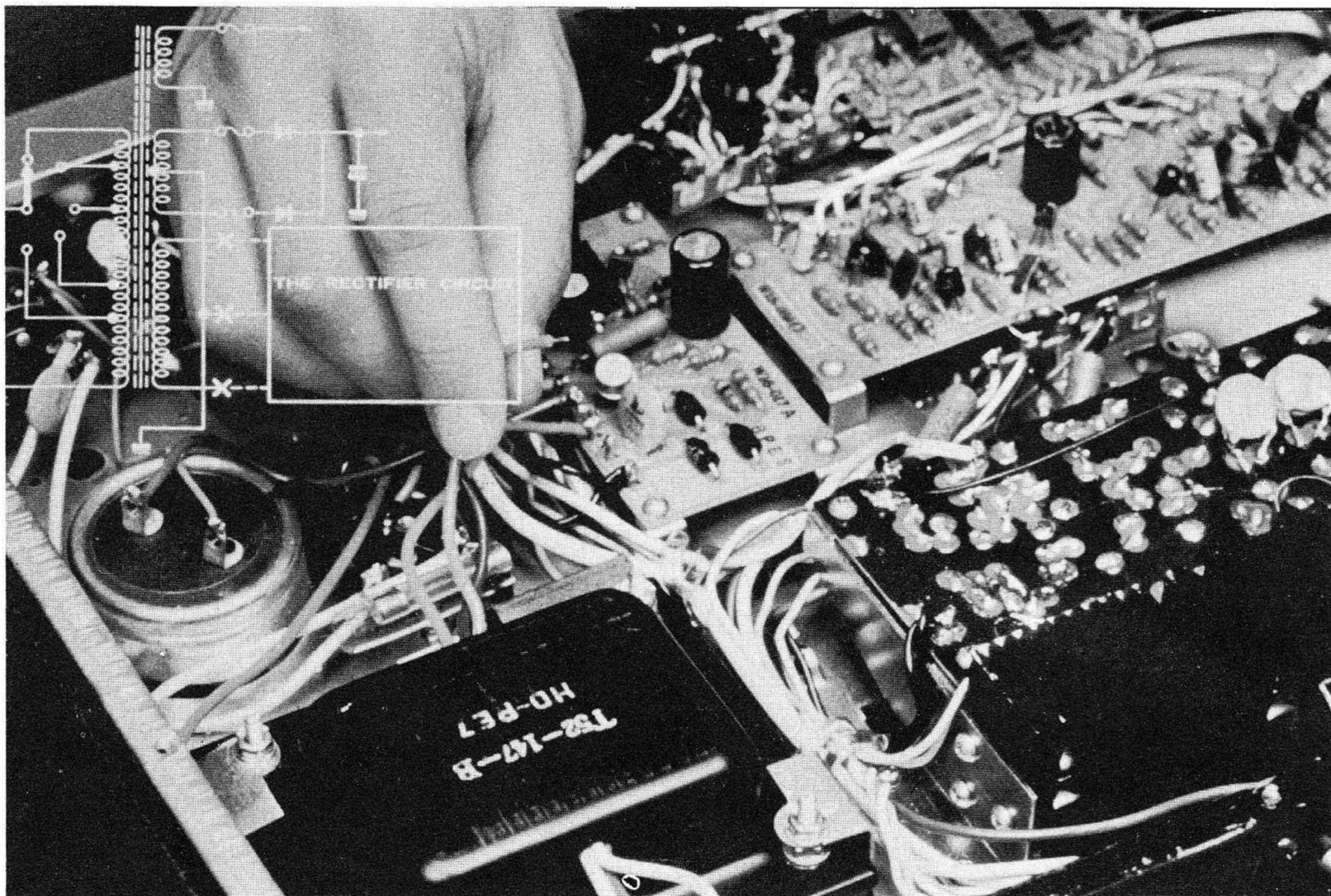
24. TO CHECK THE POWER SUPPLY CIRCUIT, DISCONNECT THE RECTIFIER CIRCUIT FROM THE SECONDARY WINDING OF THE TRANSFORMER. TURN ON THE UNIT WITH A GOOD FUSE INSTALLED. IF THE FUSE BLOWS THE FAILURE IS IN THE TRANSFORMER OR THE NOISE PREVENTION CAPACITOR.
