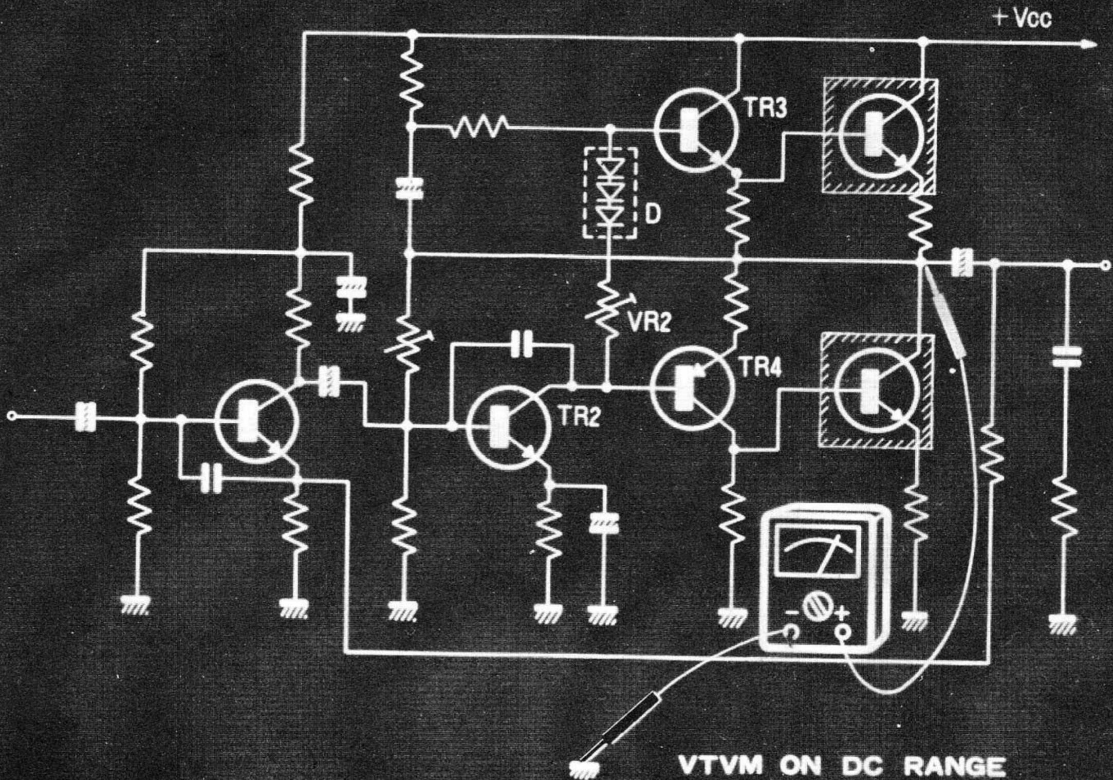
45. IF THE VOLTAGE READING IS HIGHER THAN  $\frac{1}{2}$  VCC, THEN TR-3 IS DEFECTIVE, OR THE TEMPERATURE COMPENSATING ELEMENT OR VR2 IS OPEN.
