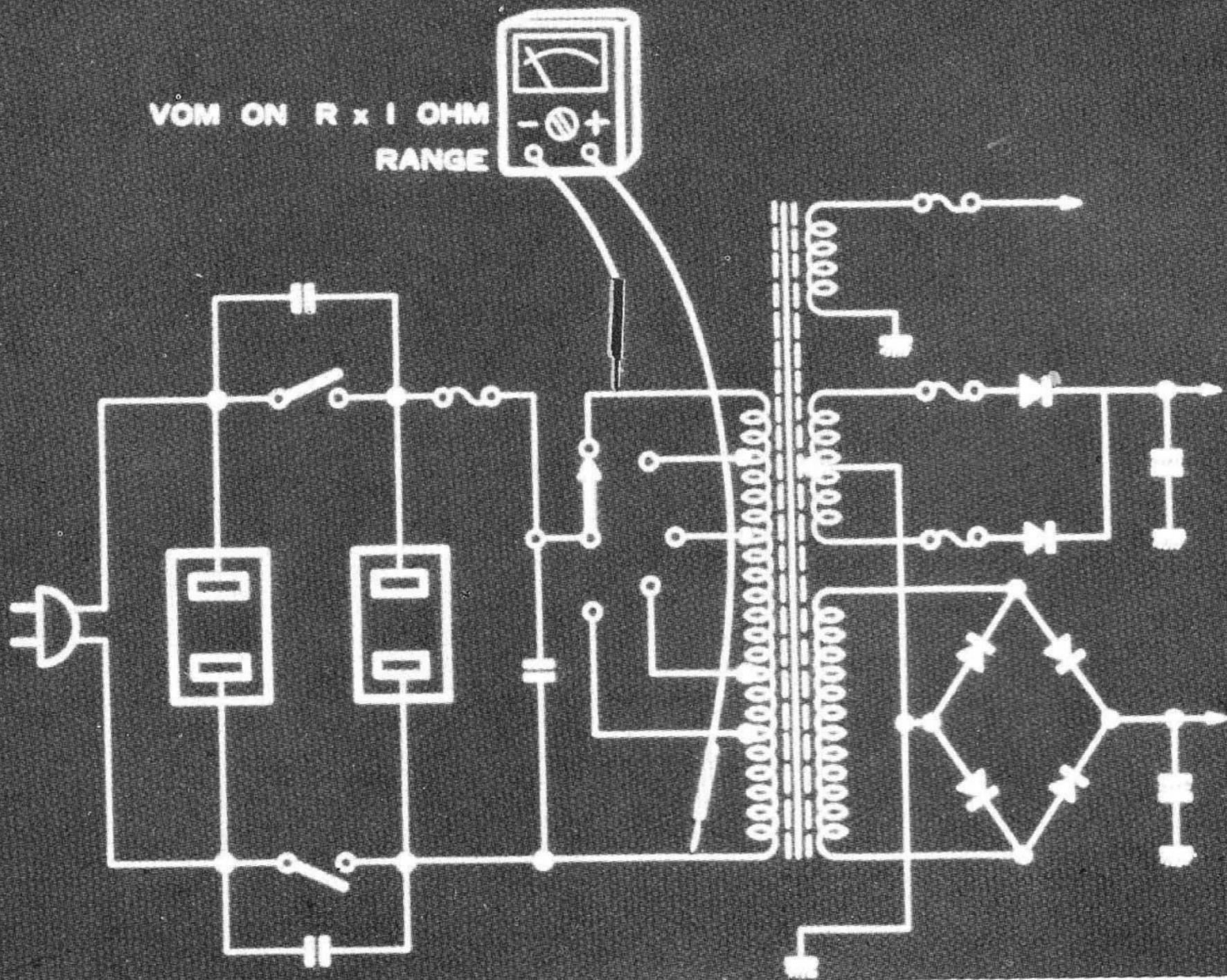
18. TO CHECK THE PRIMARY WINDING, UNPLUG THE MAIN POWER FROM THE WALL, THEN MEASURE THE CONTINUITY ACROSS THE PRIMARY WINDING-USING A VOM ON R<sub>x</sub>1 OHM RANGE. WHENEVER YOU CHECK THE CONTINUITIES, PLEASE BE SURE TO UNPLUG THE AC CORD FROM THE WALL. YOU SHOULD GET A READING OF APPROXIMATELY 30-300 OHMS. IF THE READING IS INFINITY THEN THE PRIMARY WINDING IS OPEN.
