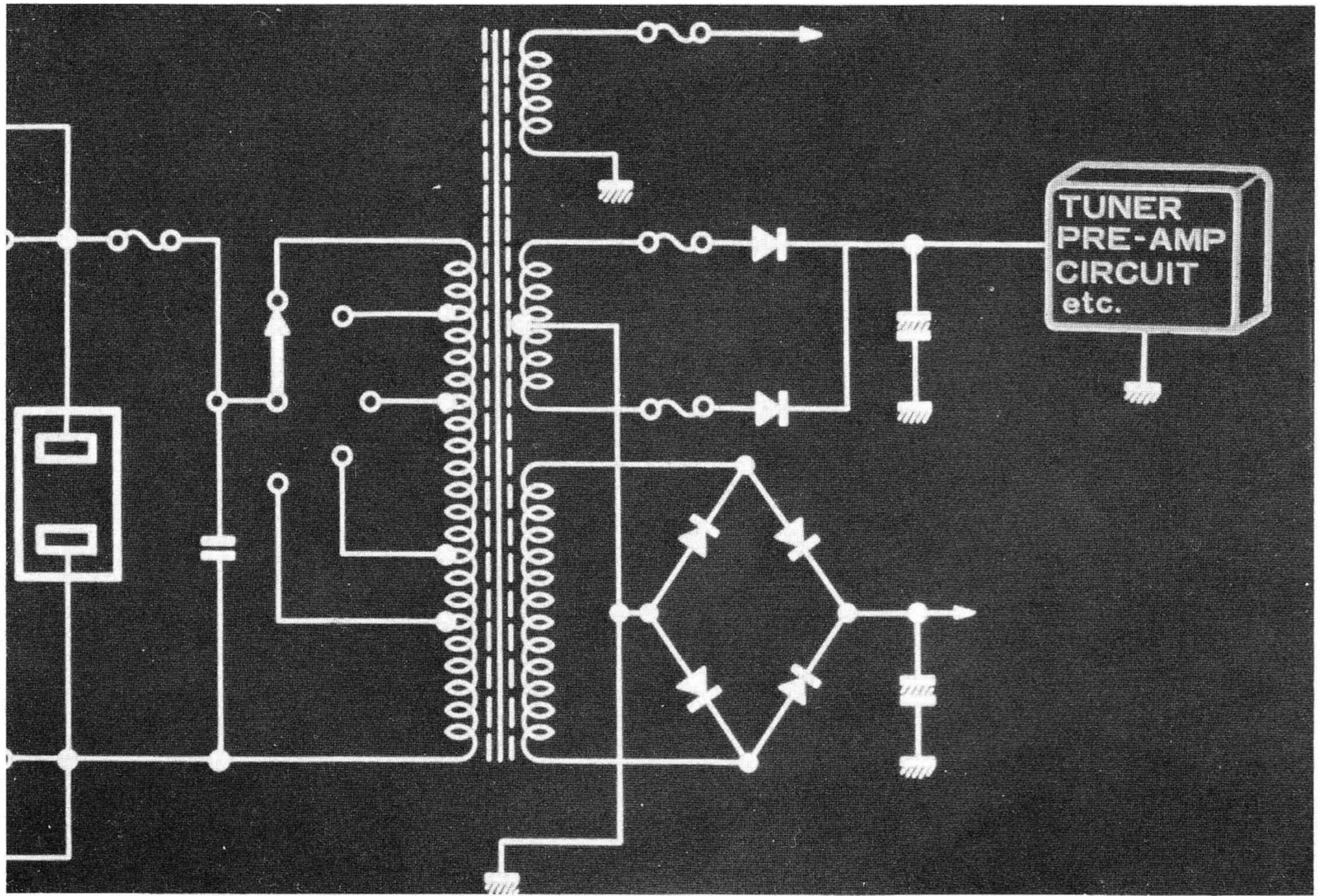
50. THIS OVERCURRENT MAY BE CAUSED BY A SHORTED SECONDARY, A DEFECTIVE DIODE, OR A SHORTED FILTER CAPACITOR.
