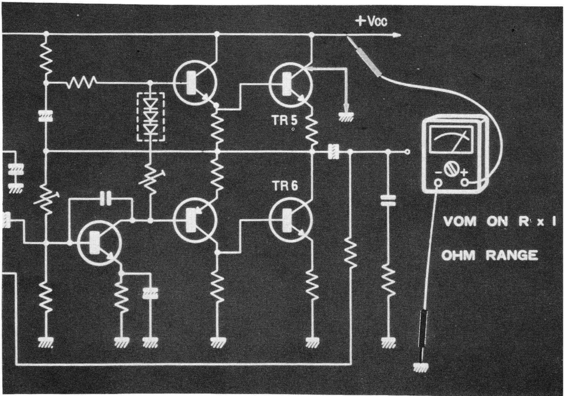
31. TO LOCATE THE PROBLEM, MEASURE THE RESISTANCE FROM VCC TO GROUND. YOUR VOM SHOULD BE SET ON R<sub>x</sub>1 OHM RANGE. ZERO RESISTANCE INDICATES A SHORT TO THE HEAT SINK OF TR5. IN THIS MEASUREMENT, THE POWER SUPPLY CIRCUIT SHOULD BE DISCONNECTED WITH THE MAIN AMP CIRCUIT.
