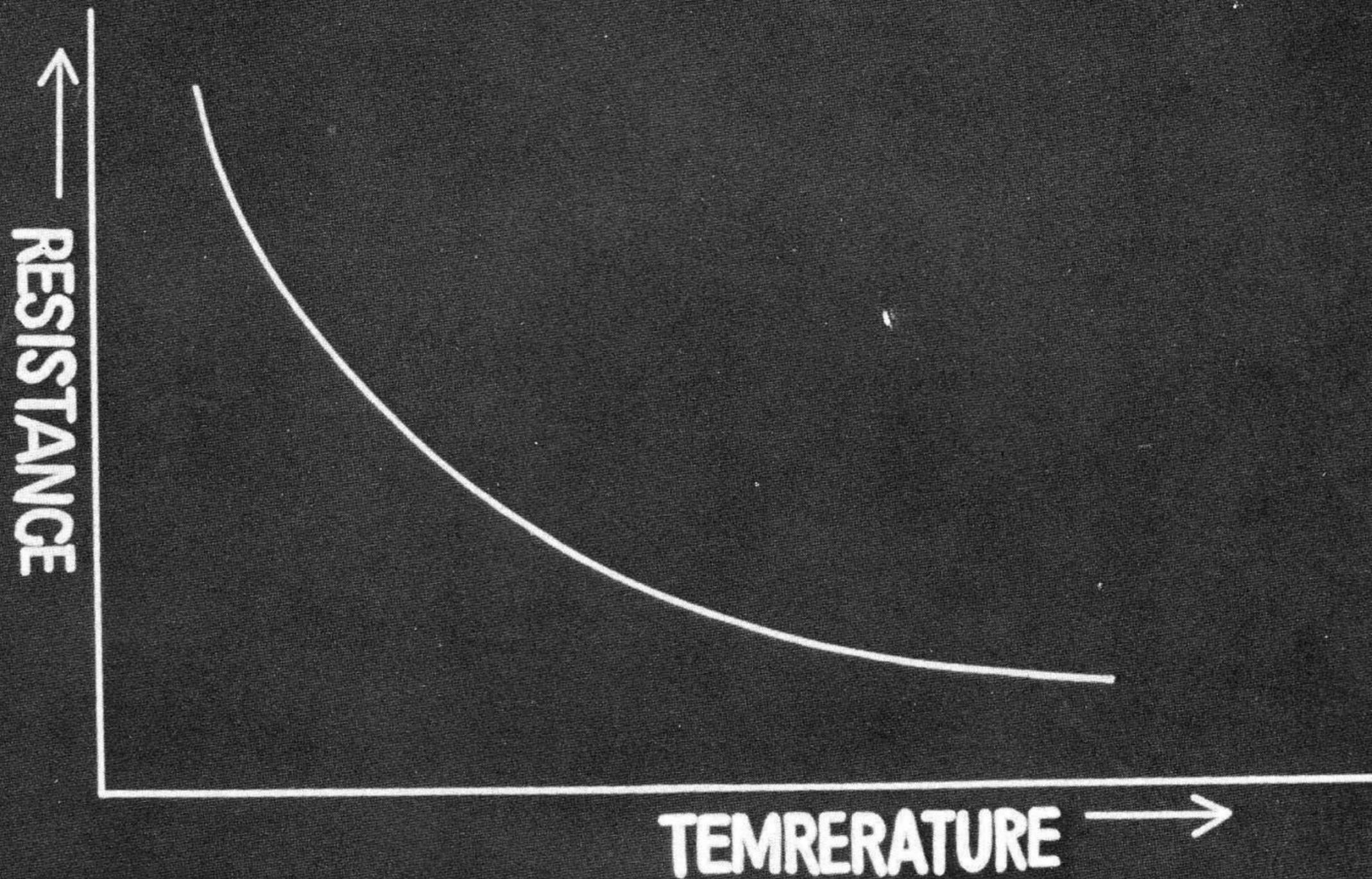
59. A GOOD TEMPERATURE COMPENSATING DIODE DECREASES RESISTANCE WITH INCREASING TEMPERATURE AND THEREFORE COMPENSATE THE BIAS OF THE TRANSISTORS IT IS CONNECTED TO.
