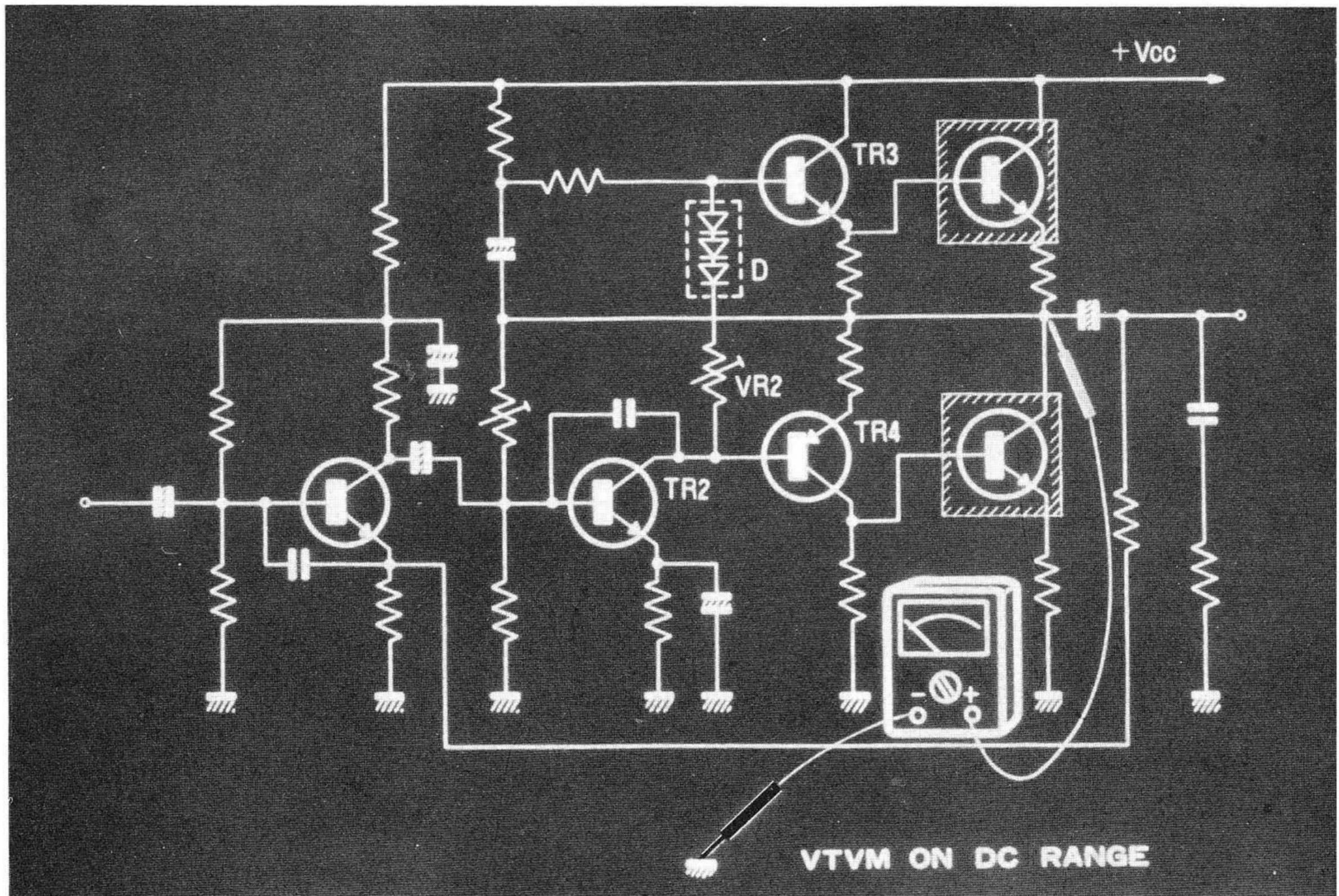
43. IF YOU DO NOT HEAR BUZZING THEN MEASURE THE CENTER VOLTAGE. IF IT READS EXACTLY  $\frac{1}{2}$  OF VCC THEN THE CIRCUIT IS WORKING NORMAL. YOU CAN SUSPECT THAT EITHER ONE OF THE POWER TRANSISTORS YOU JUST REMOVED IS DEFECTIVE.
