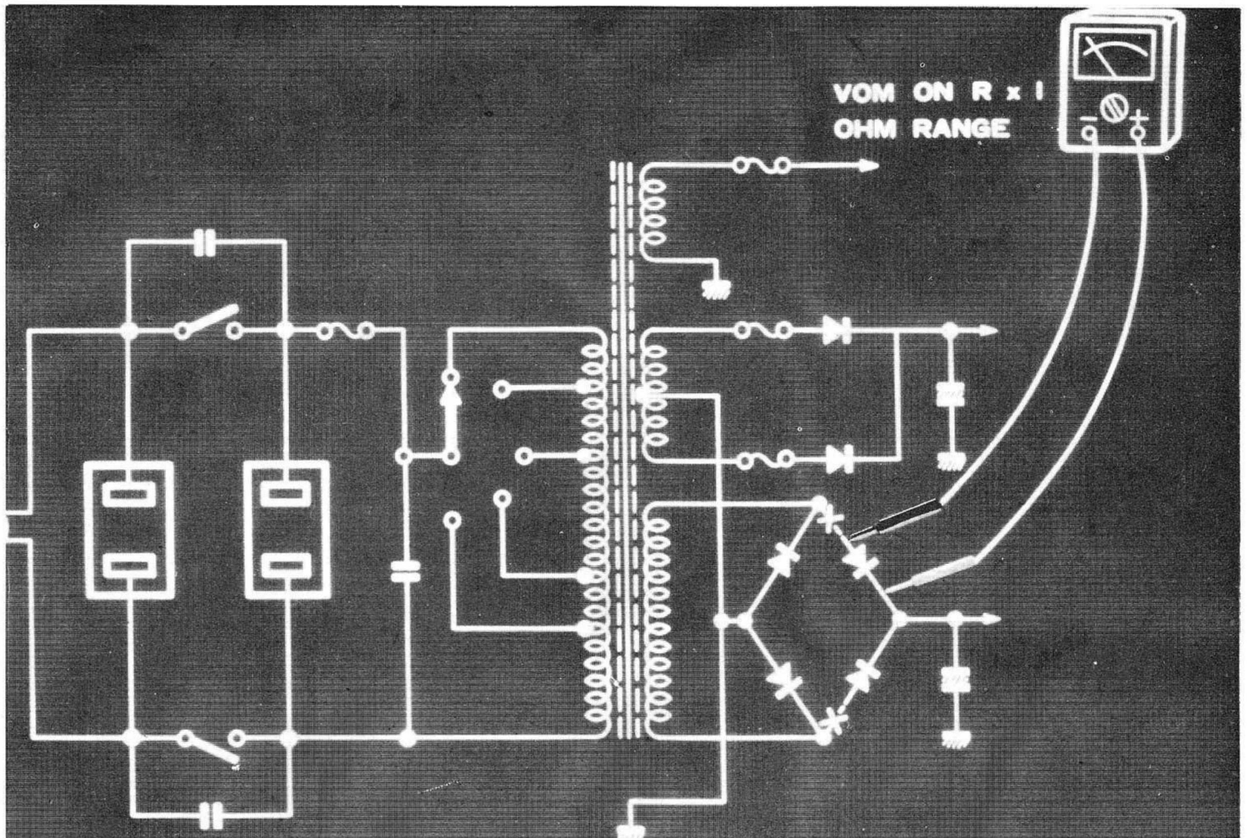
25. IF THE FUSE DID NOT BLOW IN THE PREVIOUS CHECK, THEN YOUR NEXT STEP IS TO CHECK THE DIODES IN THE RECTIFIER CIRCUIT FOR SHORTS.
