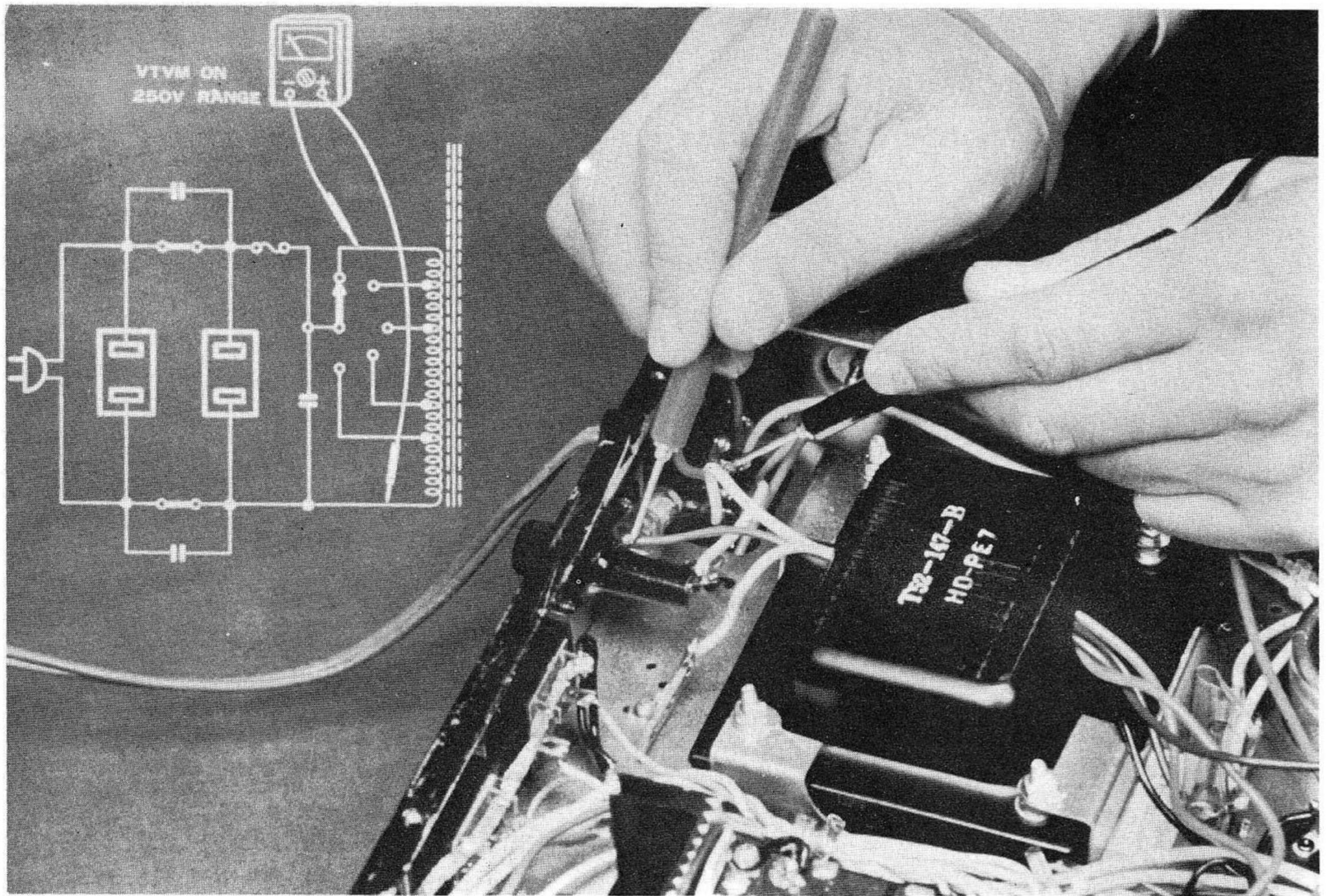
16. IF YOU DO NOT GET A READING, THEN THE FUSE HOLDER OR POWER SWITCH IS DEFECTIVE. IF YOU READ THE PROPER VOLTAGE, THEN THE PRIMARY WINDING OF THE POWER TRANSFORMER MUST BE OPEN.
