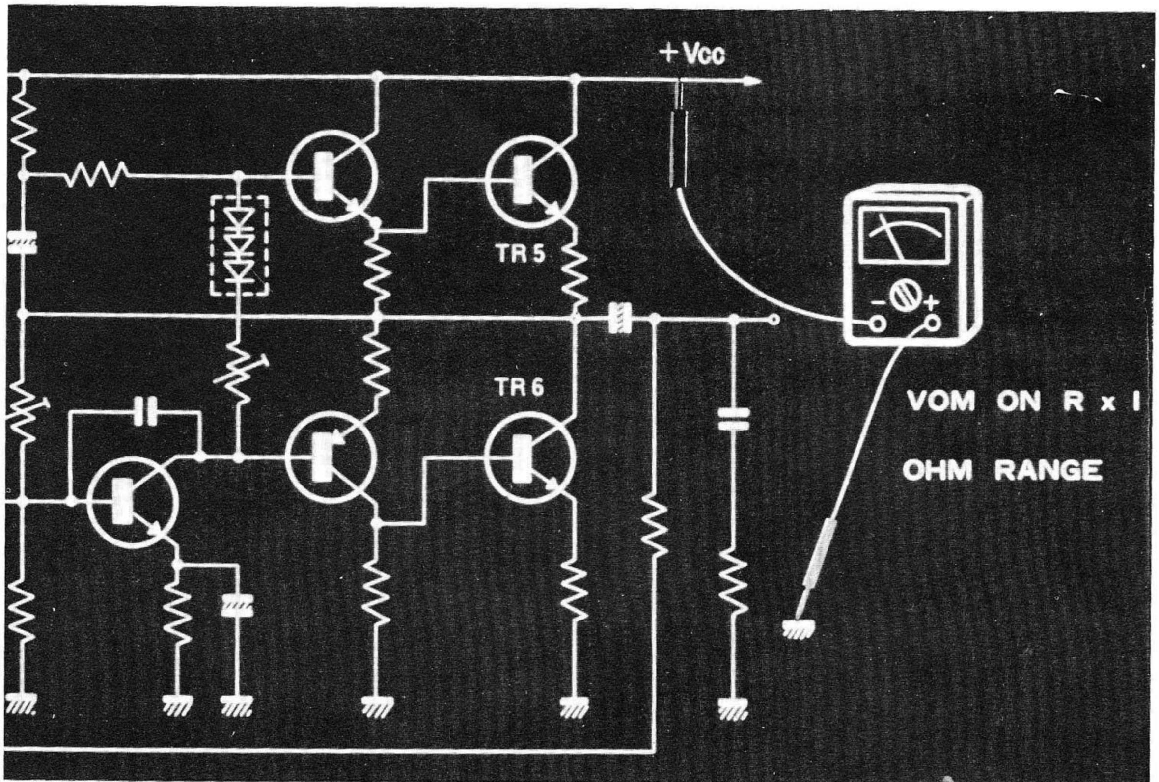
36. NOW REVERSE THE POLARITY OF THE TEST LEADS AND TAKE ANOTHER READING. IF THIS READING IS EQUAL TO THE SUM OF BOTH EMITTER RESISTORS THEN BOTH TRANSISTORS ARE SHORT-ED.
