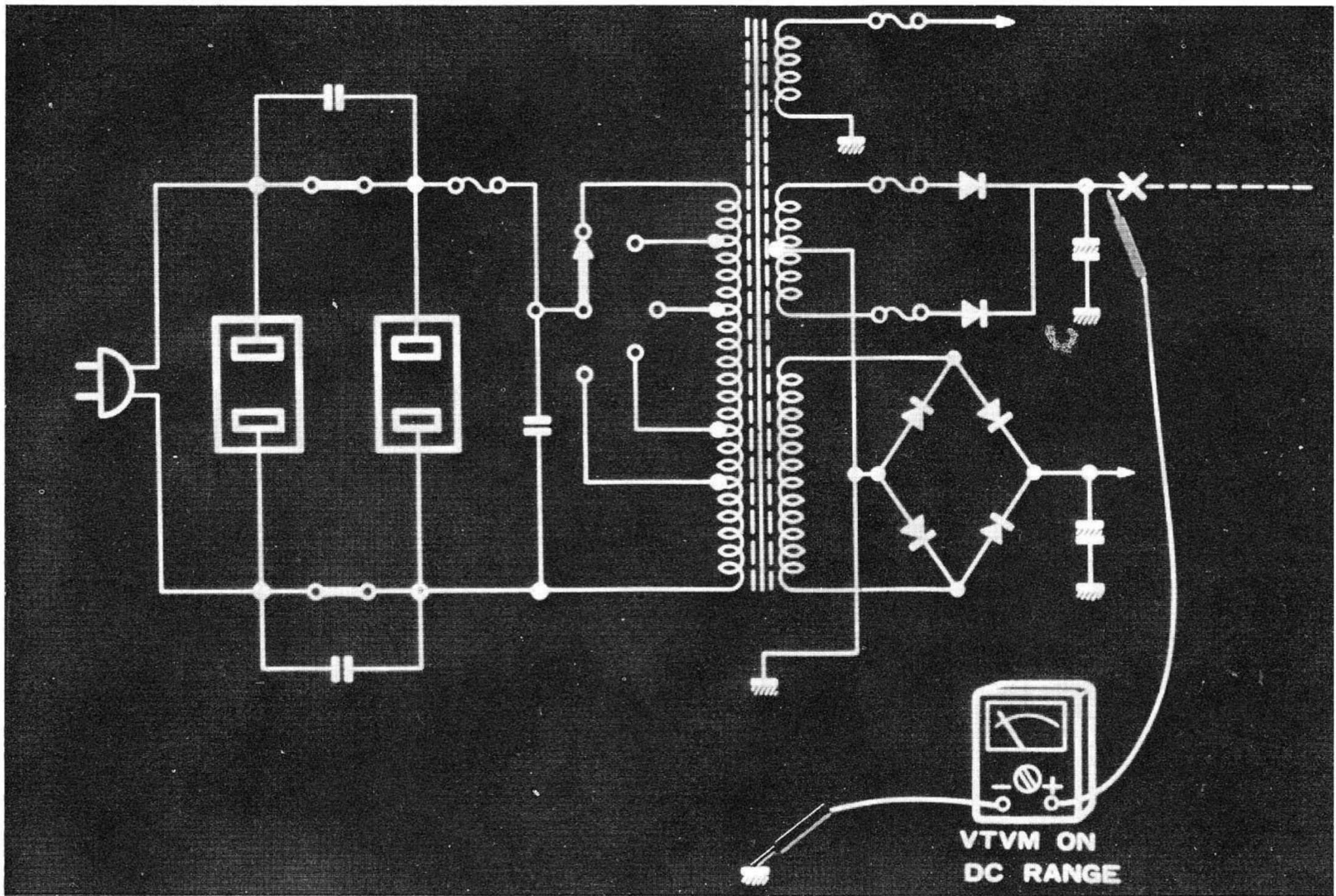
51. TO DETERMINE IF THE PROBLEM IS IN THE RECTIFIER SIDE OR THE LOAD SIDE OF THE POWER SUPPLY, REMOVE THE B(+) LINE WHICH IS CONNECTING THE LOAD TO THE POWER SUPPLY. USING YOUR VTVM ON THE 100V D.C. RANGE TAKE A READING OF THE POWER SUPPLY OUTPUT VOLTAGE. IF THE READING IS NORMAL THEN THE PROBLEM IS IN THE LOAD SIDE AND IF NOT THE PROBLEM LIES IN THE POWER SUPPLY.
