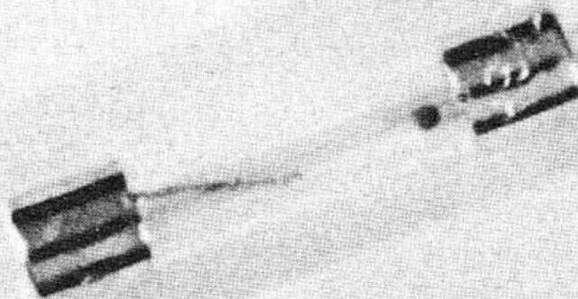
**THE FUSE BLOWS AFTER THE UNIT IS ON FOR A SHORT TIME**
