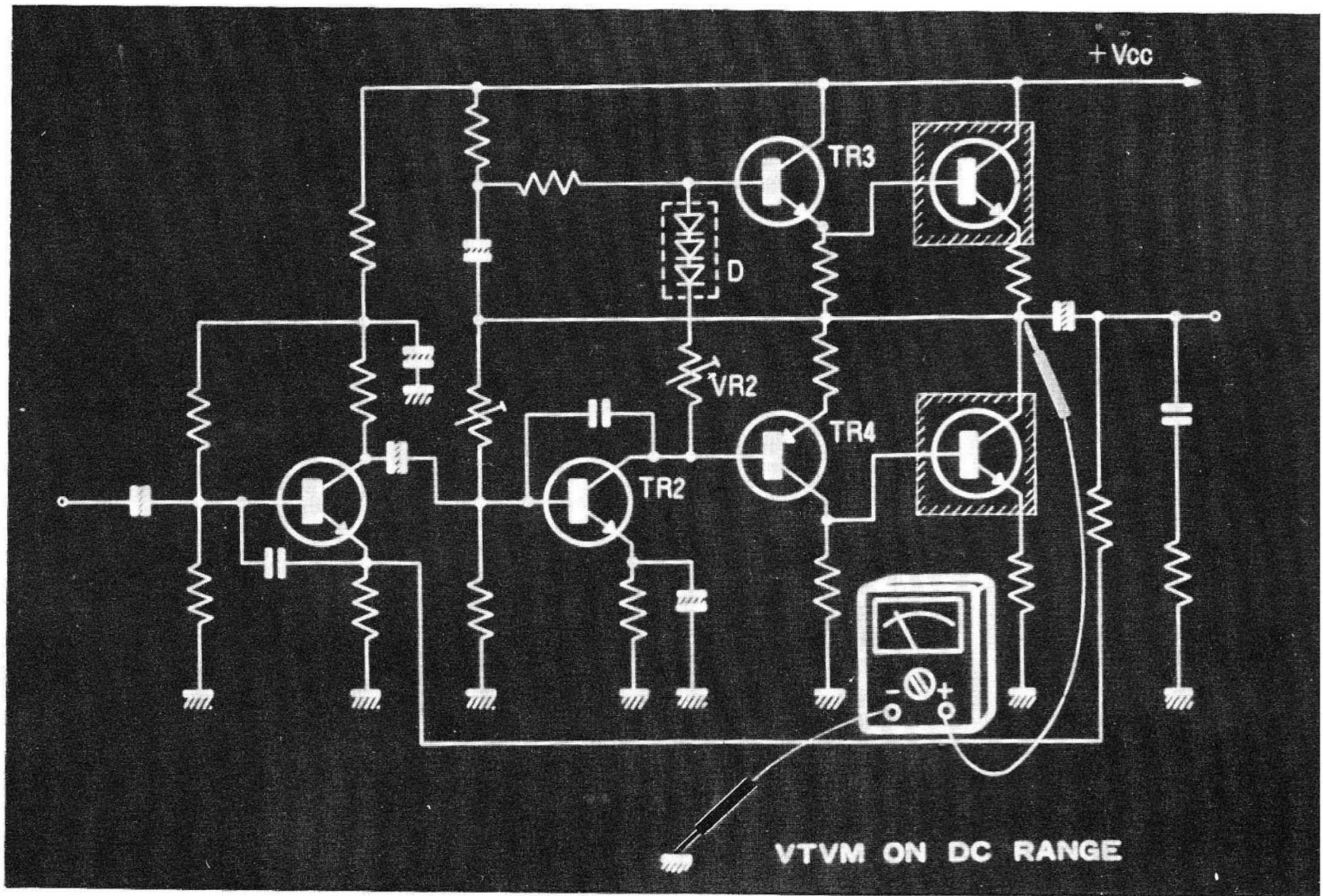
44. IF YOU DO HEAR BUZZING, THEN EXCESSIVE CURRENT MUST BE FLOWING THROUGH THE DRIVER STAGE.
