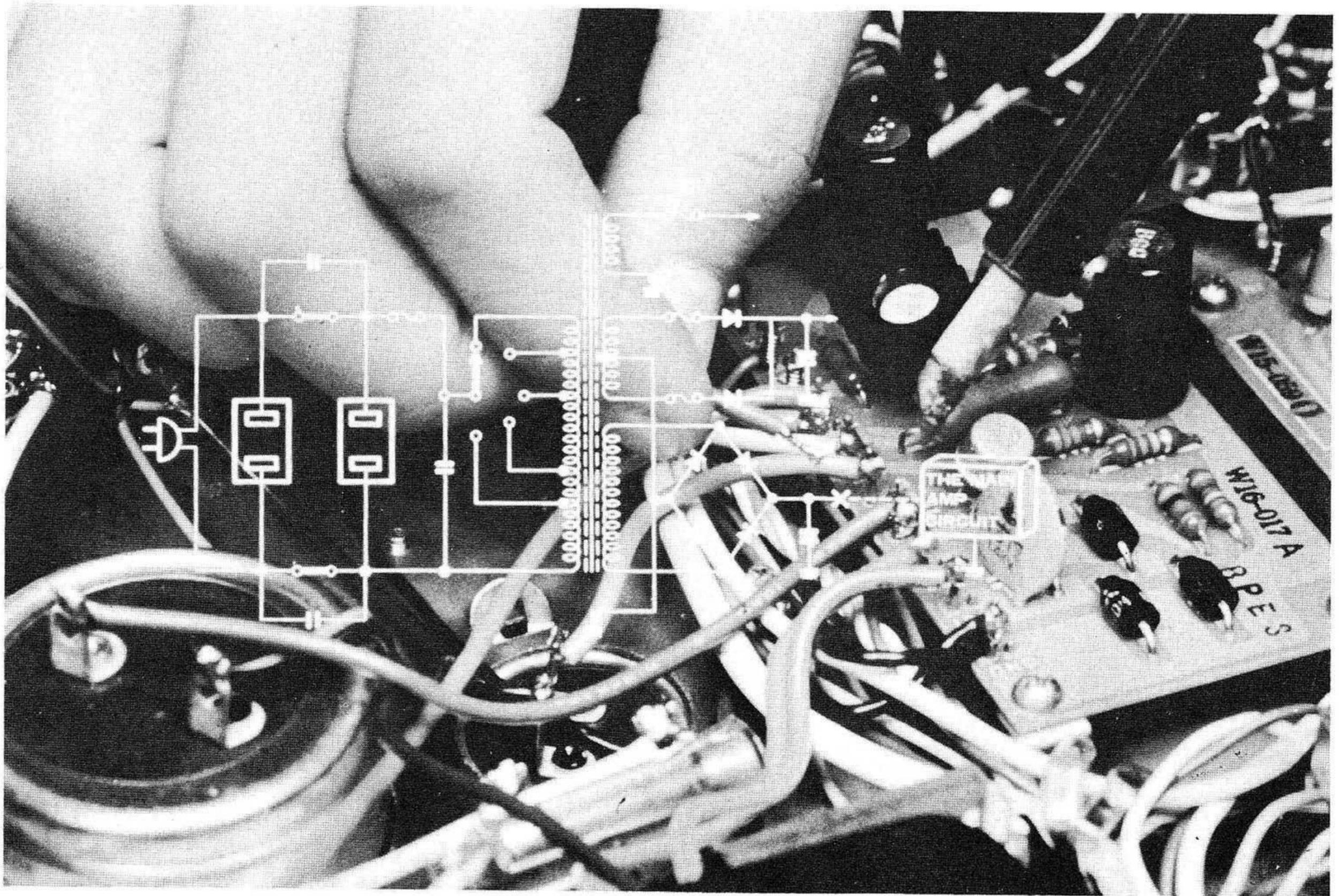
21. TO DETERMINE IF THE PROBLEM IS IN THE POWER SUPPLY OR THE MAIN AMP CIRCUIT, DISCONNECT THE B(+) LINE TO THE MAIN AMP.
