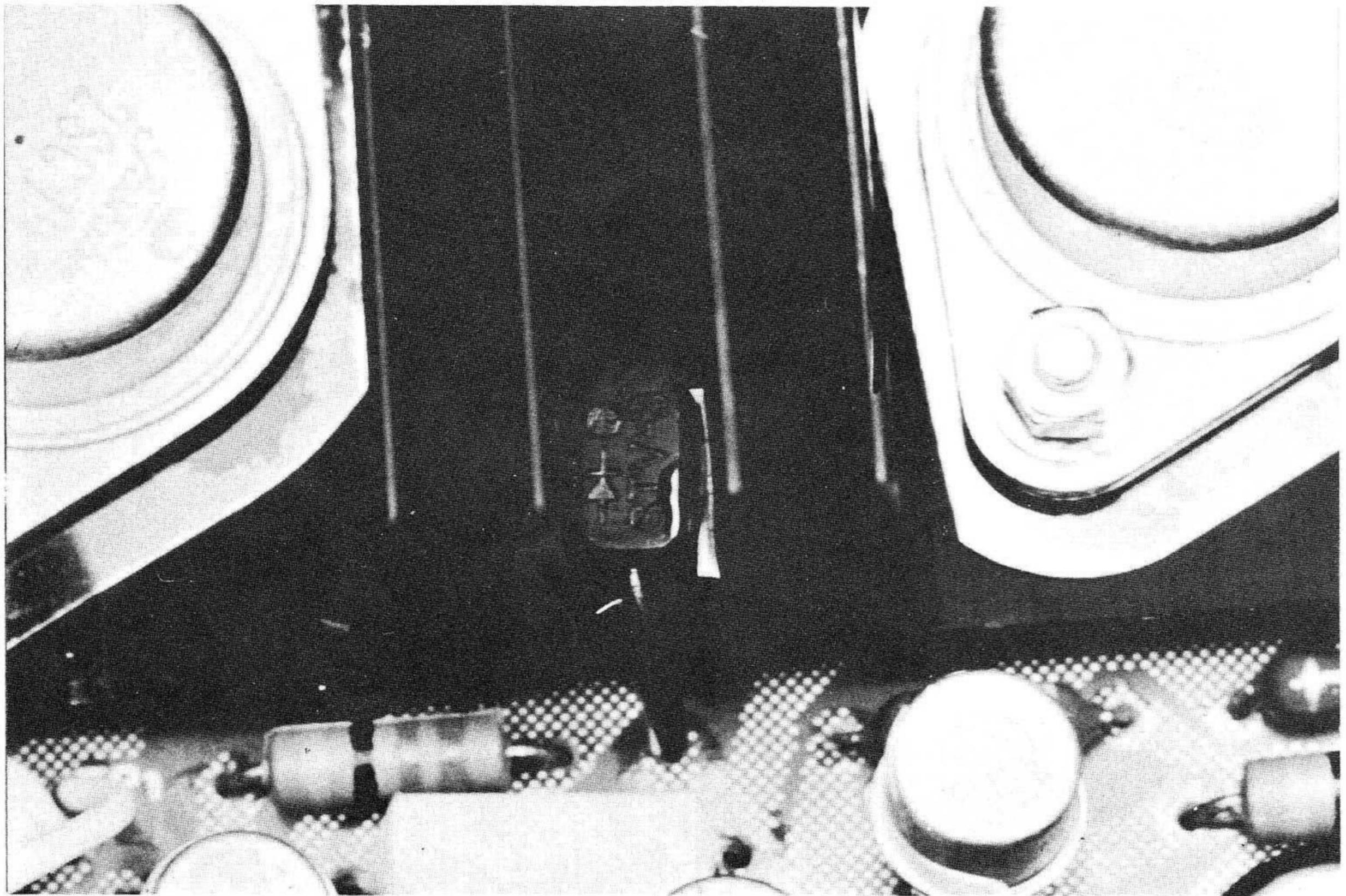
58. HERE YOU WILL SUSPECT THE TEMPERATURE COMPENSATING DIODES ARE DEFECTIVE. THEY SHOULD CHANGE VALUE ACCORDING TO THE TEMPERATURE BUT DEFECTIVE ONES WILL NOT.
