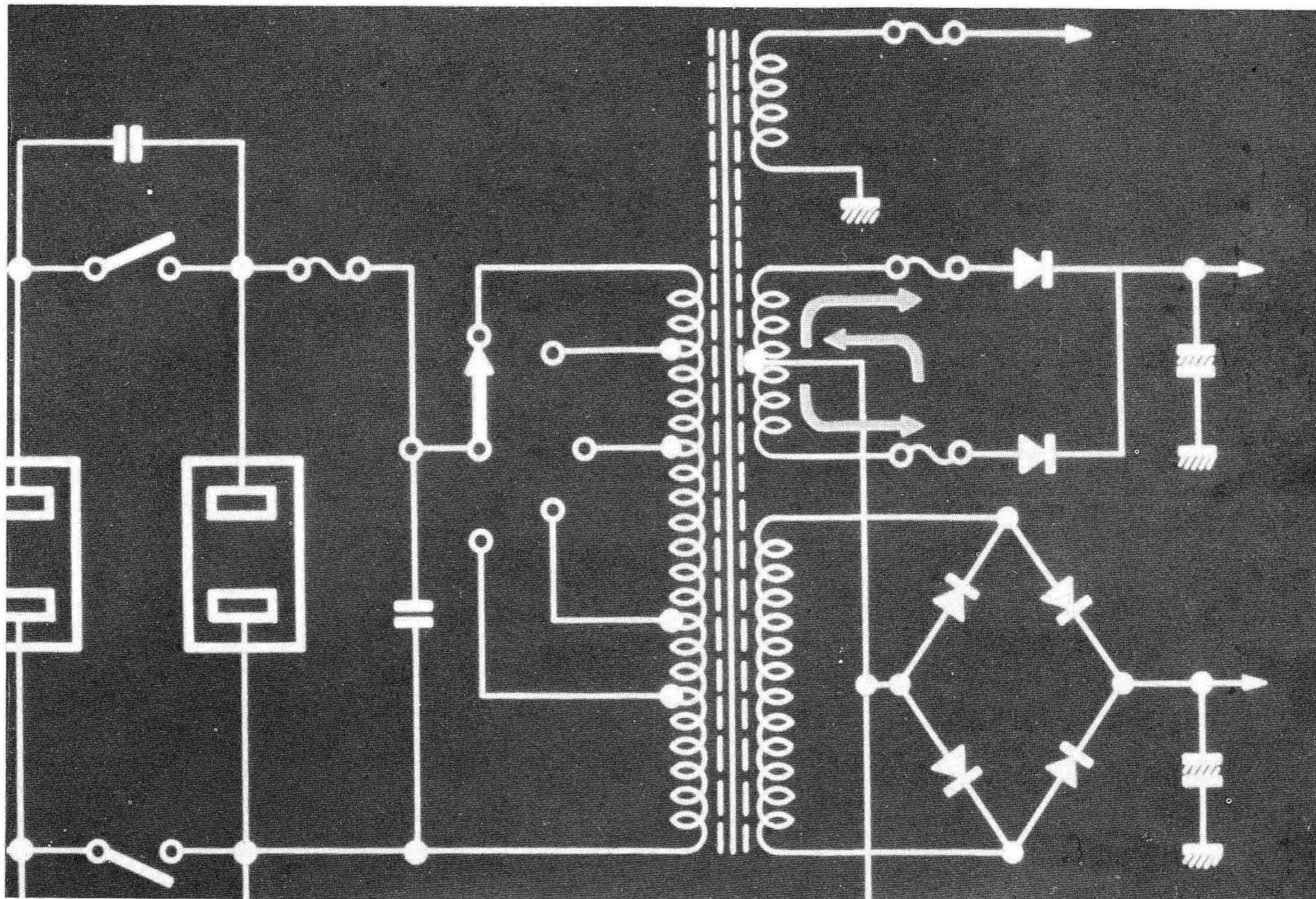
49. HERE AGAIN THE PROBLEM MAY BE IN THE POWER SUPPLY. THE SECONDARY SIDE OF THE POWER TRANSFORMER MAY BE OVER-LOADED.
