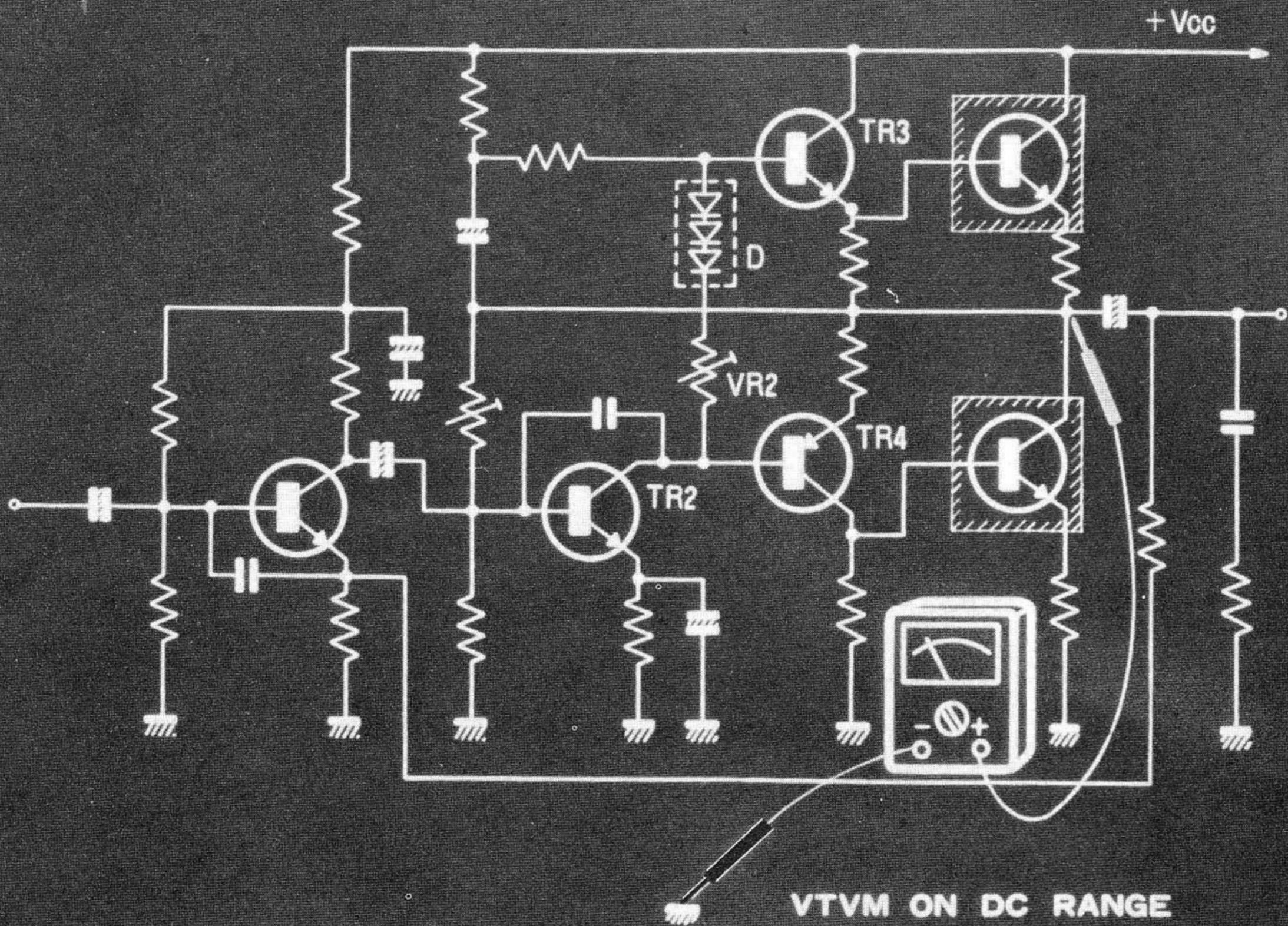
46. A VOLTAGE READING LOWER THAN  $\frac{1}{2}$  VCC INDICATES A FAILURE OF TR-2 OR TR-4.
