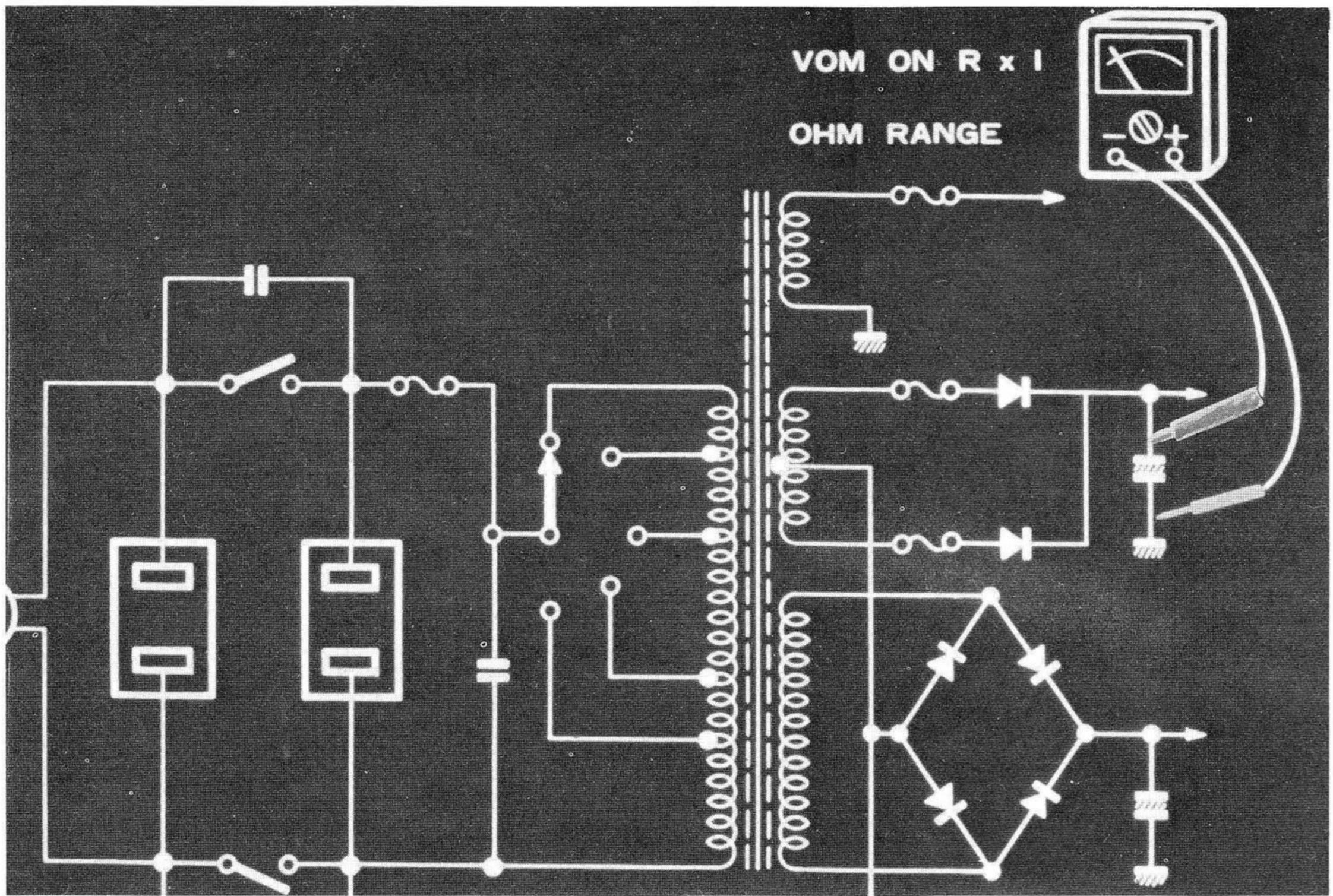
56. IF THEY CHECK OK, THEN TEST THE FILTER CAPACITORS BY PLACING YOUR VOM ON THE R<sub>x</sub>1 OHM RANGE, AND PLACE THE TEST LEADS ACROSS THE CAPACITOR. IF THE CAPACITOR IS GOOD, YOUR METER WILL SWING FROM INFINITY TO ZERO AND SLOWLY RETURNS TO INFINITY AGAIN. IF THE CAPACITOR IS SHORTED, IT WILL READ CONSTANT ZERO OR VERY SMALL RESISTANCE.
