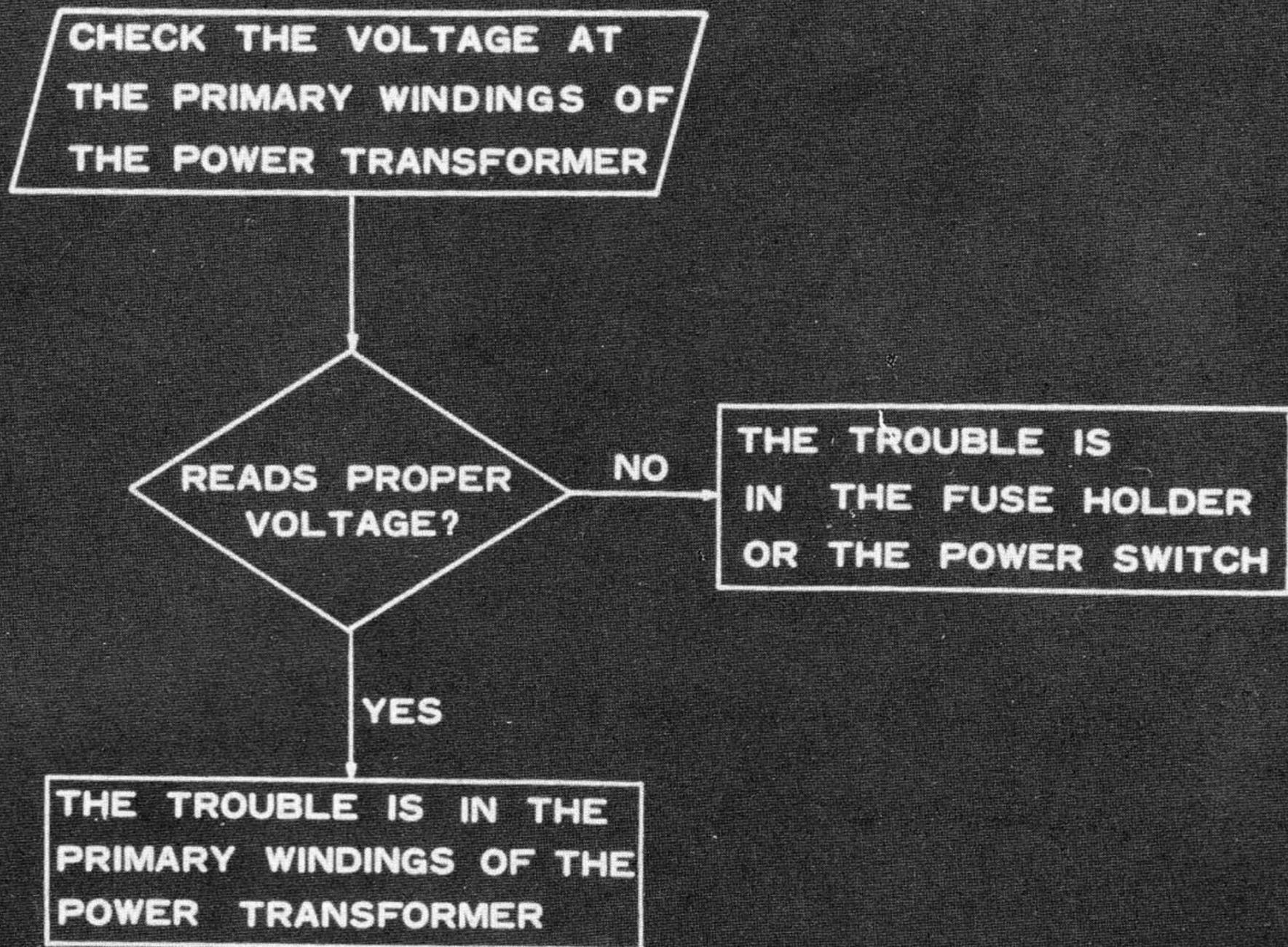
17. CHECK THE VOLTAGE AT THE PRIMARY WINDING OF THE TRANSFORMER. IF IT READS THE PROPER VOLTAGE THEN THE PRIMARY WINDING IS DEFECTIVE. IF IT DOES NOT READ PROPERLY THEN THE FUSE HOLDER OR THE POWER SWITCH IS DEFECTIVE.
