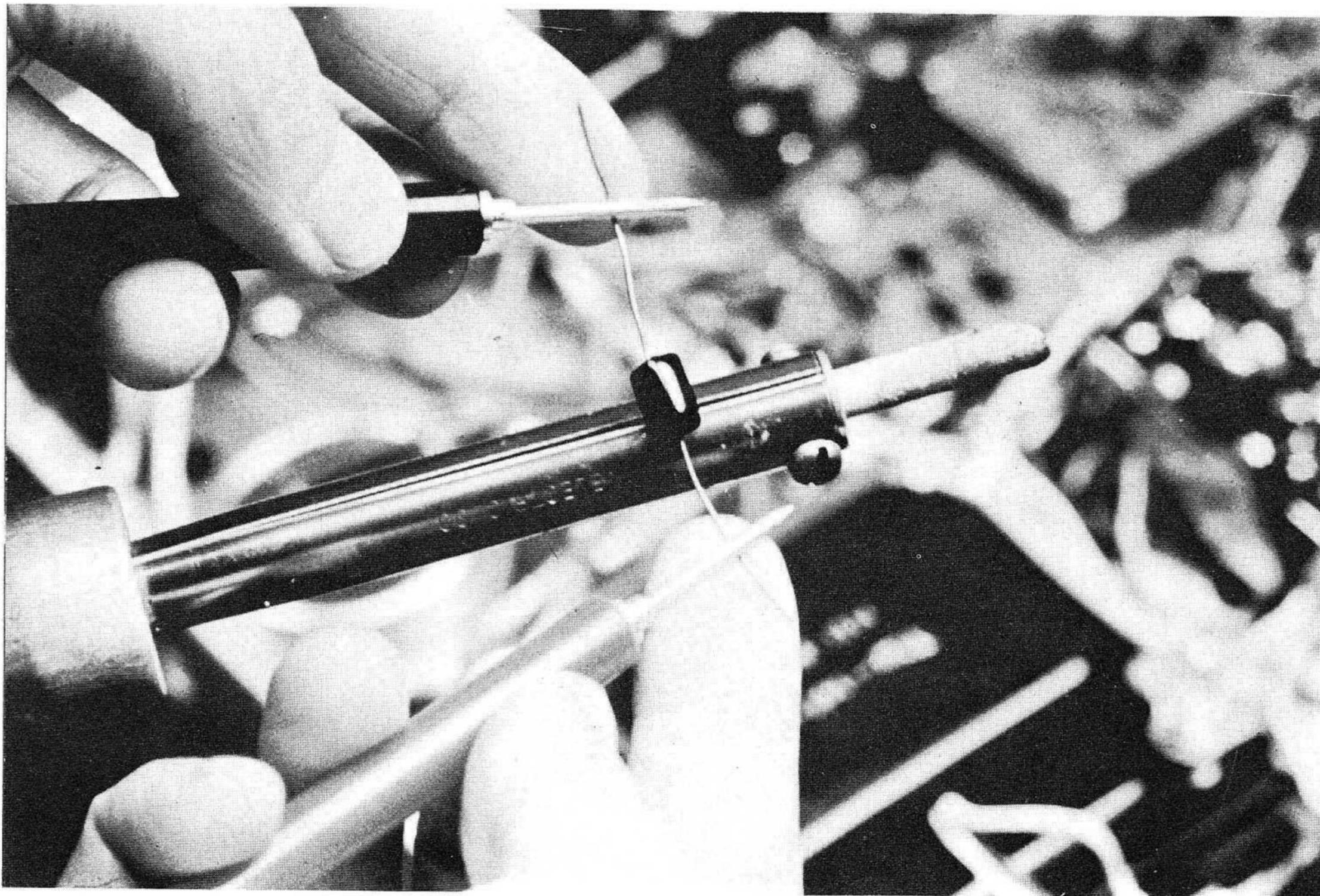
61. TO CHECK THESE DIODES JUST USE YOUR VOM ON THE  $R \times 1$  OHM RANGE. CHECK THE RESISTANCE IN A FORWARD BIAS DIRECTION WHILE YOU HEAT THE DIODE WITH YOUR FINGER OR SOLDERING IRON. IF THE RESISTANCE DECREASES AS THE TEMPERATURE RISES THEN THE DIODE IS GOOD. IF THE RESISTANCE DOES NOT CHANGE, IT IS DEFECTIVE.
