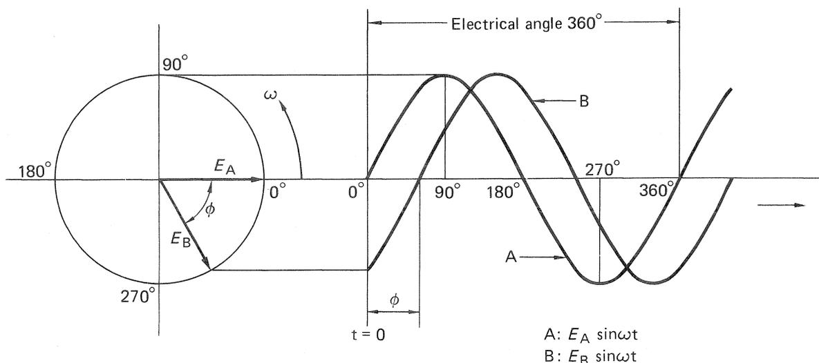
Fig. 6 Phase difference between two sine waves E1
