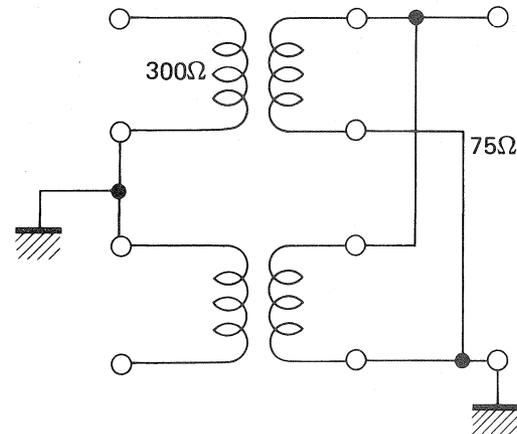
(b) An equivalent circuit of a balun transformer
