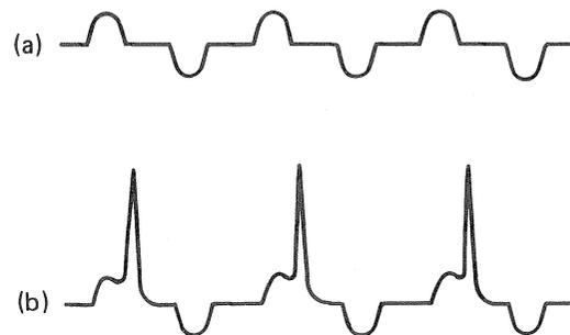
Fig. 14 Current waveforms in the primary winding
