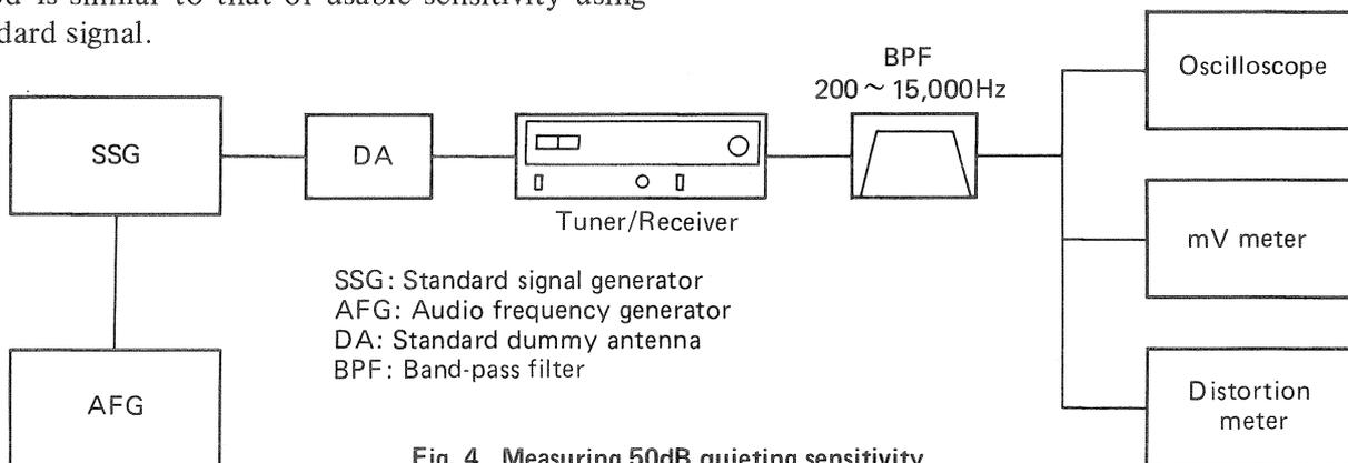
Fig. 4 Measuring 50dB quieting sensitivity
