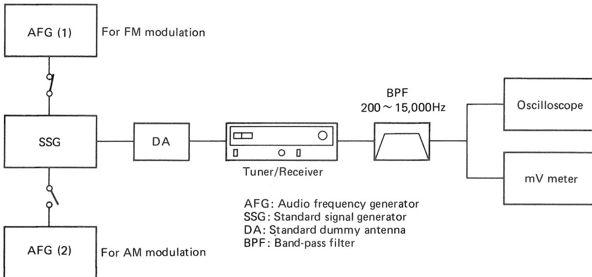
Fig. 12 Measuring AM suppression ratio
