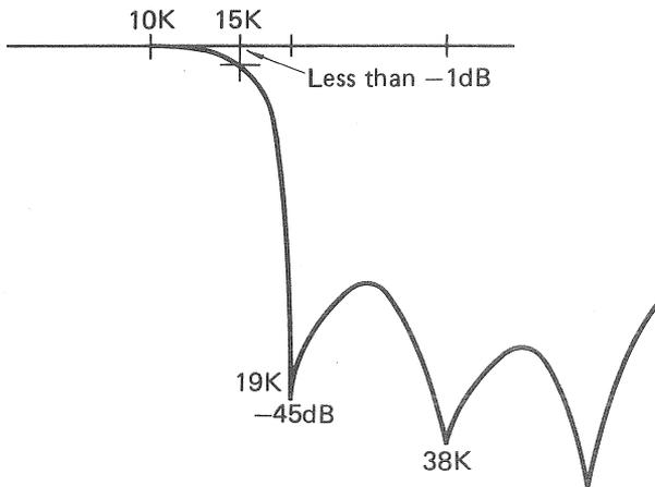
Fig. 20 Three-pole low-pass filter
