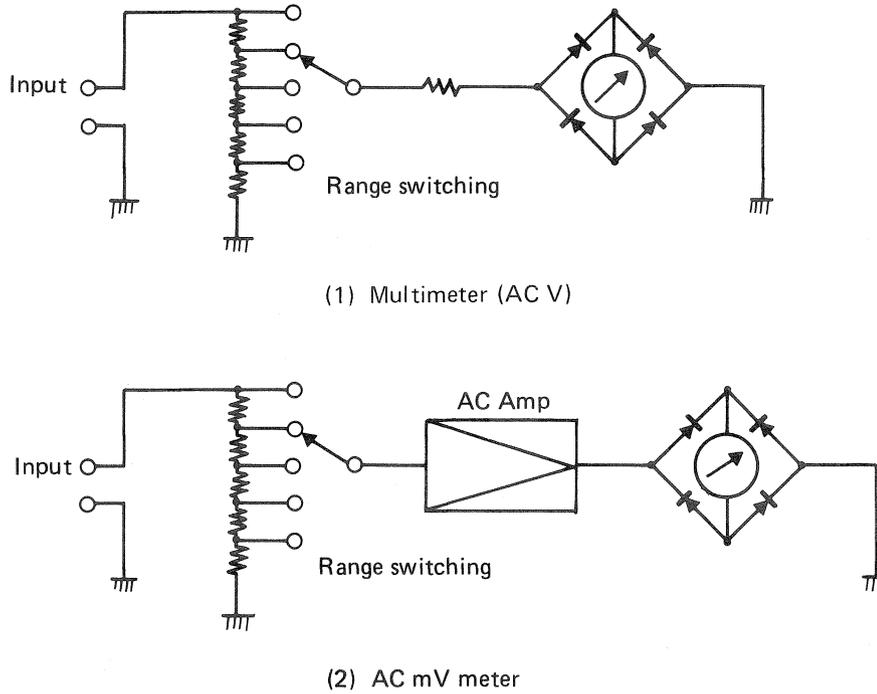
Fig. 1 Basic multimeter and mV meter circuit composition
