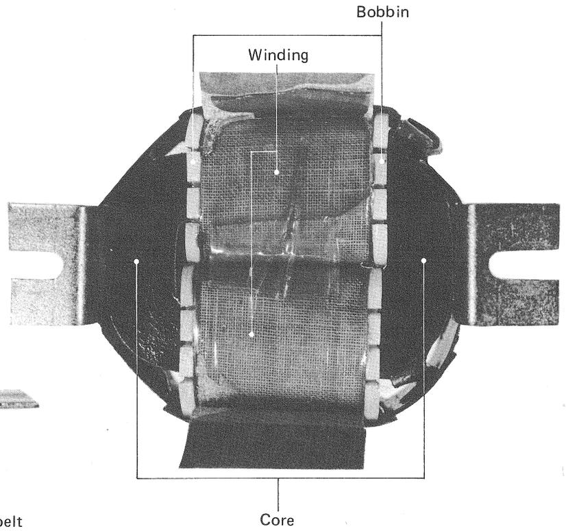
Photo 6 Cut core bottom view
