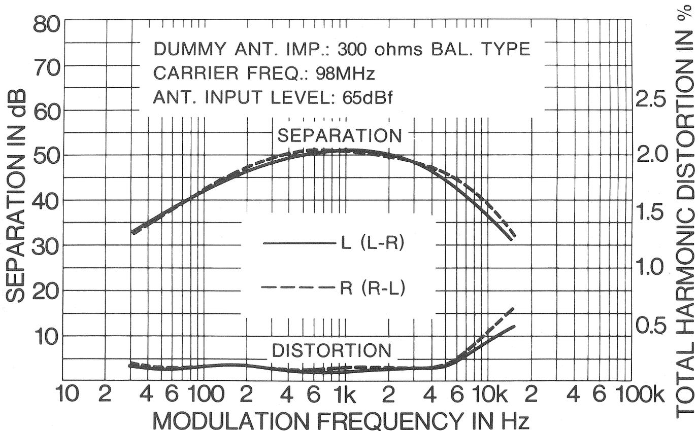
Fig. 14 FM stereo separation and distortion
