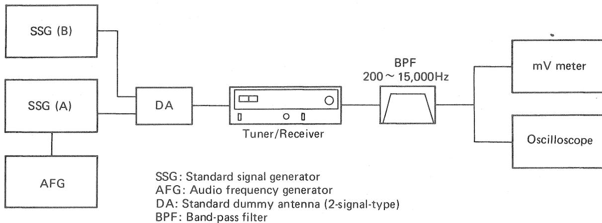
Fig. 11 Measuring spurious response ratio, image response ratio and IF response ratio
