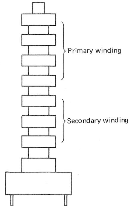
Fig. 17 Detection transformer
