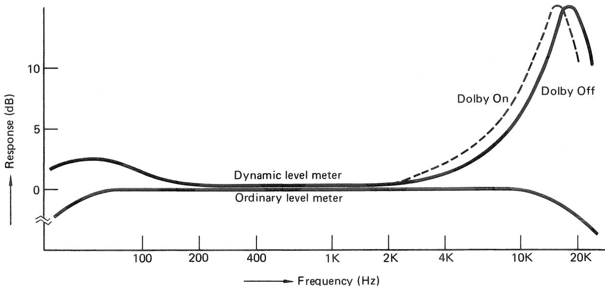
Fig. 4 Frequency characteristics of meter circuit
