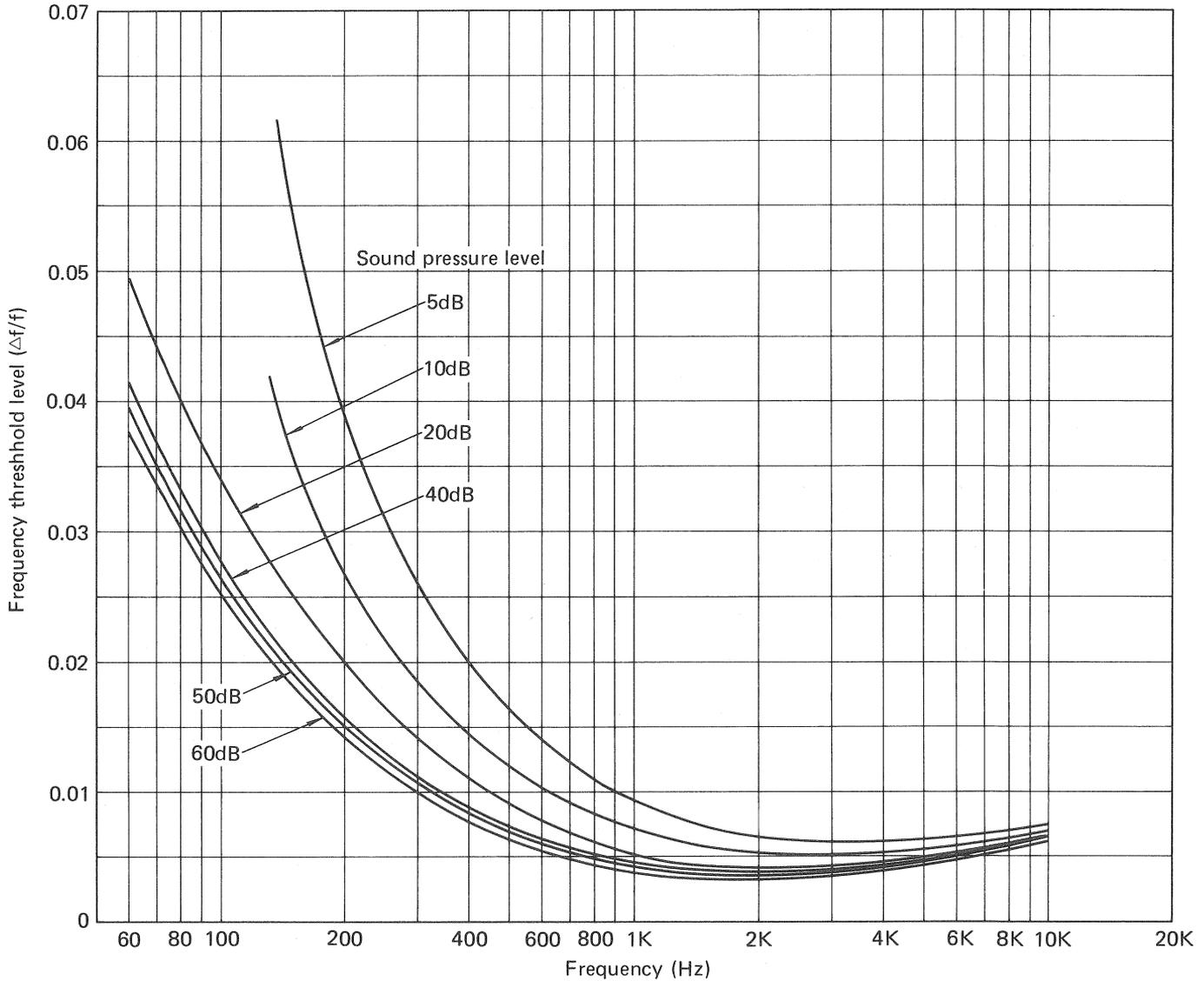
Fig. 2 Frequency threshold level of pure sounds
