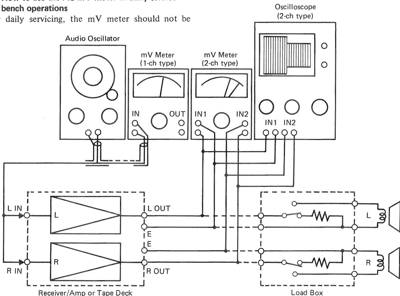
Fig. 5 Connections of mV meter and common measuring instruments
