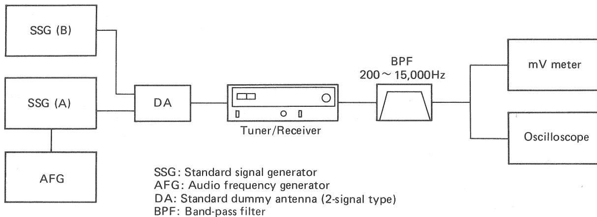
Fig. 9 Measuring alternate channel selectivity
