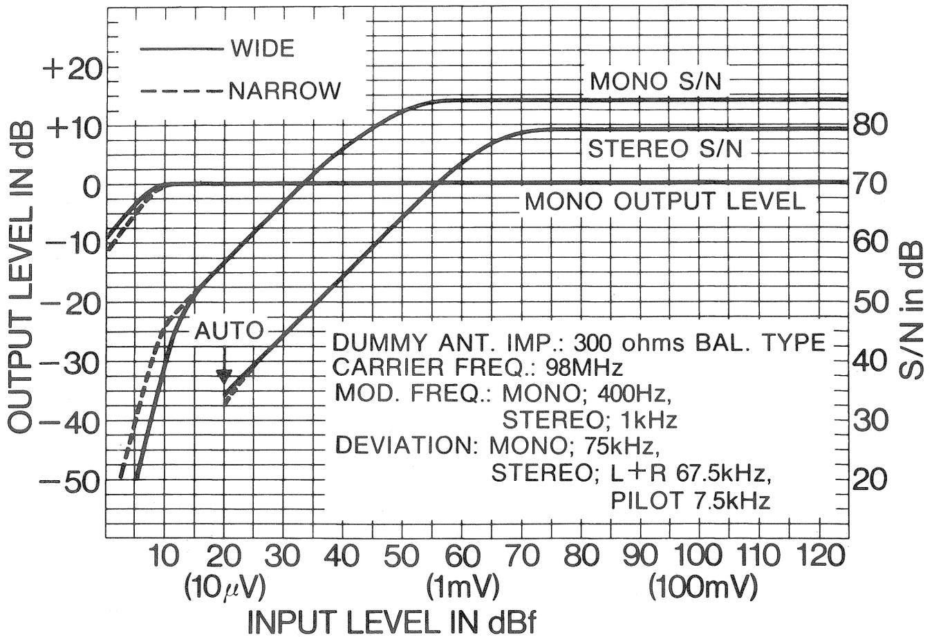
Fig. 3 Output level, S/N vs input level
