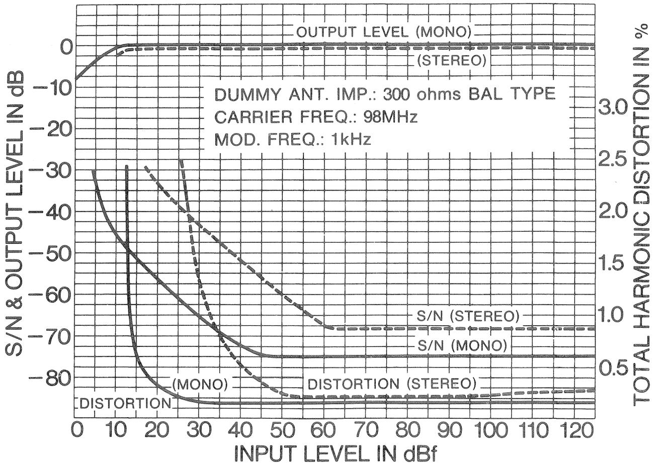
Fig. 6 Input vs output, S/N & distortion
