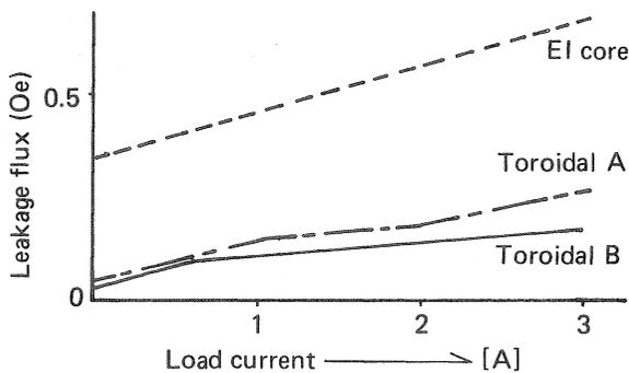
Fig. 11 Leakage flux
