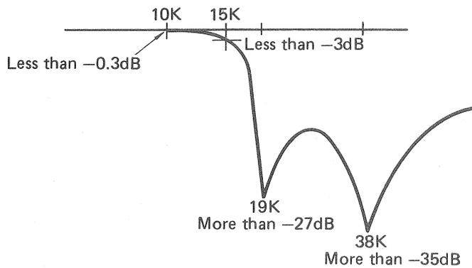
Fig. 19 Two-pole low-pass filter
