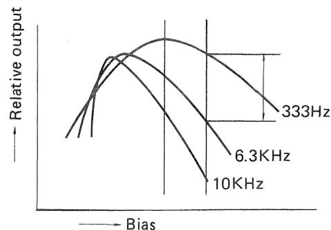
Fig. 7 Relationship between the volume of bias and output
