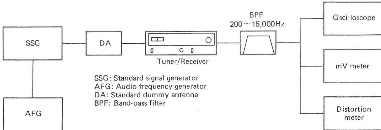
Fig. 5 Measuring S/N ratio at 65dBf
