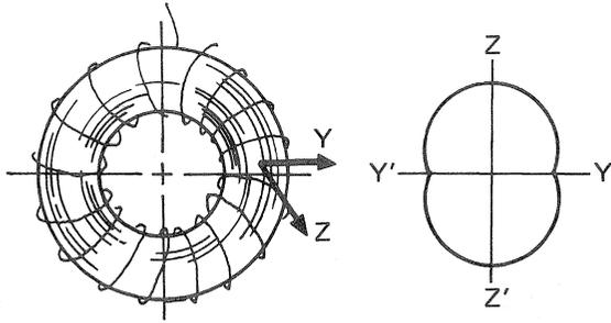
Fig. 10 The position of leakage flux
