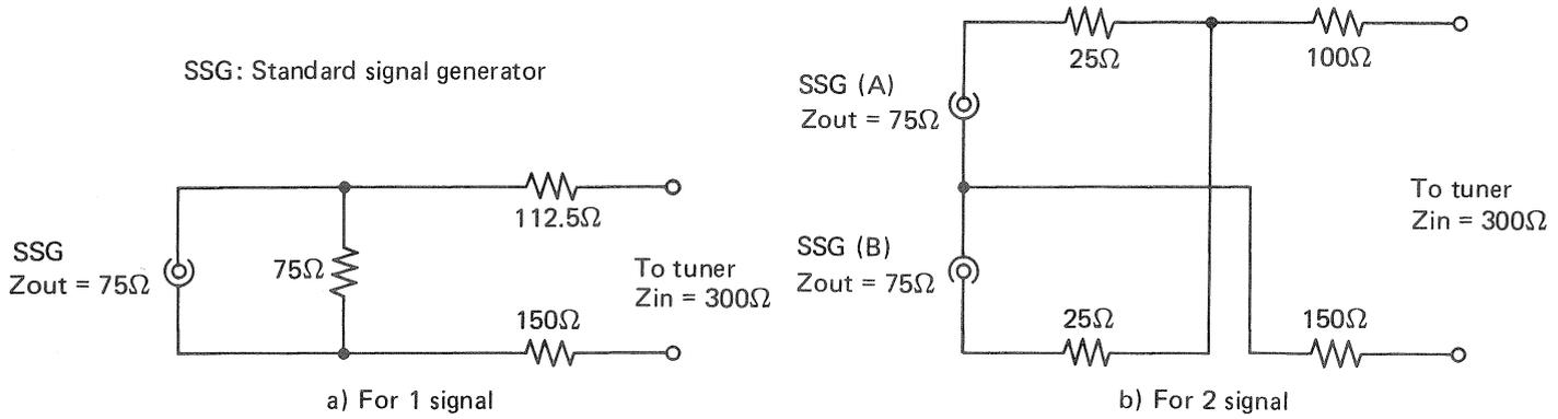
**Fig. 1 FM dummy antenna**
