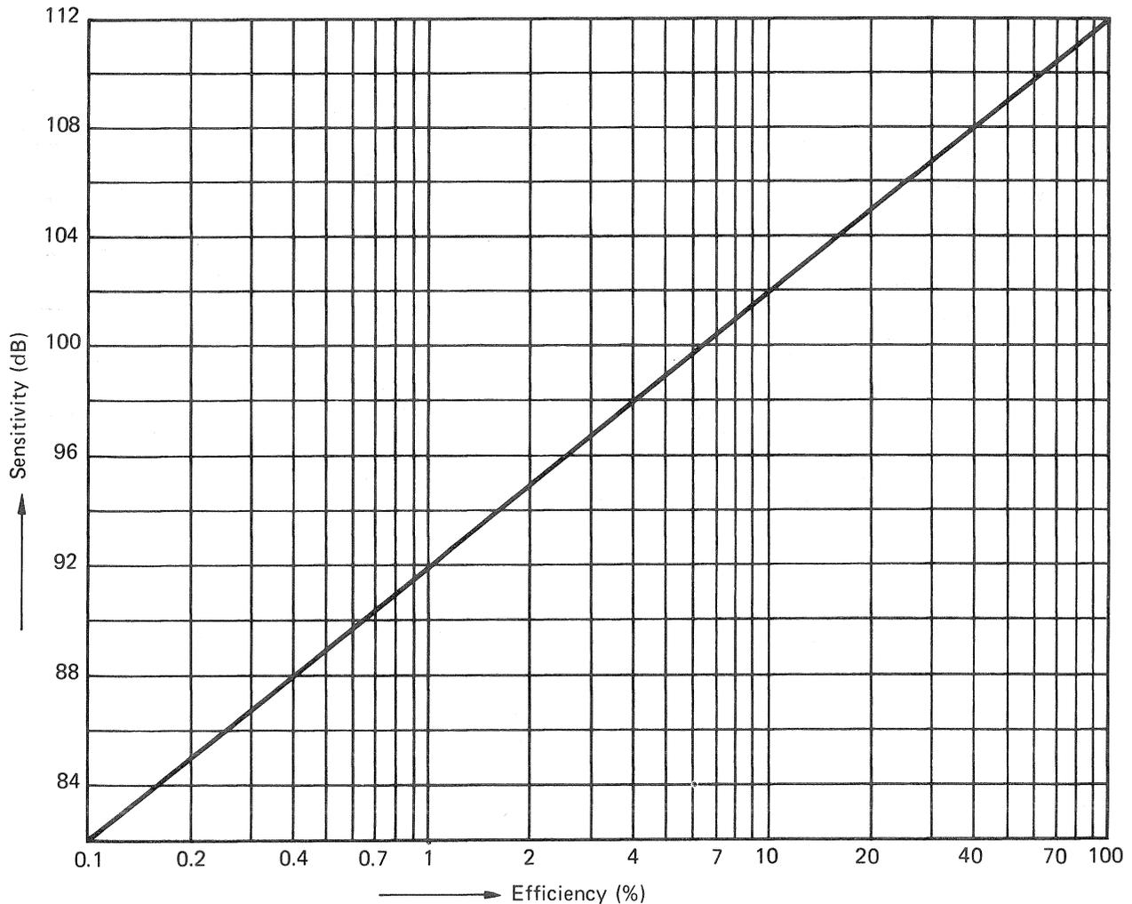
Fig. 3 Output sound pressure level at 1W input power and conversion efficiency
