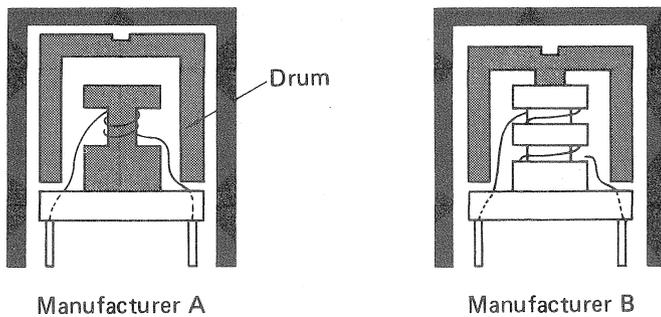
Fig. 16 The structure of IFT
