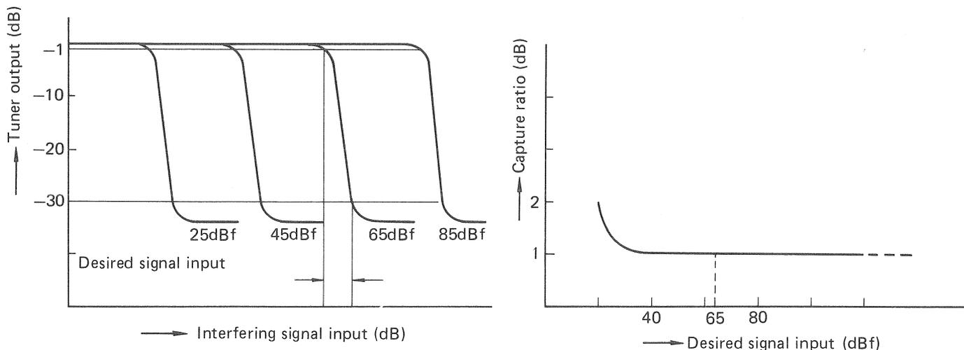
Fig. 8 Measuring capture ratio
