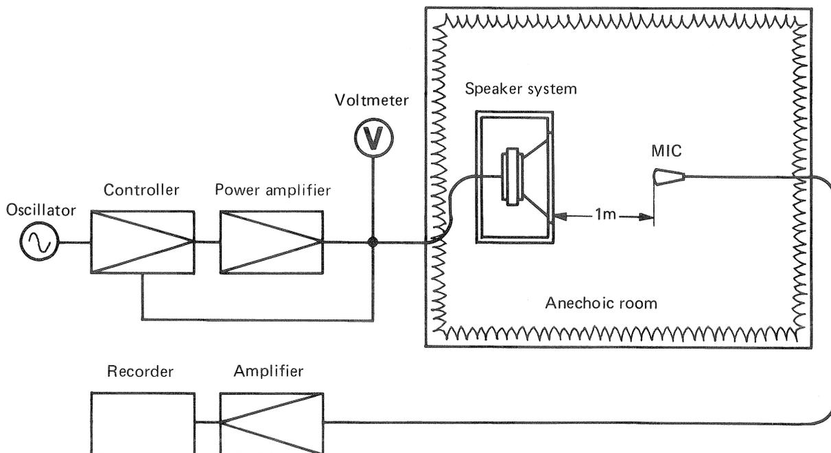
Fig. 1 The measurement of a speaker system
