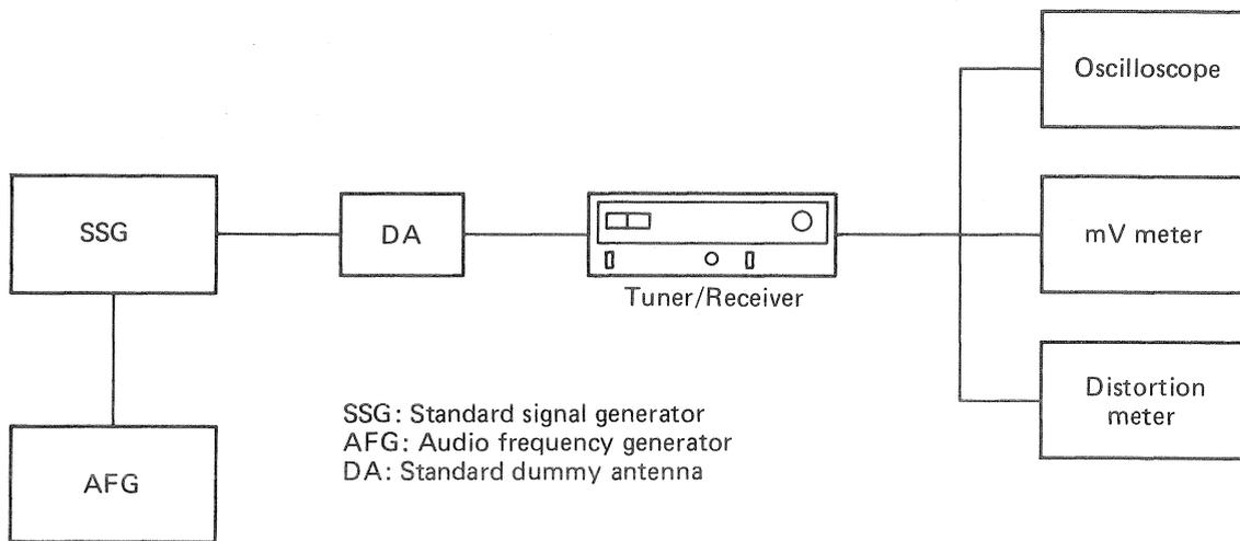
**Fig. 2 Measuring usable sensitivity**
