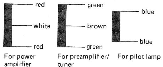
Fig. 12 Color classification of lead wires
