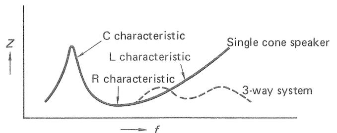
Fig. 21 Impedance characteristics of speaker systems
