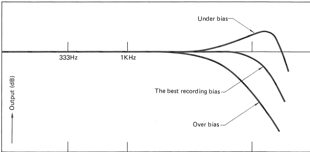
**Fig. 8 The change of bias volume and the frequency characteristics**
