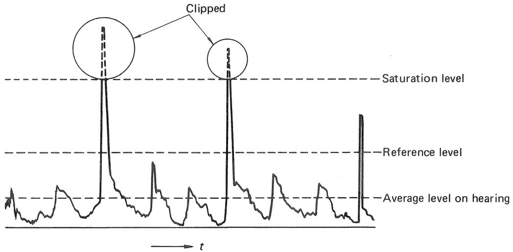
Fig. 2 The recording signal
