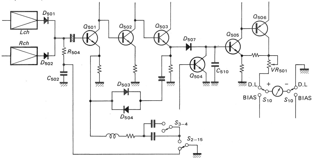
Fig. 3 Peak meter circuit
