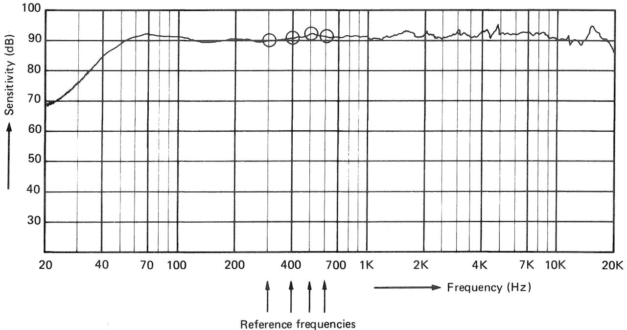
Fig. 2 Calculation of output sound pressure level
