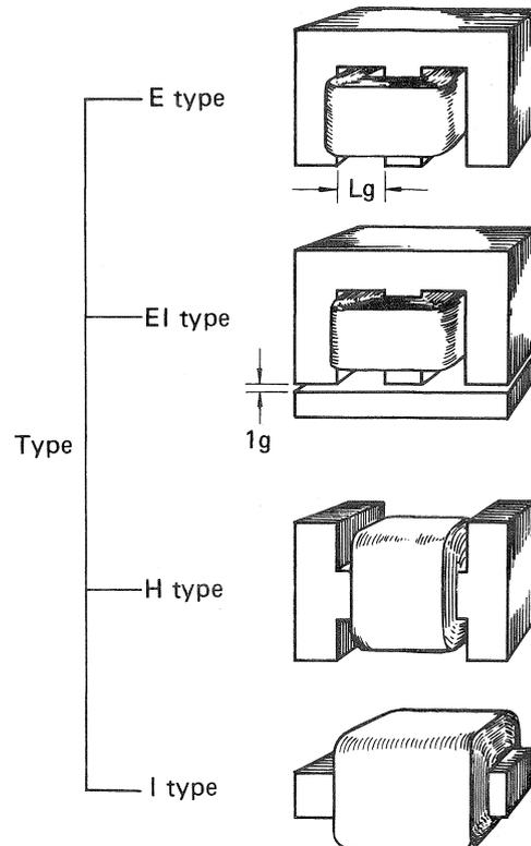
Fig. 22 Types of choke coils with cores of silic sheet steel
