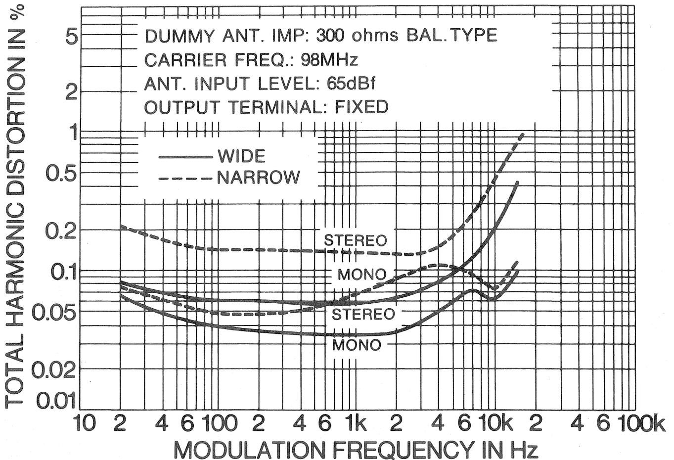
Fig. 7 Frequency vs total harmonic distortion
