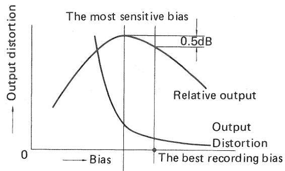
Fig. 6 Relation of the volume of bias, output and distortion
