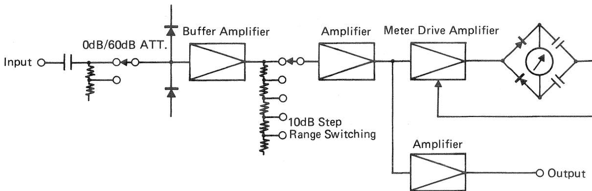
Fig. 2 Circuit composition of AC mV meter
