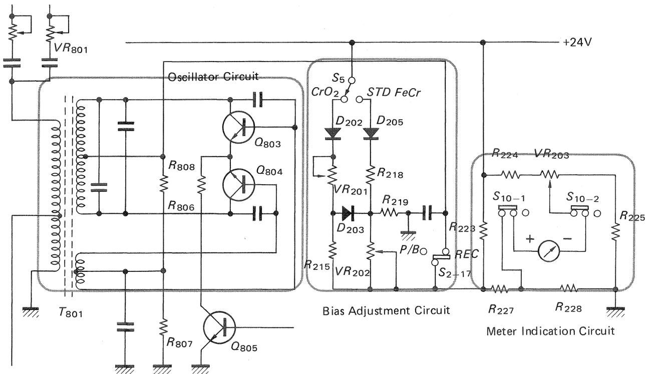
**Fig. 9 Bias Adjustment Circuit**
