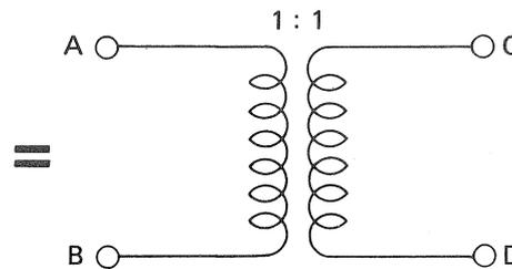
(a) An equivalent circuit of a bifilar winding
