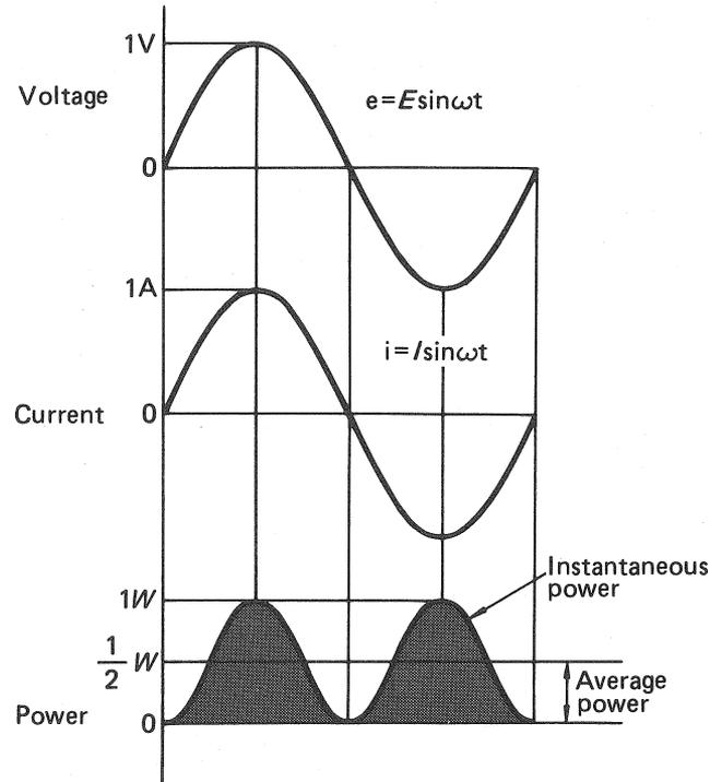
Fig. 4 Alternating current power
