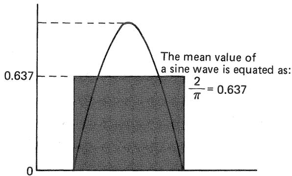
Fig. 3 Mean value of sine wave
