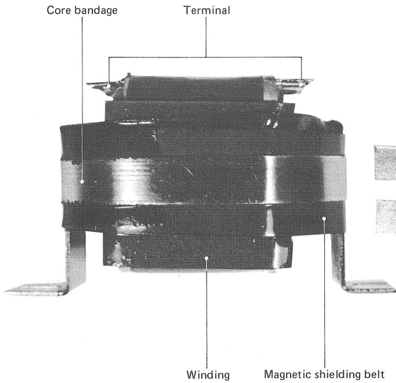
Photo 4 Cut core side view
