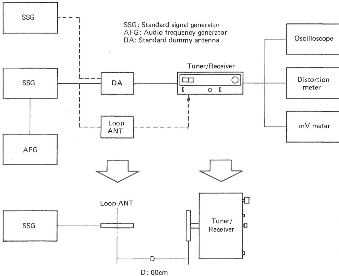
Fig. 15 Measuring AM specifications
