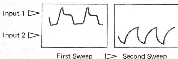
Fig. 11 Sweep in Alternate mode
