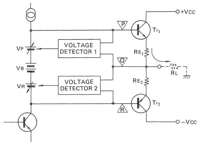
Fig. 4 Principle of Non-Switching amplifier
