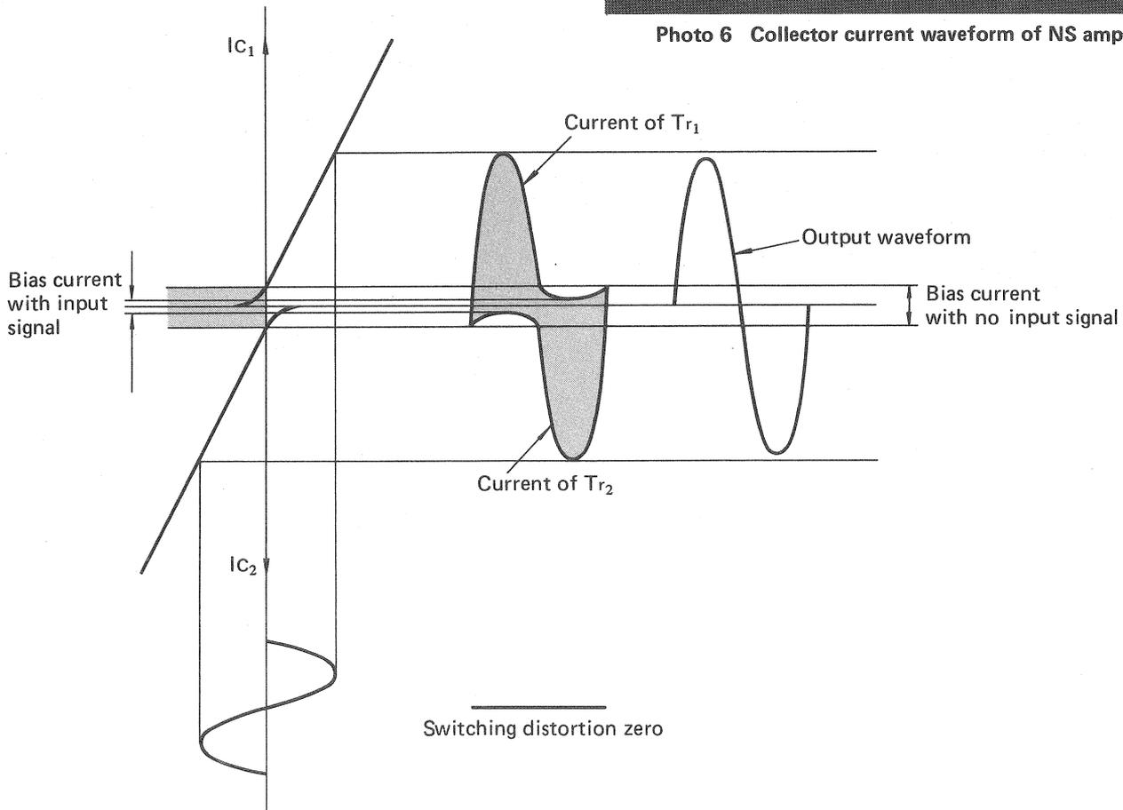
Fig. 7 Operation of Non-Switching amplifier
