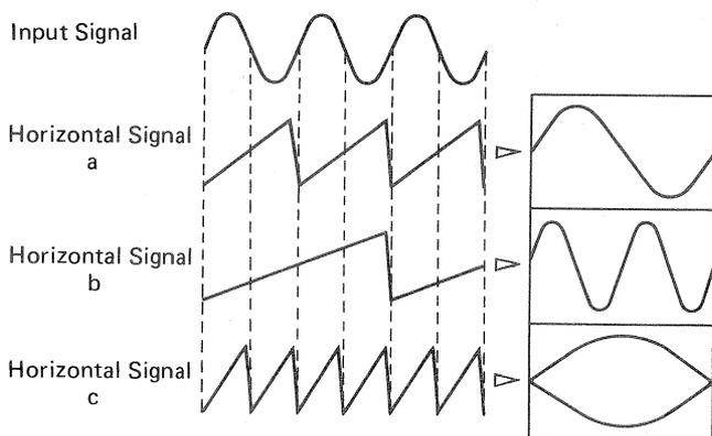
Fig. 5 Synchronization of repeating sweep type 'scope
