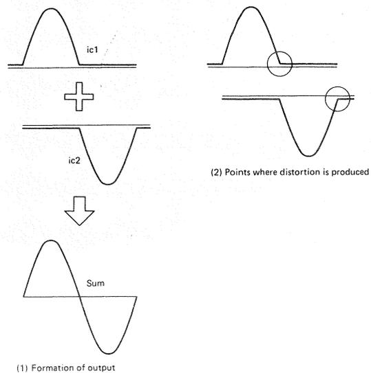
Fig. 20 In case collector currents are clear-cut
