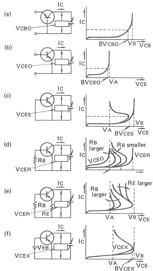
$V_A$ =avalanche breakdown voltage with emitter grounded
