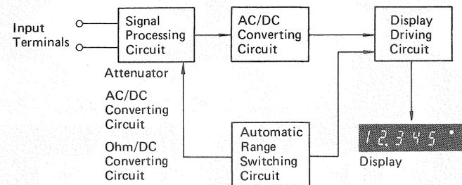
Fig. 1 Block diagram of digital multimeter
