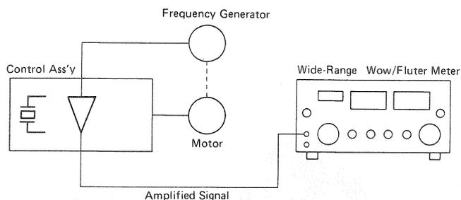
**Fig. 7 Wow/flutter measurement with FG output direct-reading method**
