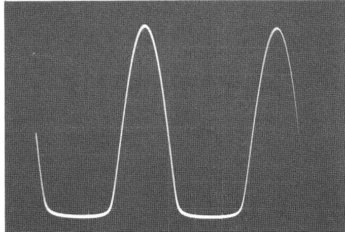
Photo 6 Collector current waveform of NS amp
