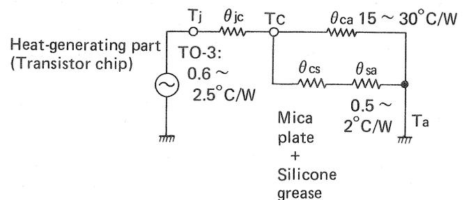
Fig. 5 Equivalent circuit of heat transfer
