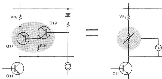
Fig. 16 Operation of Q17, Q19 & R39
