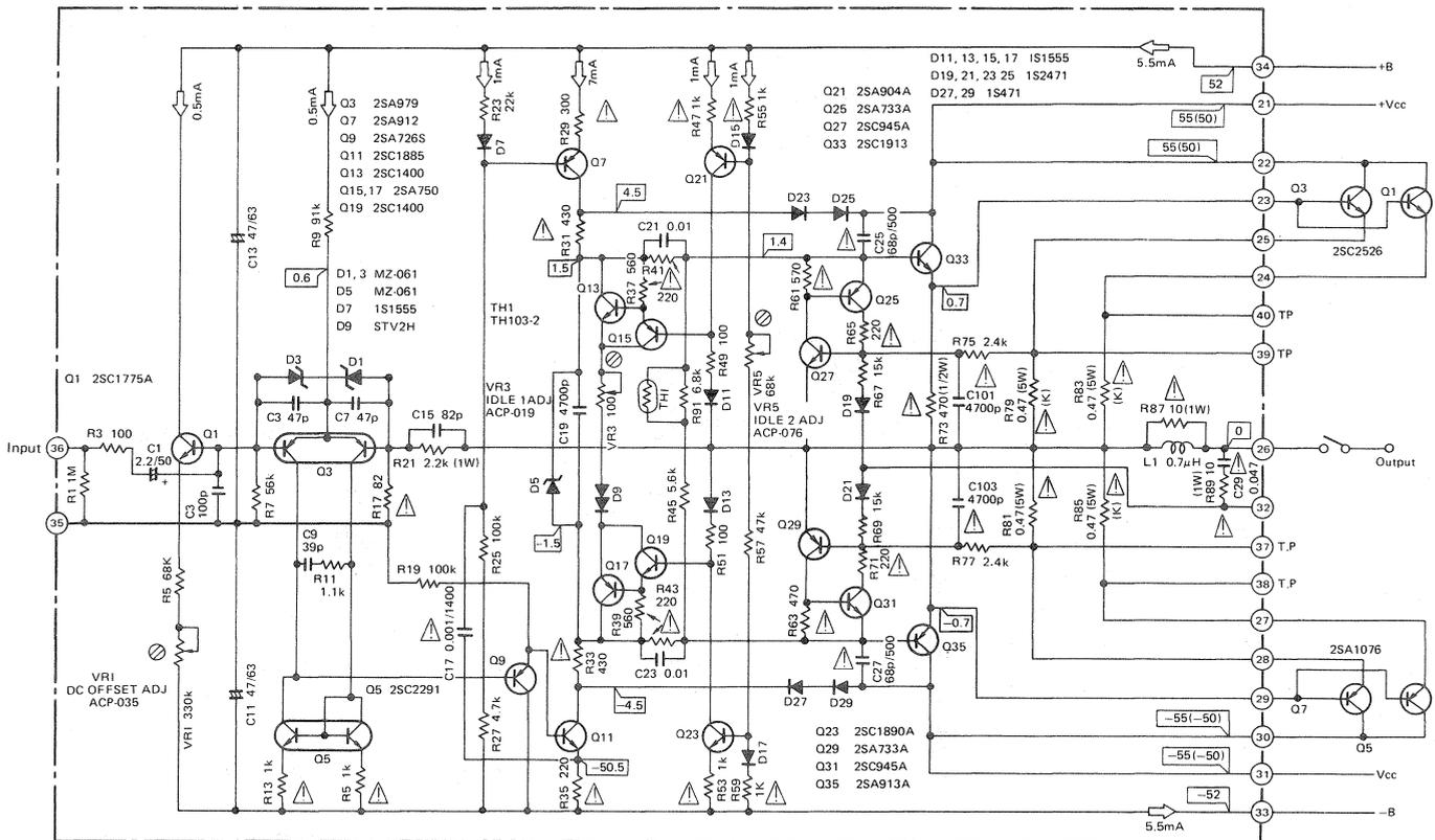
Fig. 8 Circuitry of SA-9800 Power Amp (Only left channel)
