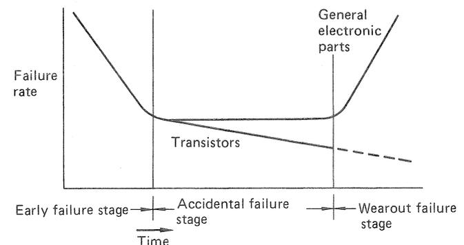
Fig. 4 Failure rate versus time lapse
