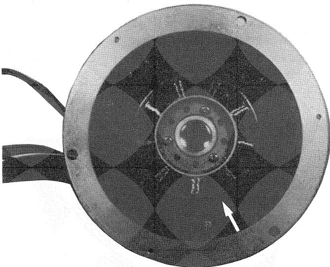
**Photo 5 FG in Quartz-PLL DD motor**
