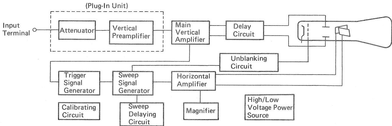
Fig. 8 Block diagram of trigger sweep 'scope
