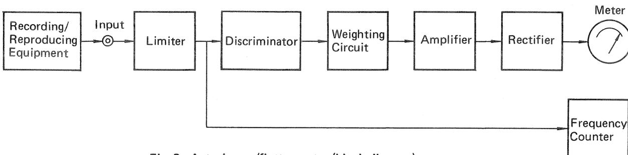
Fig. 2 Actual wow/flutter meter (block diagram)
