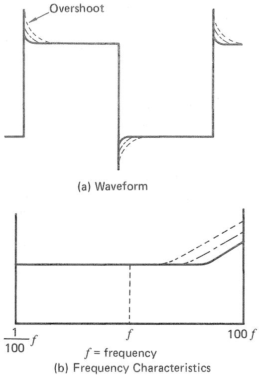
Fig. 9 Output waveform with overshoot
