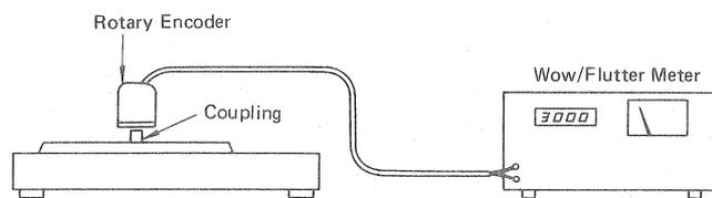
Fig. 5 Wow/flutter measurement using rotary encoder
