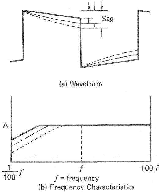
Fig. 8 Output waveform with sags
