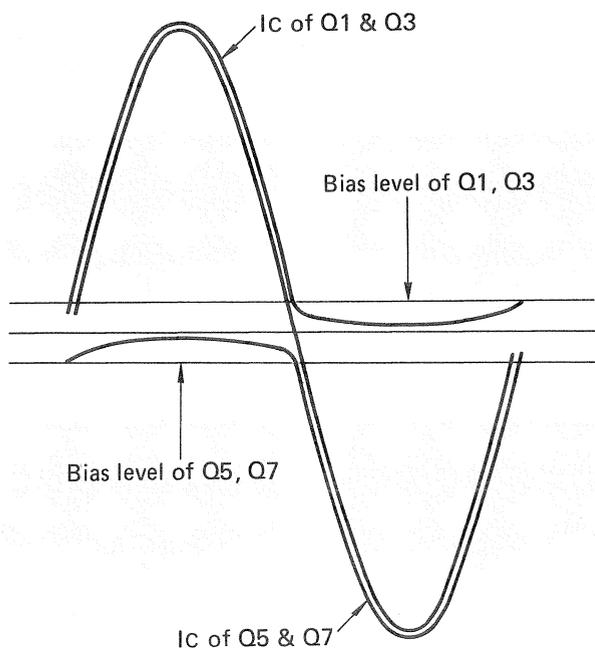
Fig. 19 Current waveform of output transistors
