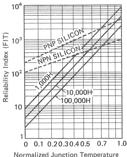
Fig. 2 Examples of NPN silicon transistor dilating curves
