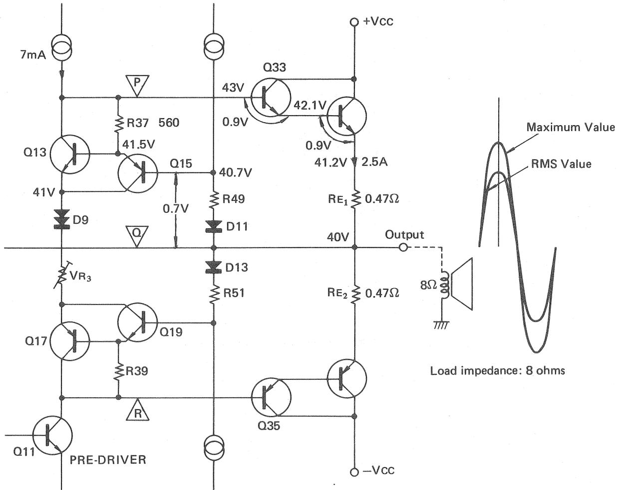
Fig. 10 Momentary potential at positive peak, 100W output
