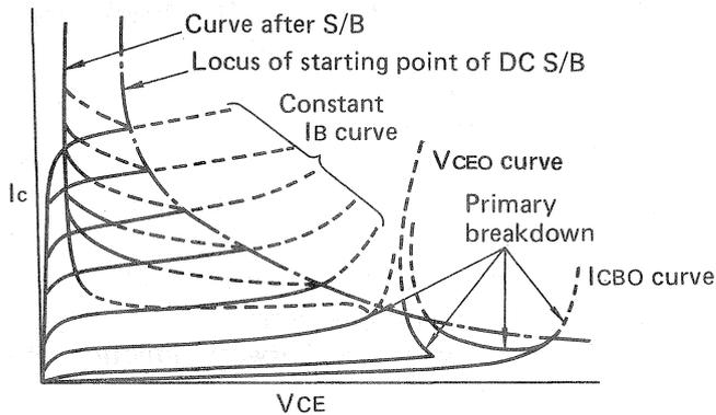
Fig. 3 Secondary breakdown phenomenon
