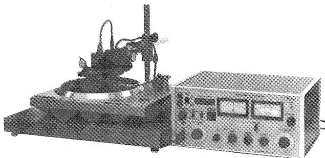
Photo 3 Wow/flutter measurement using rotary encoder
