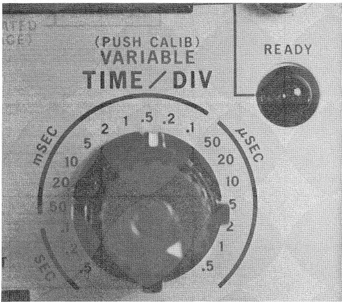
Photo 2 Time base of trigger sweep type
