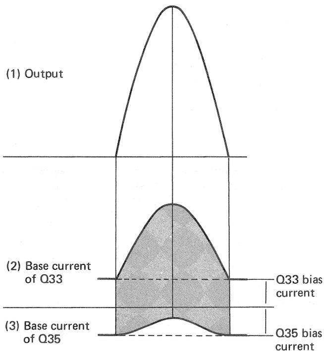
Fig. 14 Output and base current changes
