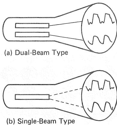
Fig. 9 Dual-beam & single-beam 'scopes
