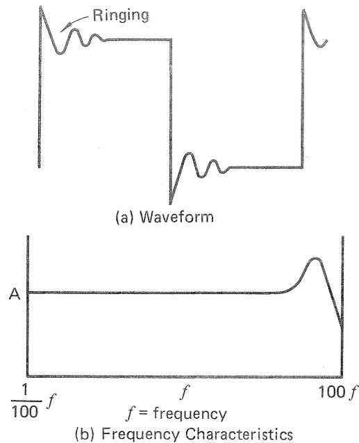
Fig. 11 Output waveform with ringing
