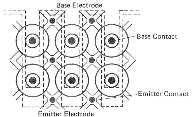
Fig. 21 Structure of a RET
