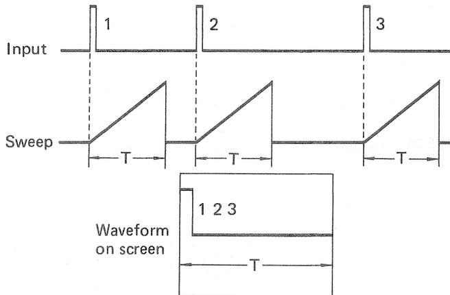
Fig. 12 Sweep in NORMAL sweep mode
