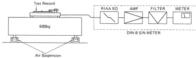
Fig. 9 Measuring S/N ratio
