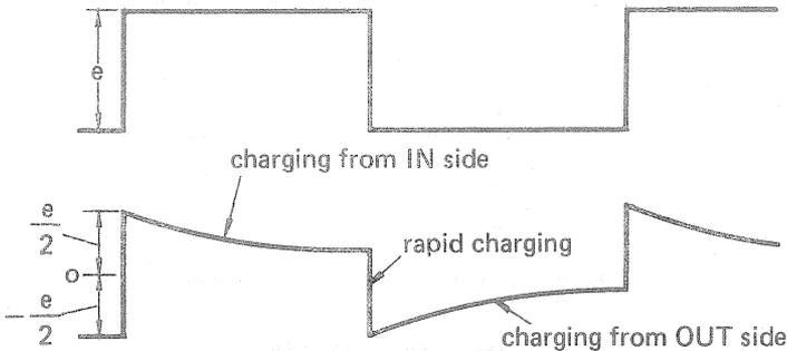
Fig. 5 In/output waveforms of High-pass filter circuit
