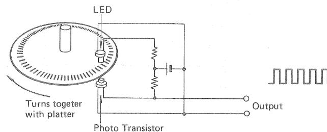
Fig. 6 Principle of rotary encoder
