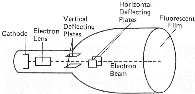
Fig. 1 Structure of cathode-ray tube
