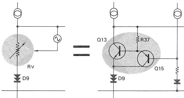
Fig. 11 Operation of Q13, Q17 & R37
