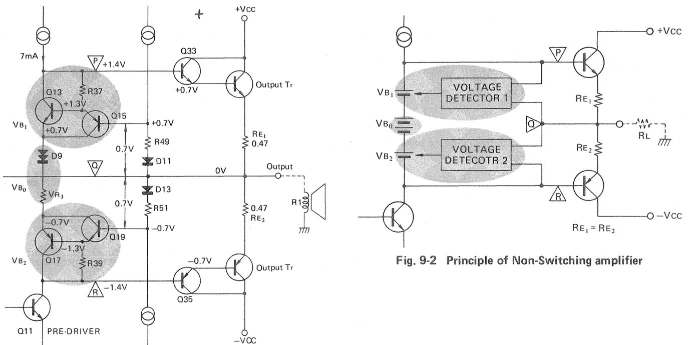
Fig. 9-1 Basic Non-Switching amplifier circuit.
