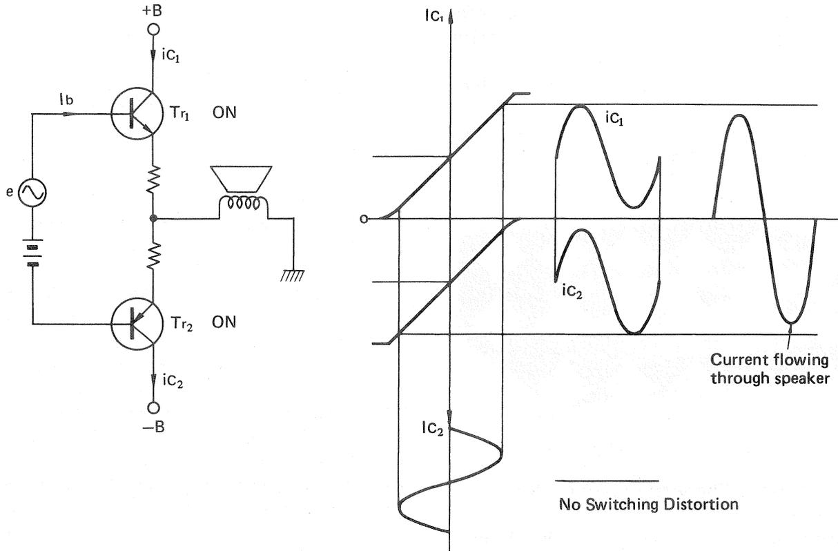
Fig. 2 Operation of Class A amplifier
