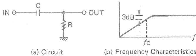
Fig. 4 High-pass filter circuit
