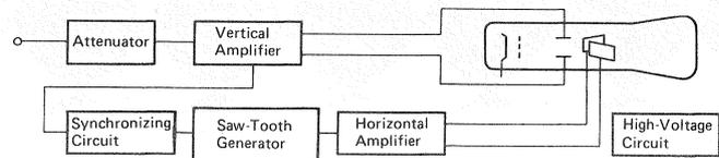
Fig. 4 Basic structure of the oscilloscope
