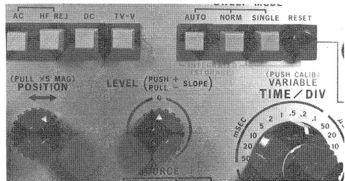
Photo 8 Trigger coupling and Sweep modes
