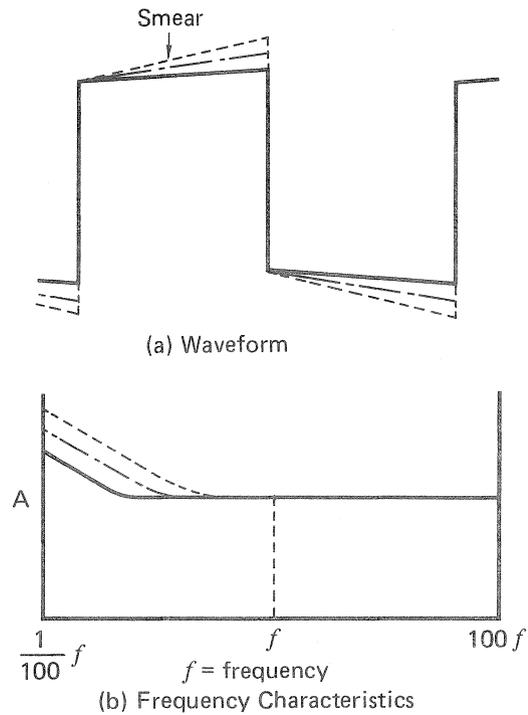
Fig. 10 Output waveform with smears
