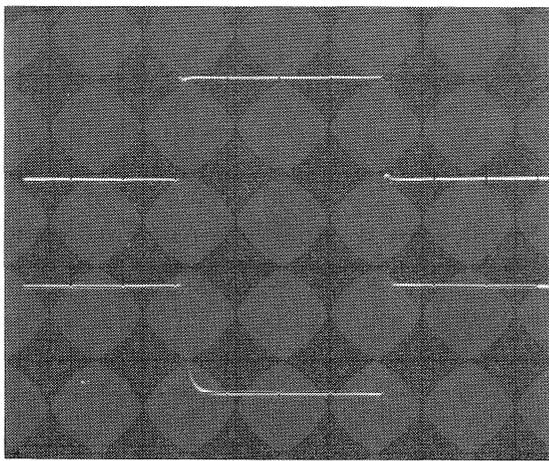
Photo 9-1 RET switching characteristics
