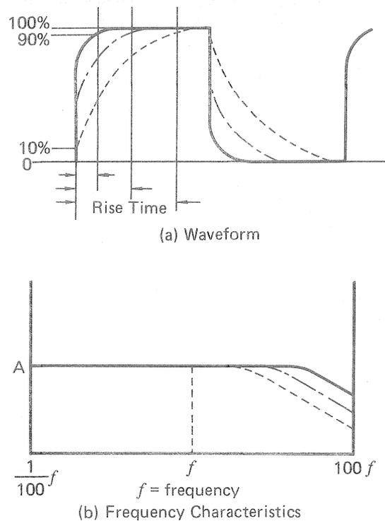
Fig. 7 Output waveform rise time
