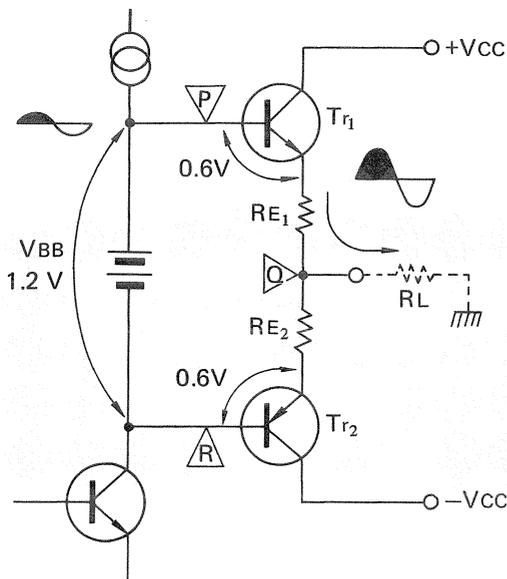
Fig 3 Basic class B circuit
