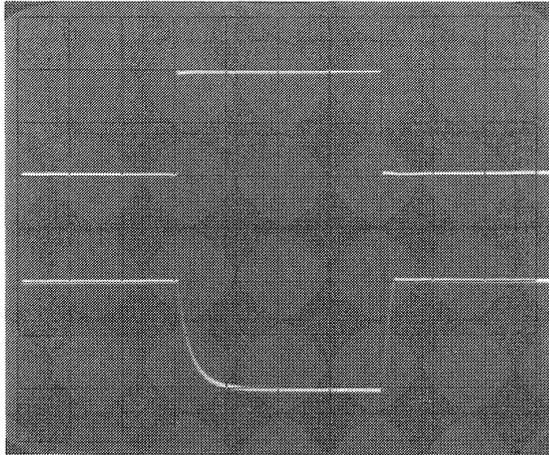
Photo 9-2 Conventional transistor switching characteristics
