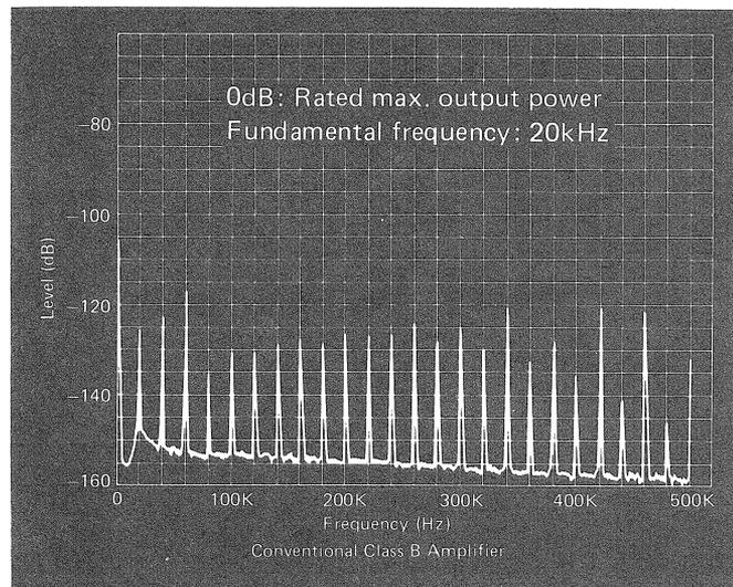
Photo 2 Distortion components
