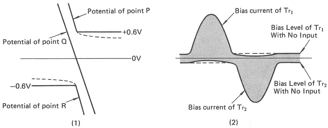
Fig. 6 Base potentials of  $T_{r1}$  &  $T_{r2}$  and bias
