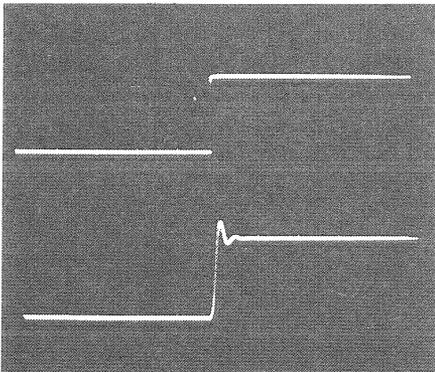
With capacitor,  $0.1\mu\text{F}$  (magnified: X 10)
