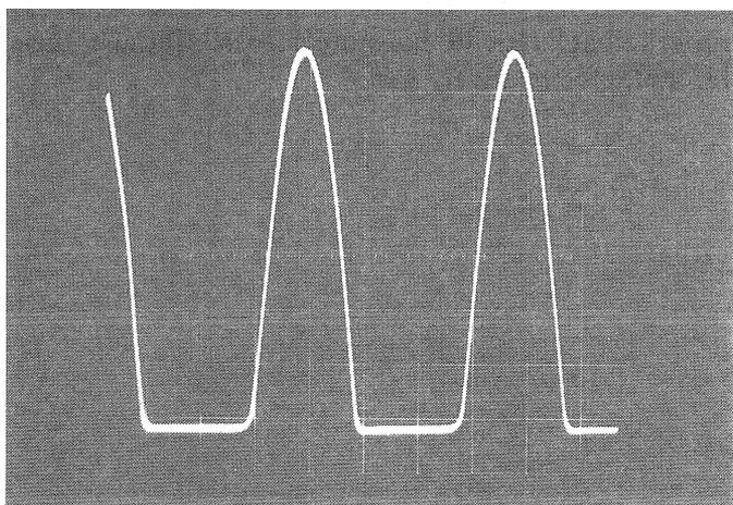
Photo 3 Collector current waveform of Class B amp
