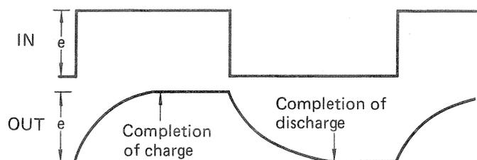
Fig. 3 In/output waveforms of a low-pass filter circuit
