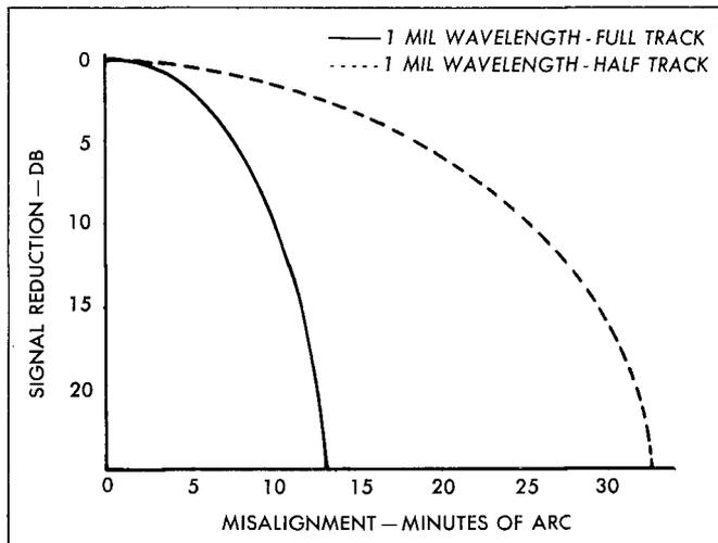
FIGURE 7. HIGH FREQUENCY LOSSES DUE TO HEAD MISALIGNMENT
