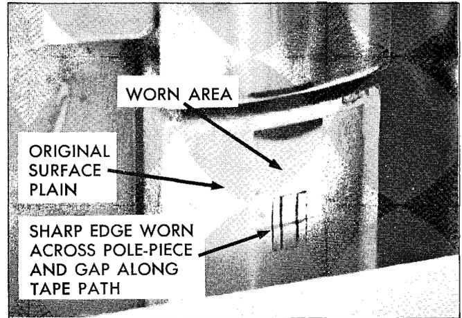
FIGURE 6. EXAMPLE OF IMPROPERLY POSITIONED HEAD EXHIBITING WEAR PATTERN
