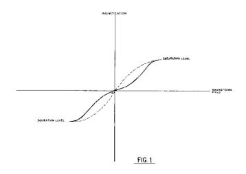
field (such as produced by a recording signal) is not directly proportional to the original signal. This characteristic, if not corrected would result in very bad distortion of
