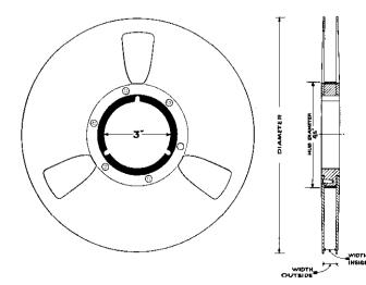
rubber ring .040" thick around the hub. With its higher coefficient of friction, the rubber threading ring makes thread-up possible by simply starting a turn of tape on the takeup reel so that the end of the tape is "buried." This is sufficient to anchor the tape and start it winding properly when the machine is started.
