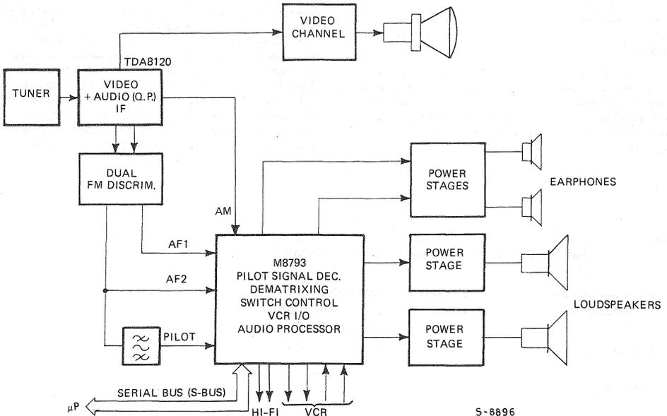
Fig. 6 - Block diagram of the stereo decoder and audio processor M8793
