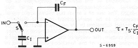
By means of switched capacitors and operational amplifiers, it is possible to implement many filter configurations.
