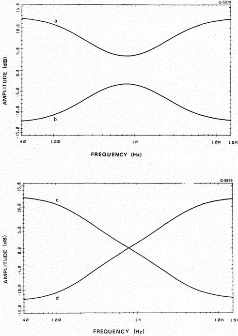
Fig. 14 shows frequency response of tone control circuit when full loudness correction is inserted together with maximum tone boost. Tone control is common to both channels.
