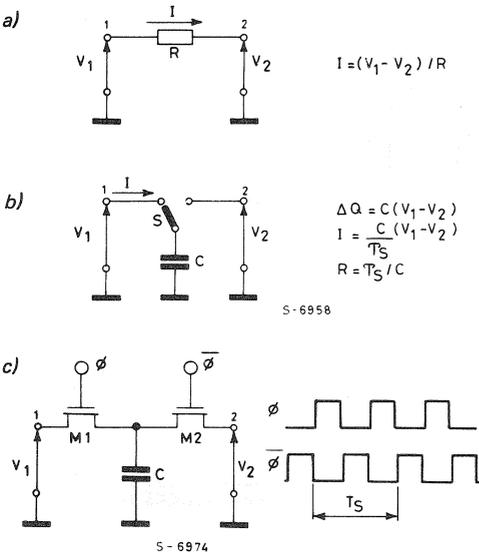
The basic concept of a SC circuit is a charge transfer between two nodes by means of switches and a capacitor (fig. 2).
