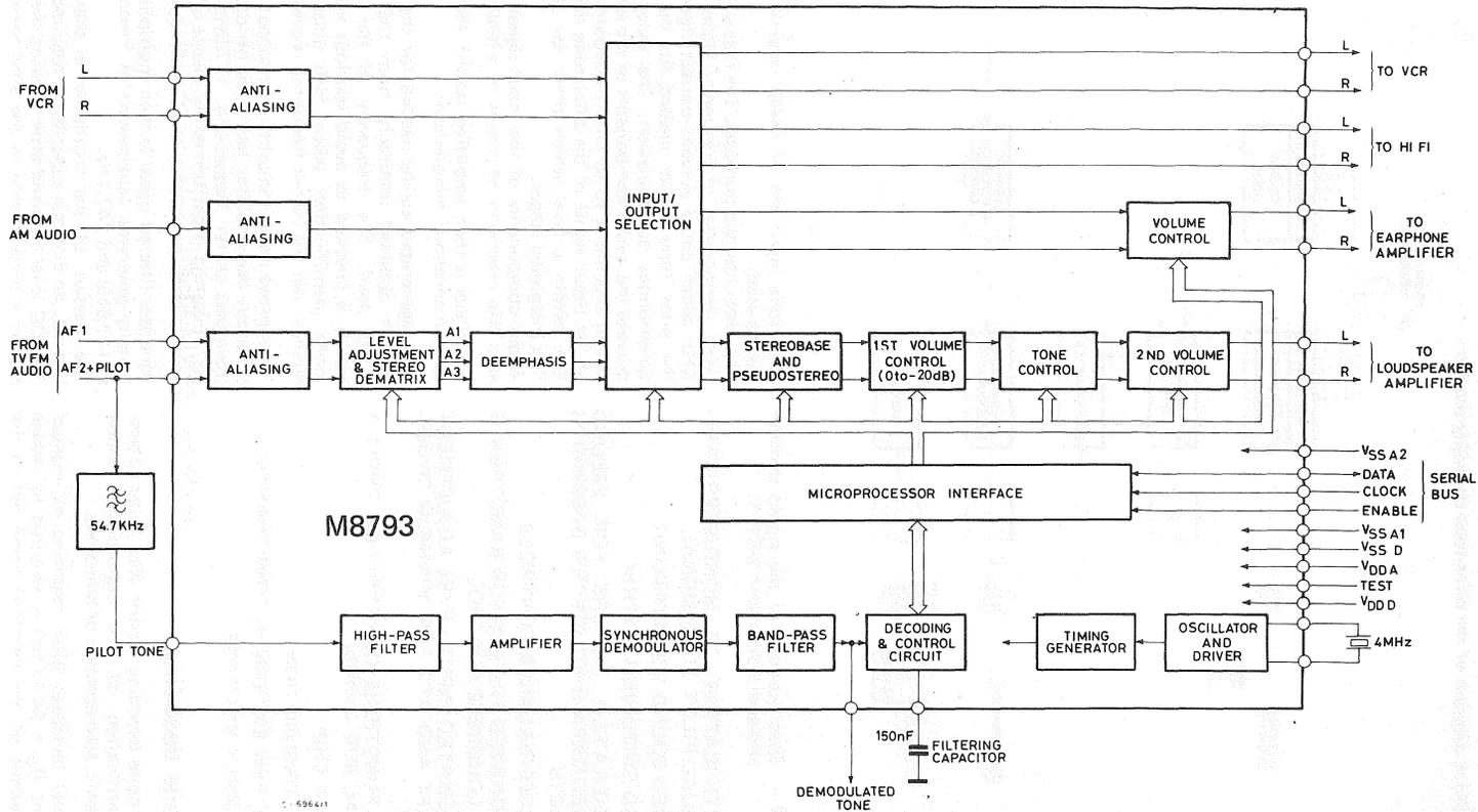
Fig. 7 - Block diagram of the pilot-tone decoding section
