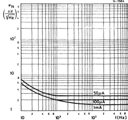
Fig. 6 - Equivalent input noise current vs. frequency (input transistor Q1)
