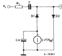
As can be seen there is a pair of diodes in anti-parallel supplied by a current generator whose output is proportional to the DC voltage present at pin 16 ( $C_0$  is a short circuit for the changing components of the signal). Diodes D1, D2 act as a dynamic resistance to the negative and positive half-waves respectively.
