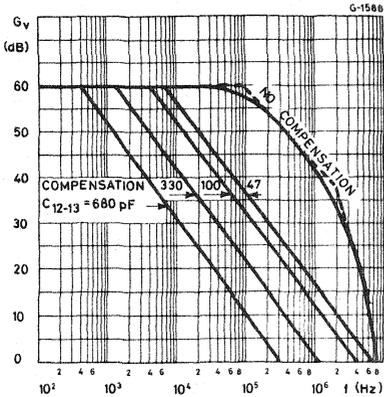
Fig. 12 - Open loop phase response vs. frequency (equalization amplifier)
