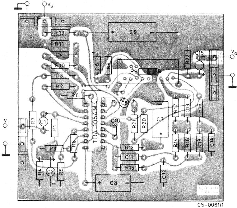
Fig. 30 - Application circuit for low-cost cassette player and recorder
