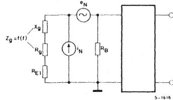
For the time being we shall disregard the noise due to the second transistor and for convenience the signal to noise ratio will be calculated considering the open-loop circuit shown in fig. 49. In fact as is known the signal to noise ratio does not depend (for the same band) on the presence of negative feedback.
