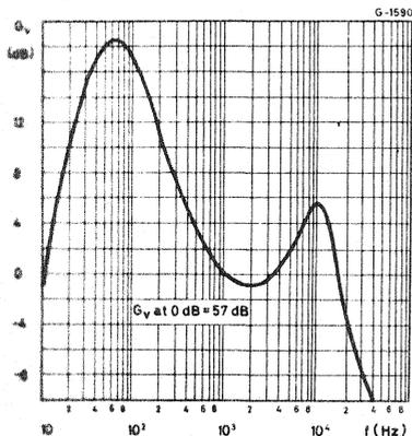
For frequencies greater than 1 kHz the circuit response depends mainly on the transfer impedance of the T circuit (formed by C12 + R15, C11, R16) relative to R12.
