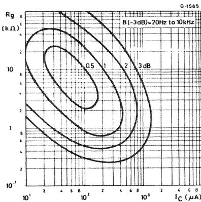
Fig. 9 - Optimum source resistance and minimum NF vs. bias current (input transistor Q1)
