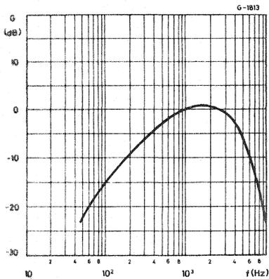
The signal at the terminals increases linearly as a function of the frequency with a slope of 20 dB per decade until about 1.5 kHz, after which it decreases rapidly because of losses due to the finite section of the head gap, the selfdemagnetization of the tape, the thickness of the magnetic coating on the tape, the finite distance between tape and gap and finally due to electrical losses in the copper and iron of the head.
