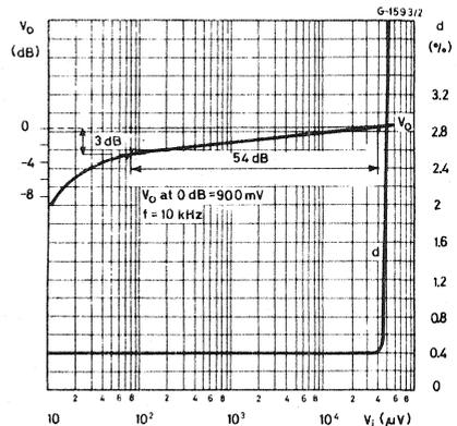
Furthermore over the whole control range the harmonic distortion remains very low ( $d = 0.4\%$ ). Fig. 26 shows distortion as a function of frequency when recording with automatic level control.
