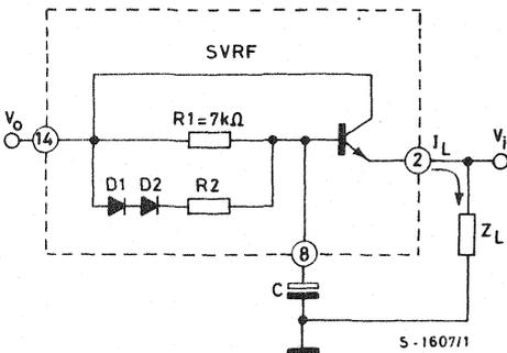
At the moment of switch-on the capacitor C is charged with a very short time constant by means of the diodes and R2 ( $R2 \approx 100 \Omega$ ).
