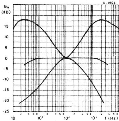
Fig. 42 - Frequency response of the preamplifier equalizer (RIAA) in the circuit of fig. 38
