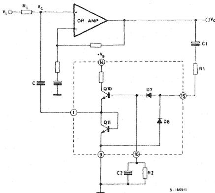
Fig. 19 - Basic dynamic attenuator circuit
