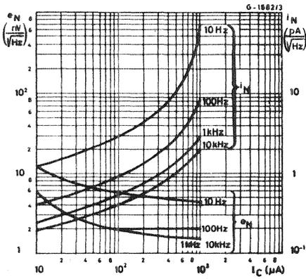
Fig. 8 - Noise figure vs. bias current (input transistor Q1)
