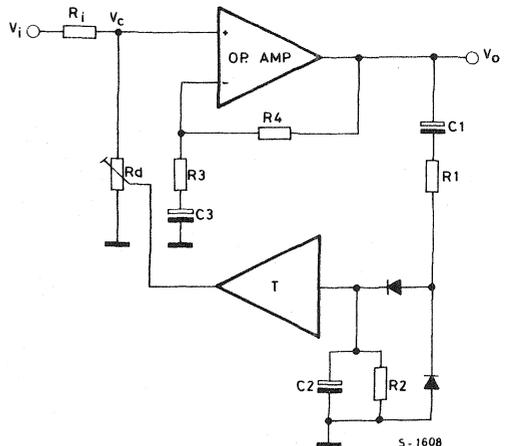
This consists of an amplifier (OP. AMP.) having constant gain ( $G_V = 1 + \frac{R_4}{R_3}$ ), which in feedback
