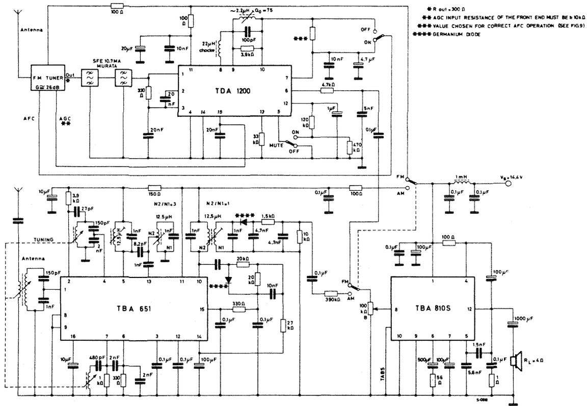
Fig. 14 - Circuit diagram of AM/FM portable radio
