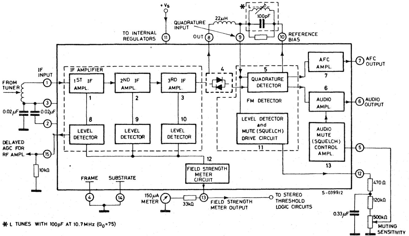
Fig. 2 - TDA1200 schematic diagram
