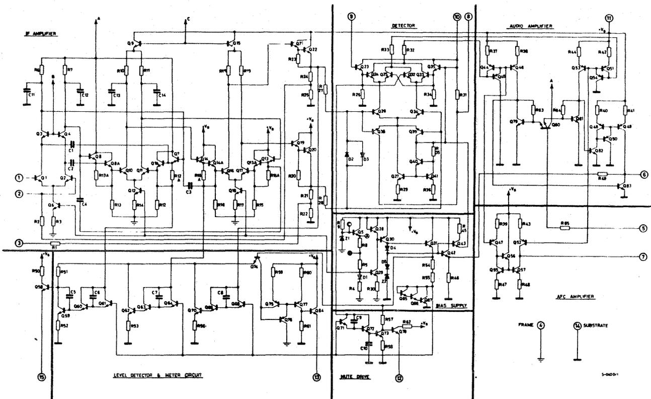
which is limited by two diodes D2 and D3, comes directly to the first input (bases of Q26 and Q34); it reaches the second input (pin 9) by means of an external circuit which introduces a phase-shift proportional to the instantaneous frequency and a static  $90^\circ$  shift at the nominal frequency of 10.7 MHz.
