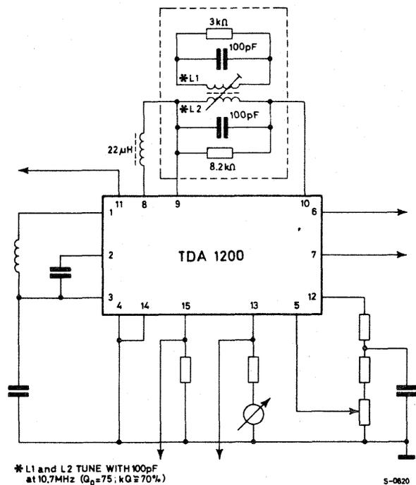
Fig. 4 shows the detected output signal as a function of the input signal. The circuit can handle fairly high input voltages ( $> 500$  mV) without any deterioration of AM rejection; when functioning normally the AGC of the tuner prevents signals of amplitude greater than 10 mV from reaching the input of the device, since AGC intervention occurs for input signals of approximately 10 mV.
