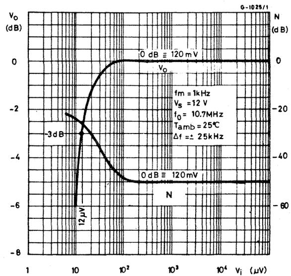
Fig. 5 - Typical capture ratio vs. input voltage
