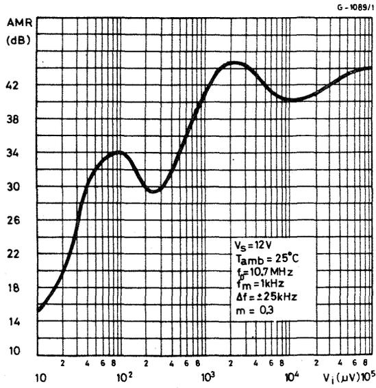
Fig. 8 - Typical AMR vs. change-in tuning frequency
