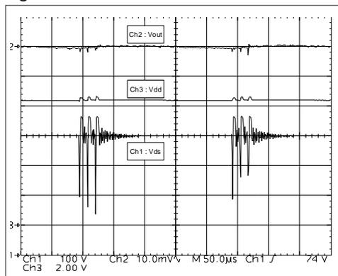
This results in missing cycles, as shown on the following scope waveform ( $V_{in} = 400V$ ,  $I_{out} = 30mA$ ).
