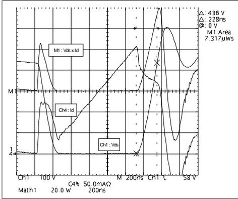
Note that the right cursor has been set at the same value as the turn on voltage. This assumes that nothing is dissipated at turn off, because the cross over time is only due to capacitor charging (The one of the device itself) and the internal turn off of the power mosfet is sufficiently fast. The corresponding energy of this capacitor is dissipated at turn on, and this explains that only the part of voltage which is discharged at turn on is taken into account at turn off.
