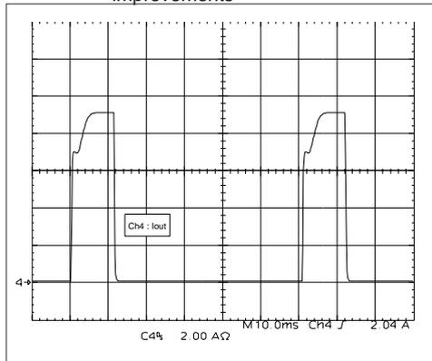
Also note that an optimization of the transformer can lead to the same results. But the primary peak current must always be limited to a value compatible with the application. This could be done in most cases by the right device choice (VIPer100, VIPer50 or VIPer20).
