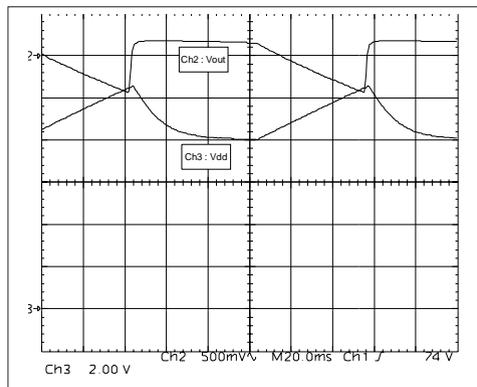
Each time that the  $V_{dd}$  voltage reaches the low threshold voltage of the UVLO logic, the device is reset and the  $V_{dd}$  capacitor is charged back to the high threshold of this UVLO logic thanks to the start up current source which is turned on. The recurring period of this phenomenon is about  $110ms$ . This behaviour leads to the following drawbacks :
