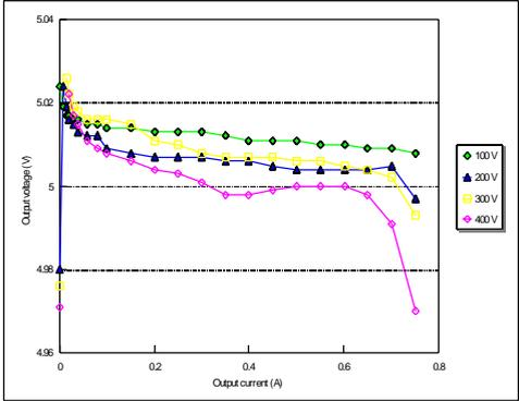
It can be seen that the bad burst mode leads to a slightly lower voltage than the nominal one, but is still convenient for voltage checking: If the power supply is operated without any load, the output voltage is still very close to the normal output voltage and this can be used for checking the output voltage. Also, the output ripple is far less than in figure 6, where the worst case was shown.
