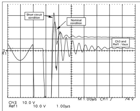
A solution to get rid of these spikes is to implement a filter, by just increasing R2. But this leads to poor performances in regulation, especially for light loads, where the bad burst mode will appear sooner (i.e. for larger current than in figure 7).
