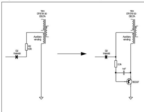
Note that R2 was doing the same thing, but in a less efficient manner. In nominal mode, this resistor avoids excessive Vdd voltage, which should reach the internal reference voltage and interferes with the secondary feedback. With the new design, it is possible to eliminate this resistor, and even to add two turns more on the auxiliary winding.
