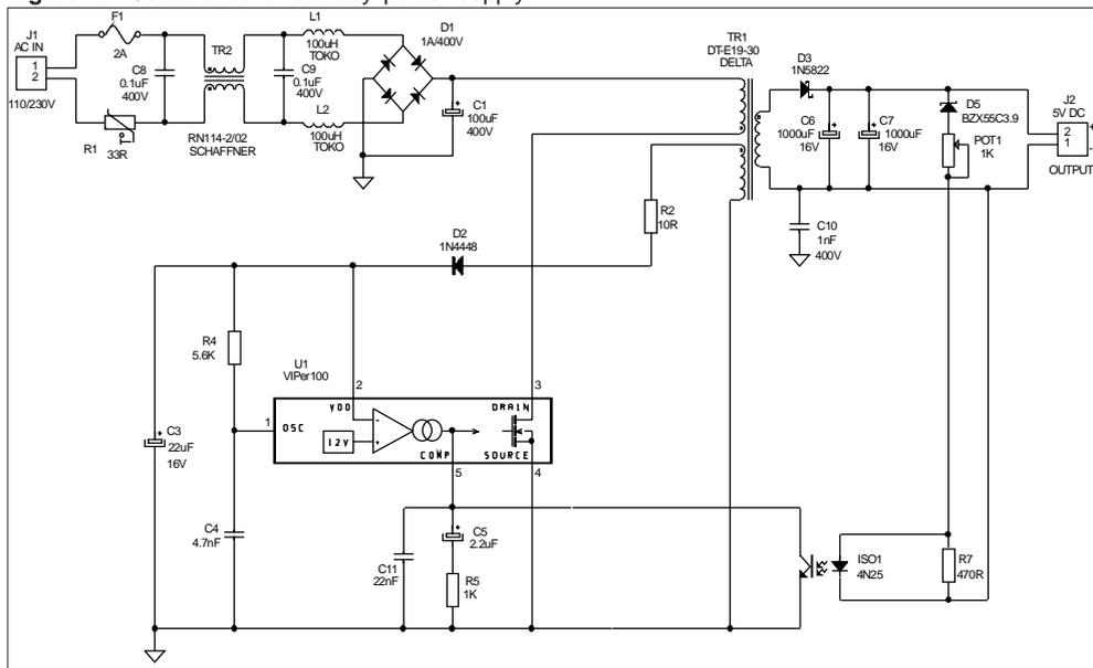
5. A resistor R7 has been added across the diode of the optocoupler to increase the biasing current of D5. This improves the dynamic performance of the power supply.
