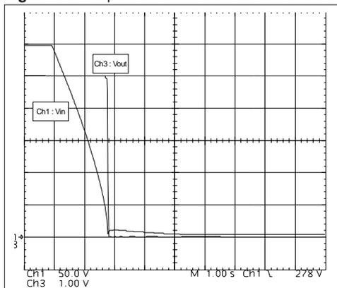
The protection which is foreseen for the VIPer100 consists of a monitor of the Vdd voltage and to switch off the device when this voltage is below the low threshold voltage (8V) of the UVLO logic. This is done naturally when the output voltage is low (i.e. in short), because the auxiliary winding is delivering a Vdd voltage which is proportional to the output voltage.
