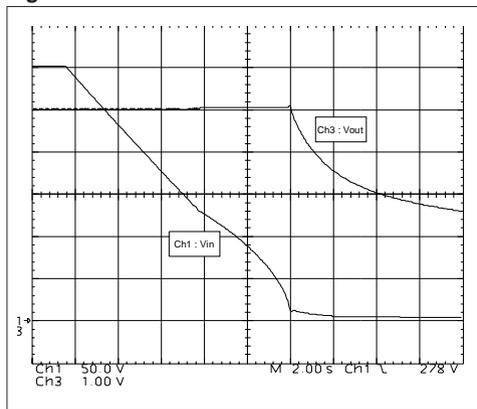
**Figure 15.** Turn off in full load condition
