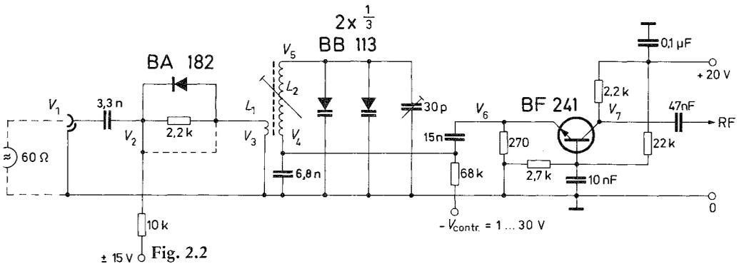
The divided circuit voltage is tapped at point C and fed to the emitter. This coupling offers the advantage that the load transformation changes as a function of frequency. At low frequencies a better circuit attenuation may be achieved than at high frequencies, i. e. the selection may be maintained more uniformly over the frequency range.
