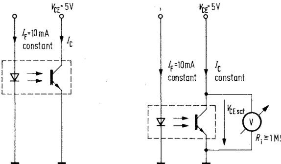
The analogy with the transistor goes so far that, except of course for the isolation characteristics, one can gauge couplers at the plotter oscilloscope like transistors with extreme low current amplification.
