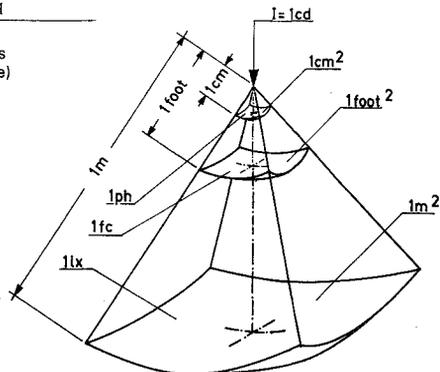
Luminous flux  $\phi$  per second per sterad (sr) 1 lumen (lm)
