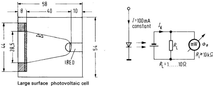
In cases where IRED emitting diodes are used in connection with mirrors or lenses, for example in light barriers it can prove useful to state the radiant power (radiation capacity)  $\Phi_e$  defined in a cone with the half viewing angle  $\varphi$ , respectively the curve  $\Phi_e = f(\varphi)$  – (Fig. 14)
