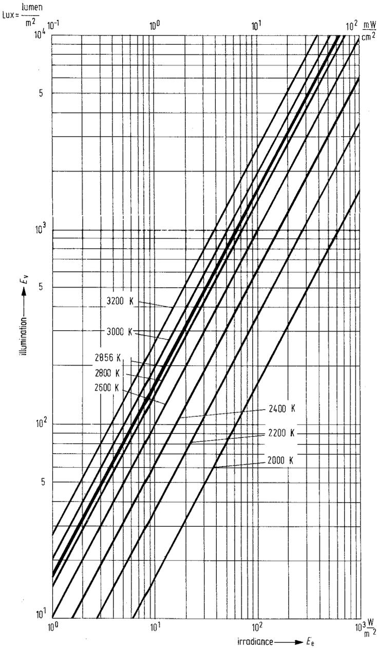
**Conversion of  $E_v$  (lx) into  $E_e$  ( $W/m^2$  or  $mW/cm^2$ ) referred to the radiation of a black radiator**
