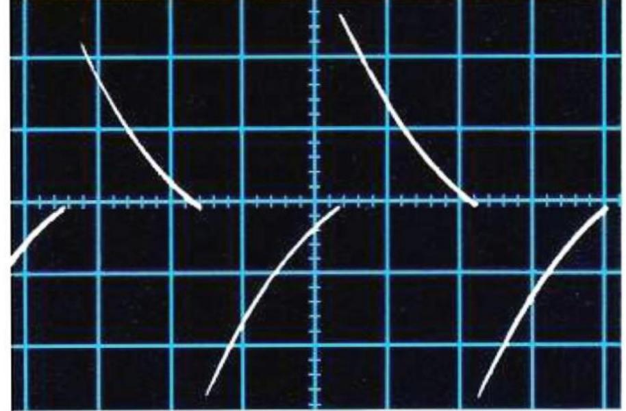
We can see the shape of the 20Hz square wave of a typical Harman Kardon amplifier. The tilt is less than 3%.
