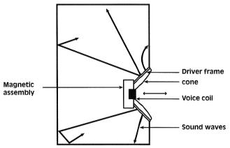
2. Sound pressure waves within the enclosure are formed by the moving cone as it responds to input signals. These pressure waves can generally be damped by using dacron or a similar material inside the enclosure. The choice of the proper material and density of the material is of critical importance for the proper absorption of unwanted energy. Refer to diagram 2.
