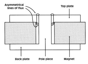
The uneven lines shown in Figure 1. create an asymmetrical magnetic flux field which results in higher distortion. Both the Infinity/Watkins dual voice coil woofer and midbass coupler utilize an extended pole piece which creates symmetrical lines of flux in the magnetic gap as shown in Figure 2. This significantly lowers distortion.
