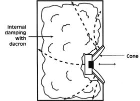
The enclosure must be constructed so it is rigid and cannot respond to the pressure waves generated by the drivers. By use of special material and properly placed internal bracing, unwanted resonances and vibrations can be minimized so they will not interfere with the sound emanating from the drivers.
