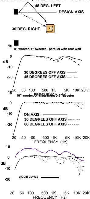
**Figure 23.** A room layout in which the loudspeakers are facing directly forward, as happens in many home stereos and custom installations. In this case the "best" sound component misses the listener completely and is lost in the general reverberant sound field in the room. If the loudspeaker does not have constant directivity, the system will take on a coloration related to how the loudspeakers misbehave off axis.
