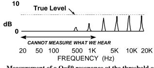
Measurement of a Q=50 resonance at the threshold of audibility using a time window of 17 ms (60Hz)
