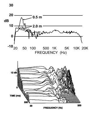
**Figure 17.** A comparison of before and after measurements showing the dramatic improvement resulting from moving the listener out of the powerful high-pressure region of the second order length mode in the room.
