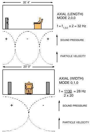
**Figure 9.** A view of a listening room showing the distribution of sound pressure and particle velocity for the second-order mode, 2,0,0, along the length of the room
