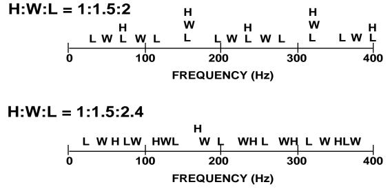
**Figure 3 (top)** Axial modes calculate for a rectangular room. "L" identifies a length mode, "W" a width mode, and "H" a height mode. The dimensions are simple multiples of each other and, as a consequence, there are regularly repeated combinations of the same axial modes, and similarly regular gaps. This room is likely to have some problems.
