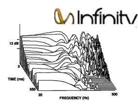
**Figure 20.** A "waterfall" plot of the situation after parametric equalization.
