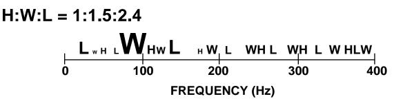
Figure 4 In this diagram the size of the mode identifiers has been adjusted to reflect their audible importance to a listener in a realistic stereo system setup.
