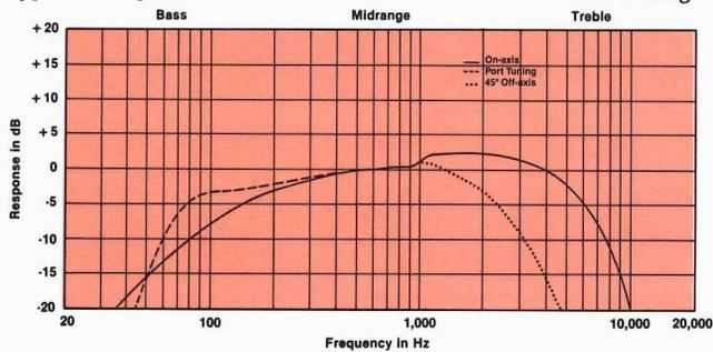
Frequency response of the 2118H/J in a closed box of 14 L (0.5 ft<sup>3</sup>) internal volume. Measured response of a typical production unit, including all peaks and dips, does not deviate more than 2 dB from the above curve. The dashed curve represents the response with a 30 cm<sup>2</sup> (5 in<sup>2</sup>) port, 8 cm (3 in) long, tuning the enclosure to 70 Hz.
