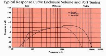
Frequency response of the 2118H/J in a closed box of 14 L ( $0.5 \text{ ft}^3$ ) internal volume. Measured response of a typical production unit, including all peaks and dips, does not deviate more than 2 dB from the above curve. The dashed curve represents the response with a 30 cm<sup>2</sup> (5 in<sup>2</sup>) port, 8 cm (3 in) long, tuning the enclosure to 70 Hz.
