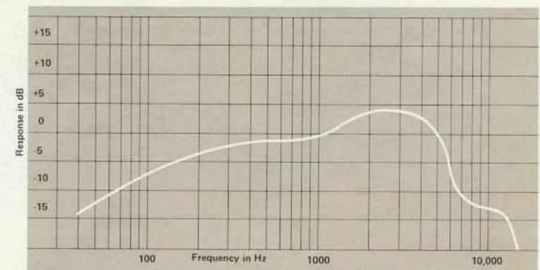
Frequency response contour of the 2130 in a closed box of six cubic feet internal volume. Measured response of a typical production unit, including all peaks and dips, does not deviate more than 2dB from the above curve. Additional acoustic loading (a port) will further extend bass response.
