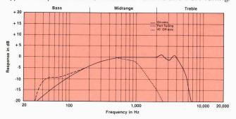
Frequency response of the 2202H in a closed box of 57 L (2 ft³) internal volume. Measured response of a typical production unit, including all peaks and dips, does not deviate more than 2 dB from the above curve. The dashed curve represents the response with an 80 cm² (12.5 in²) port, 18 cm (7 in) long tuning the enclosure to 40 Hz.
