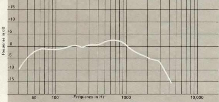
Frequency response contour of the 2205 in a closed box of six cubic feet internal volume. Measured response of a typical production unit, including all peaks and dips, does not deviate more than 2 dB from the above curve. Additional acoustic loading (passive radiator or port) will further extend bass response.
