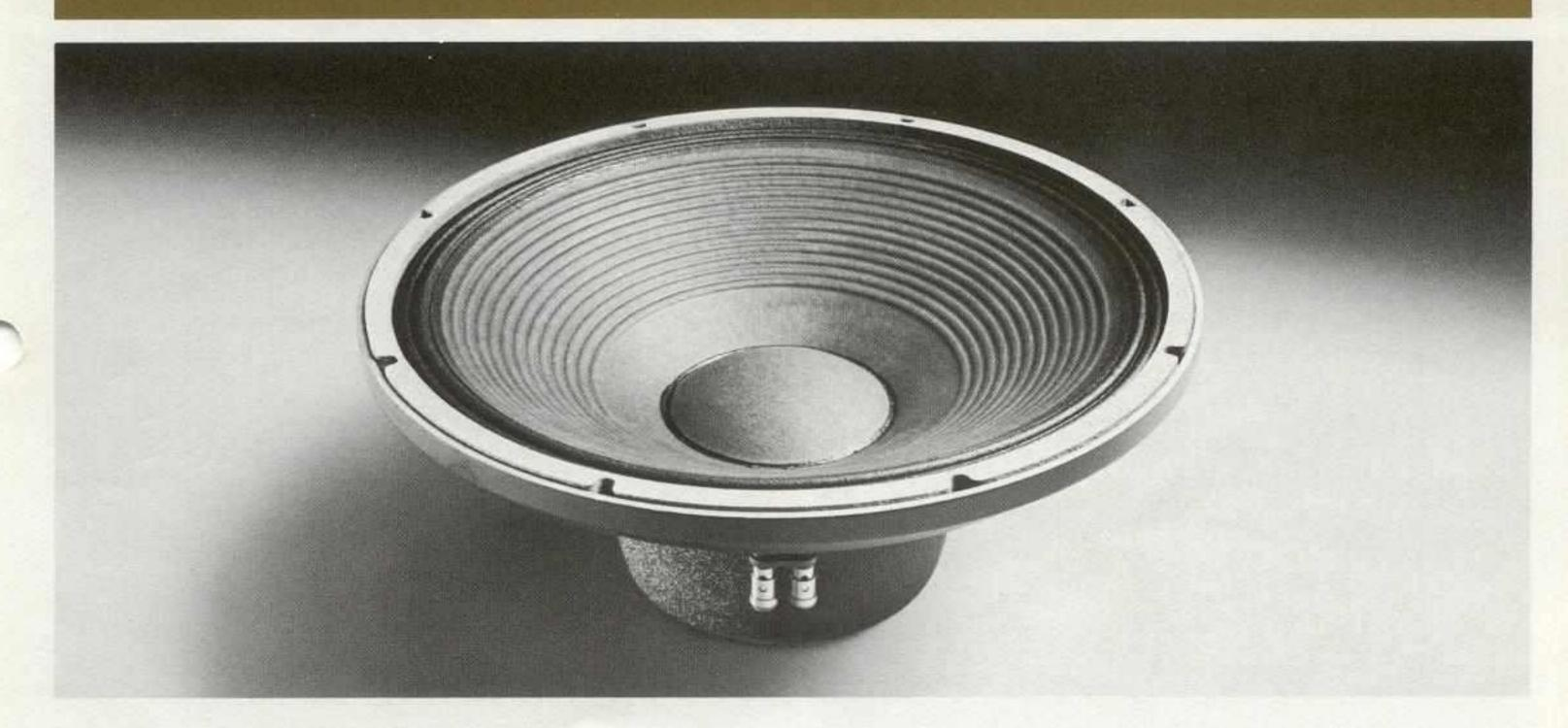
Model 2205 is a professional quality low frequency transducer capable of handling great amounts of power with ease. Sensitivity through the midrange is carefully controlled to provide highest possible efficiency without sacrificing bass performance. Because of this design approach, loading of the 2205 is not critical. It performs well in infinite baffles, ported enclosures, or as a horn driver. It is offered in 8, 16 and 32 ohm impedances for maximum versatility in multiple-transducer arrays.
