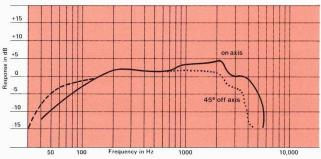
Frequency response contour of the 2220H/J taken in a hemispherical free-field environment, a closed box of 140 L (5 ft³) internal volume enclosing the rear of the driver. Measured response of a typical production unit, including all peaks and dips, does not deviate more than 2 dB from the above curve. The dashed curve represents the response from a  $160\ cm^2\,(25\ in^2)$  port with a 13 cm (5 in) long duct tuning this enclosure to 40 Hz.
