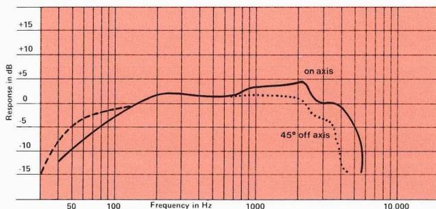
Frequency response contour of the 2220H/J taken in a hemispherical free-field environment, a closed box of 140 L (5 ft<sup>3</sup>) internal volume enclosing the rear of the driver. Measured response of a typical production unit, including all peaks and dips, does not deviate more than 2 dB from the above curve. The dashed curve represents the response from a 160 cm<sup>2</sup> (25 in<sup>2</sup>) port with a 13 cm (5 in) long duct tuning this enclosure to 40 Hz.
