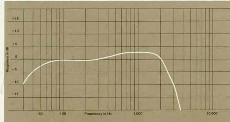
Frequency response contour of the 2231 in a closed box of 5 cubic feet (140 litres) internal volume. Measured response of a typical production unit, including all peaks and dips, does not deviate more than 2 dB from the above curve. Additional acoustic loading (passive radiator or port) will further extend bass response.
