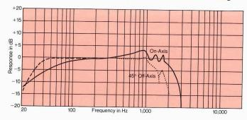
Frequency response contour of the 2235H taken in a hemispherical free-field environment, a closed box of 140 L (5 ft³) internal volume enclosing the rear of the driver. Measured response of a typical production unit, including all peaks and dips, does not deviate more than 2 dB from the above curve. The dashed curve represents the response from a 160 cm² (25 in²) port with a 28 cm (11 in) long duct tuning this enclosure to 30 Hz.
