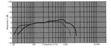
Frequency response contour of the 2240H/G taken in a hemispherical free-field environment, a closed box of 280 I (10 ft<sup>3</sup>) internal volume enclosing the rear of the driver. Measured response of a typical production unit, including all peaks and dips, does not deviate more than 2 dB from the above curve. The dashed curve represents the response from a 320 cm<sup>2</sup> (50 in<sup>2</sup>) port with a 20 cm (8 in) long duct tuning this enclosure to 30 Hz.
