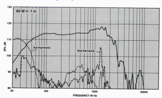
Distortion levels raised 20 dB, measured at 60 watts, 1 meter.
