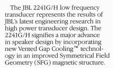
To increase power handling while reducing power compression, JBL engineers have created a unique, direct voice-coil-to-air heat dissipation method called Vented Gap Cooling (patent pending). This process pumps air through the magnetic gap and directly over and around the voice coil to provide immediate heat transfer and reduction in operating temperature — a direct improvement in power compression.
