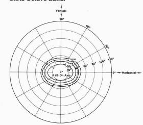
2 kHz octave bandwidth constant sound pressure contours. Same conditions as 500 Hz contours. This data may be considered essentially the same as would be observed at 4 kHz and 8 kHz, considering only the -3, -6, and -9 dB isobars.
