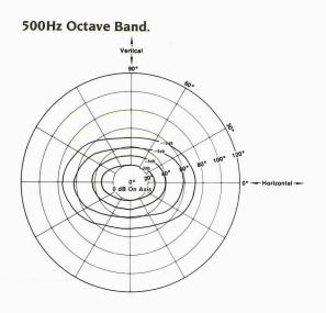
500 Hz octave bandwidth constant sound pressure contours of 0 to -12 dB in steps of -3 dB. The contours are plotted on polar grid lines with on axis being the center of the plot. The data was gathered by taking an octave polar plot at all oblique angles from 0° (horizontal) to 90° (vertical) in steps of 5°.
