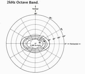
2 kHz octave bandwith constant sound pressure contours. Same conditions as 500 Hz contours. This data may be considered essentially the same as would be observed at 4 kHz and 8 kHz, considering only the -3, -6, and -9 dB insobars.
