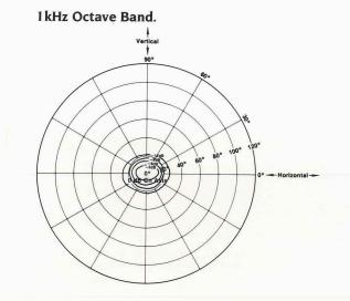
I kHz octave bandwidth constant sound pressure contours. Same conditions as 500 Hz contours.
