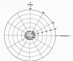
2 kHz octave bandwidth constant sound pressure contours. Same conditions as 500 Hz contours. This data may be considered essentially the same as would be observed at 4 kHz and 8 kHz, considering only the -3, -6, and -9 dB isobars.
