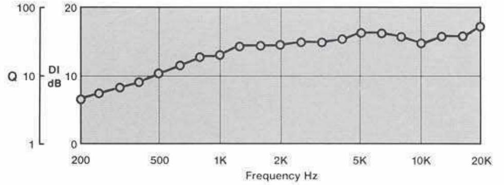
Horizontal Off-axis Response (Normalized to on-axis)
