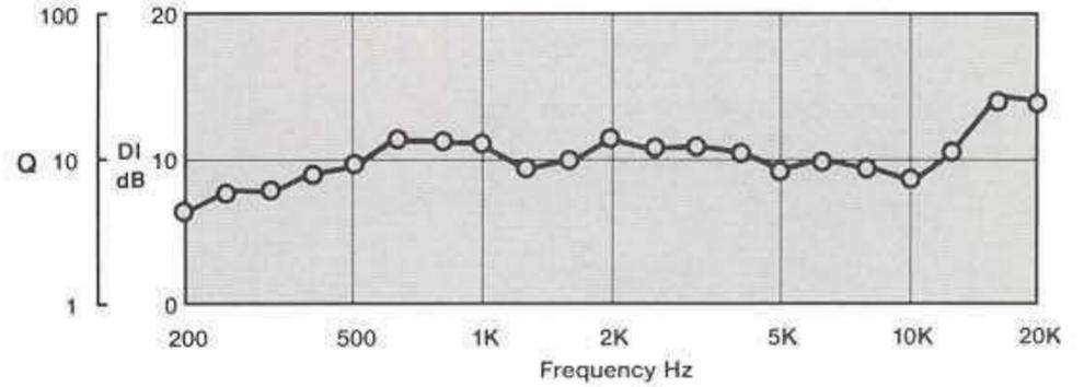
Horizontal Off-axis Response (Normalized to on-axis)
