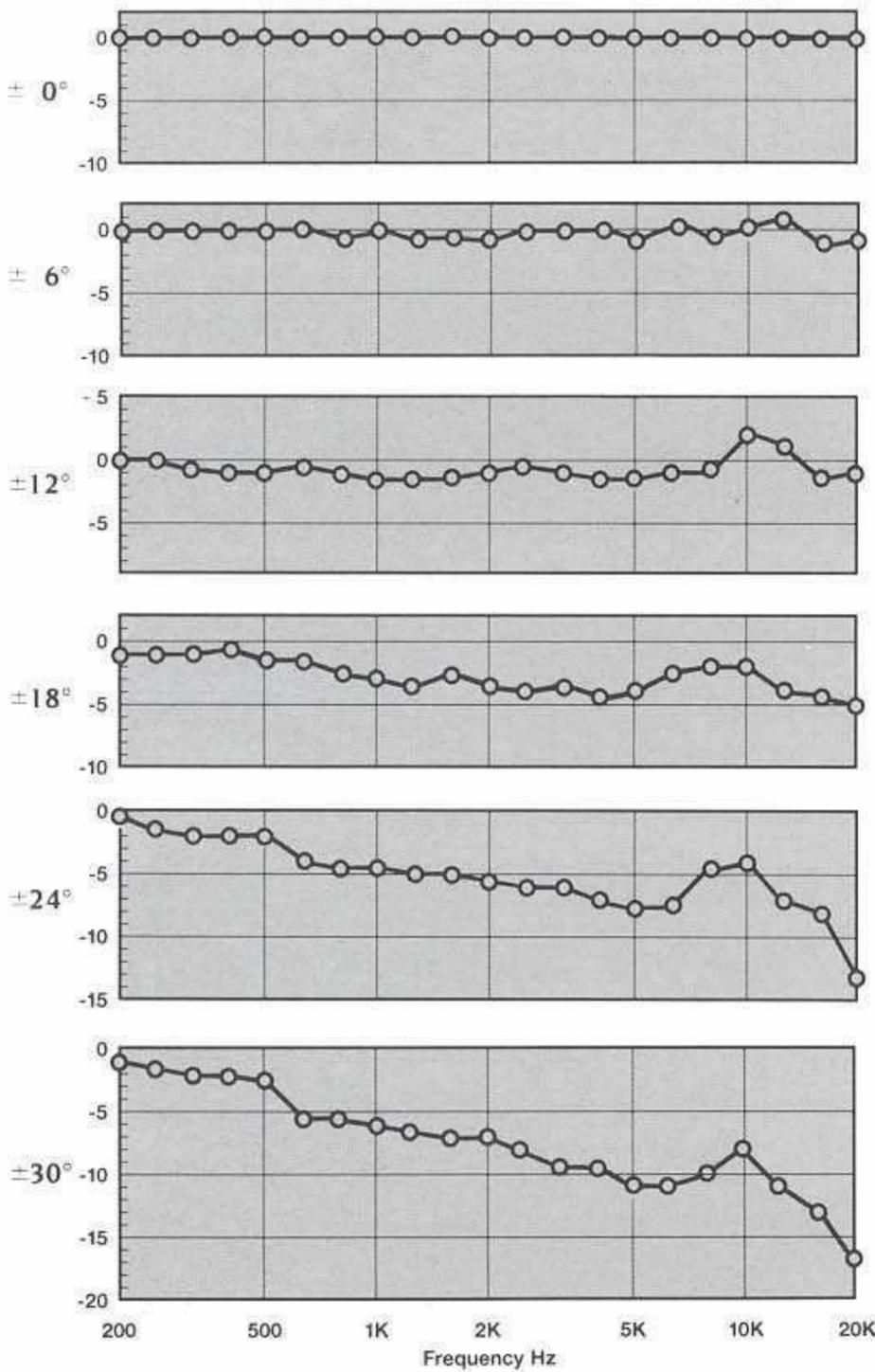
Vertical Off-axis Response (Normalized to on-axis)
