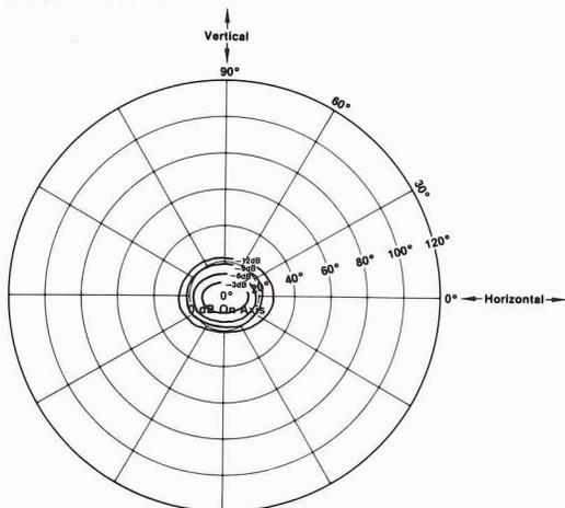
2 kHz octave bandwidth constant sound pressure contours. Same conditions as 500 Hz contours. This data may be considered essentially the same as would be observed at 4 kHz and 8 kHz, considering only the -3, -6, and -9 dB isobars.
