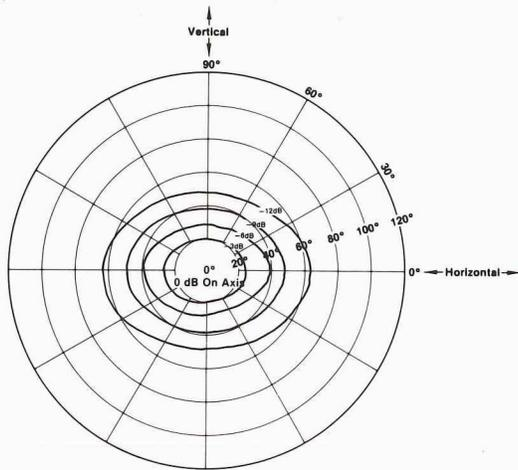
500 Hz octave bandwidth constant sound pressure contours of 0 to -12 dB in steps of -3 dB. The contours are plotted on polar grid lines with 0 dB axis being the center of the plot. The data was gathered by taking an octave polar plot at all oblique angles from 0° (horizontal) to 90° (vertical) in steps of 5°.
