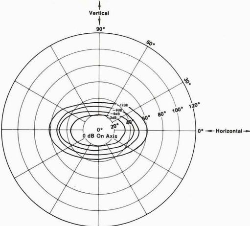
2 kHz octave bandwidth constant sound pressure contours. Same conditions as 500 Hz contours. This data may be considered essentially the same as would be observed at 4 kHz and 8 kHz, considering only the -3, -6, and -9 dB insobars.
