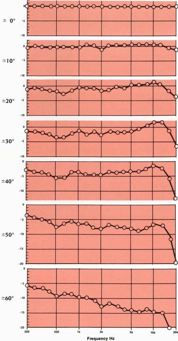
Vertical Off-axis Response (Normalized to on-axis)
