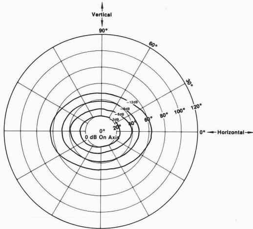
500 Hz octave bandwidth constant sound pressure contours of 0 to -12 dB in steps of -3 dB. The contours are plotted on polar grid lines with 0 axis being the center of the plot. The data was gathered by taking an octave polar plot at all oblique angles from 0° (horizontal) to 90° (vertical) in steps of 5°.
