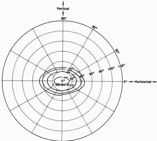
500 Hz octave bandwidth constant sound pressure contours of 0 to -12 dB in steps of -3 dB. The contours are plotted on polar grid lines with on axis being the center of the plot. The data was gathered by taking an octave polar plot at all oblique angles from 0° (horizontal) to 90° (vertical) in steps of 5°.
