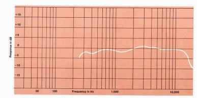
Frequency response contour of Model 2421 coupled to a 2350 horn. Measured response of a typical production unit, including all peaks and dips, does not deviate more than 2 dB from the above curve.
