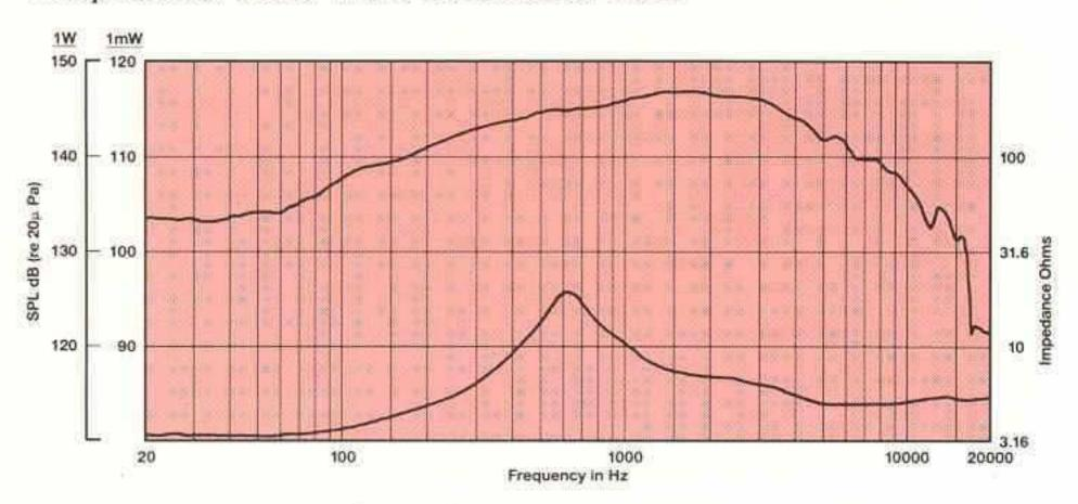
Frequency response and impedance modules of Model 2427H/J coupled to a 25 mm (I in) diameter terminated plane-wave tube. This is the power response of the transducer, and is the frequency response that will be obtained on a true full-bandwidth constant-directivity horn design, such as JBL's 2360 series of Constant Coverage Bi-Radial Horns.
