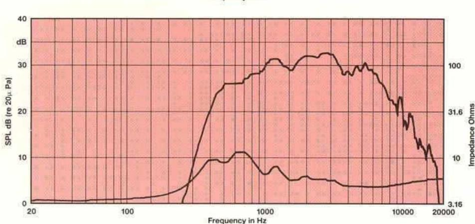
Frequency response of the 2427H/J coupled to the 2380A (top graph) and 2385A (bottom graph) Flat-Front Bi-Radial horns, measured on-axis at a distance of I meter with a 1-watt (2.83 V RMS) input in a reflection-free environment, with impedance vs. frequency curve. The increased high-frequency output is due to the horn design's increasing directivity in the vertical plane.
