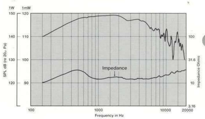
Frequency response and impedance modulus of Model 2450J coupled to a 49 mm (2 in) diameter terminated plane-wave tube, with sensitivity referenced to a 25 mm (1 in) tube. This is the power response of the transducer, and is the frequency response that will be obtained on a true full-range constant directivity horn design, such as JBL's 2360 series of Constant Coverage Bi-Radial® Horns.
