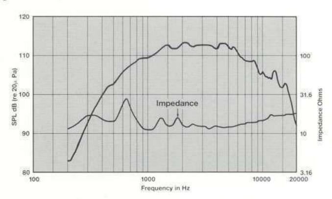
Frequency response of the 2450J coupled to a JBL 2380A Flat-Front Bi-Radial® Horn, measured on-axis at a distance of 1 meter with a 1-watt (4.0 V RMS) input in a reflection-free environment, with impedance vs. frequency curve. A horn with a pure exponential flare, such as typical radial horn designs, will exhibit greater high frequency output onaxis at the expense of lost annular coverage.
