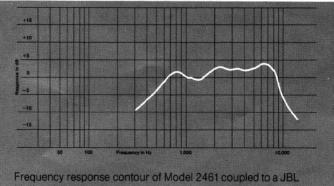
Model 2350 horn. Measured on-axis response of a typical production driver on this horn, including all peaks and dips, does not deviate more than 2 dB from the above curve.
