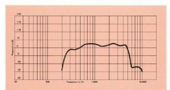
Frequency response contour of Model 2482 coupled to a 2366 horn. Measured response of a typical production unit, including all peaks and dips, does not deviate more than 2 dB from the above curve.
