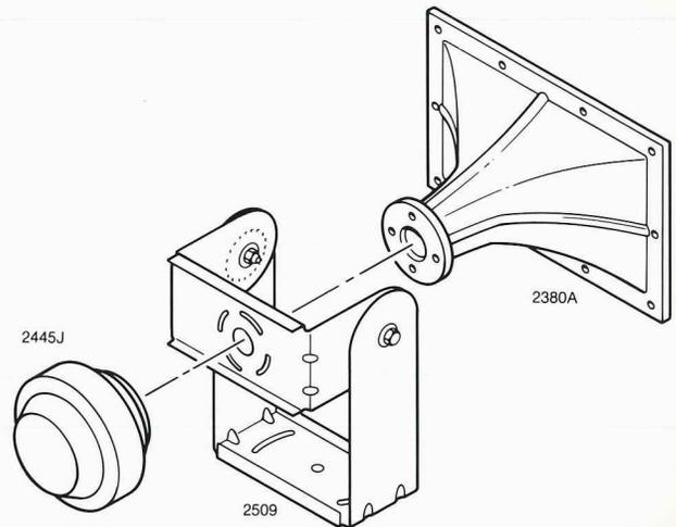
INSTALLATION ORIENTATION FOR WALL OR CLUSTER MOUNTING
