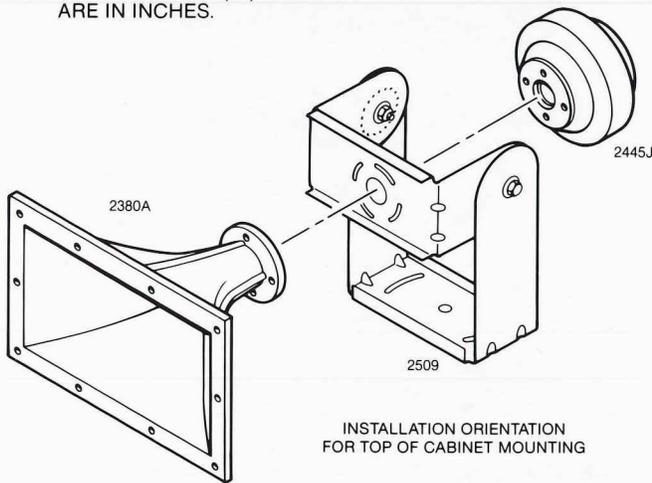
INSTALLATION ORIENTATION FOR TOP OF CABINET MOUNTING
