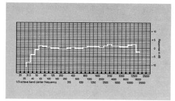
Frequency response of the 4301BE taken with ½-octave band pink noise. Measured response of a typical production system averaged through an inclusive arc of 30° vertically and horizontally does not deviate more than 3 dB from the above curve.
