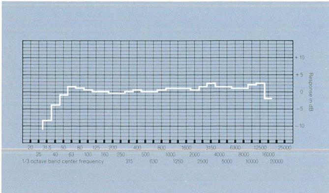
Frequency response of the 4301E taken with  $\frac{1}{3}$ -octave band pink noise. Measured response of a typical production system averaged through an inclusive arc of  $30^\circ$  vertically and horizontally does not deviate more than 3 dB from the above curve.
