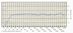
Frequency response of the 4313B taken with ½-octave band pink noise. Measured response contour of a typical system averaged through an inclusive arc of 120° in the horizontal plane does not deviate more than 3 dB from the above curve.
