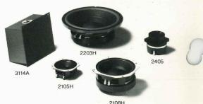
assembly. Its 44 mm (1% in) edgewound aluminum ribbon voice coil is suspended within a field having a flux density of 1.65 T (16,500 gauss), and it is affixed to a heat-resistant support bonded to a ring diaphragm pneumatically formed of 0.05 mm (0.0022 in) aluminum stock. The integral diffraction horn produces a wide high-frequency dispersion pattern.
