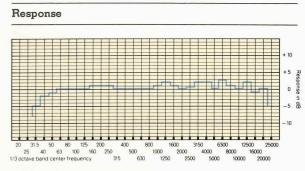
Frequency response of the 4315B taken with ½-octave band pink noise. Measured response contour of a typical system averaged through an inclusive arc of  $80^\circ$  in the horizontal and  $60^\circ$  in the vertical planes does not deviate more than 2 dB from the above curve.
