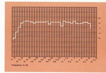
Frequency response of the 4345 taken with 1/3-octave band pink noise. Measured response contour of a typical system averaged through an inclusive arc of 60° in the horizontal and 30° in the vertical planes does not deviate more than 2 dB from the above curve.
