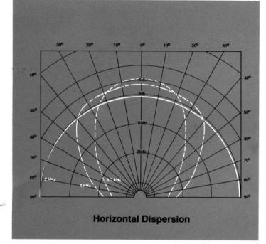
Above curves taken in hemispherical free-field conditions with the microphone at 7 m (24 ft) from the system.
